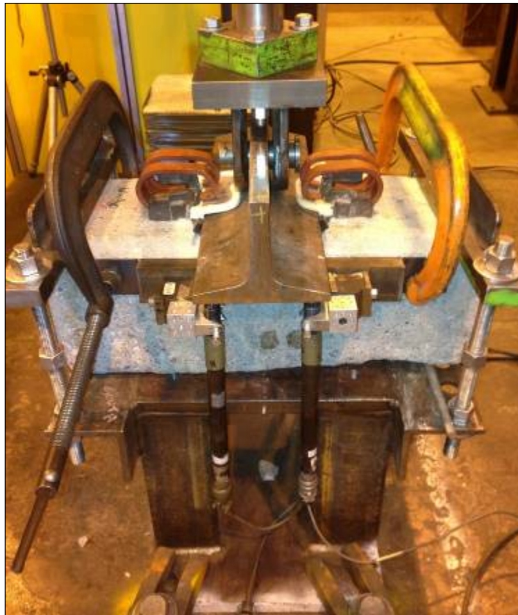
Figure 18. Vertical Rail Uplift Fixture
