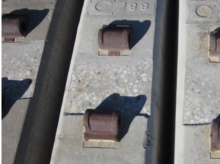
Figure 4. Detailed View of Ground Rail Seat with 0.1875-inch triangular RSD before installation at FAST
