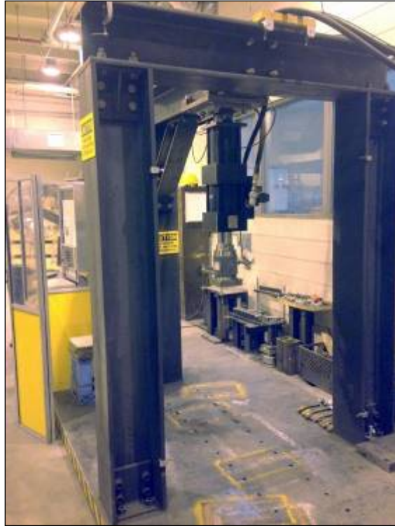
Figure 14. Three-Post Load Frame
