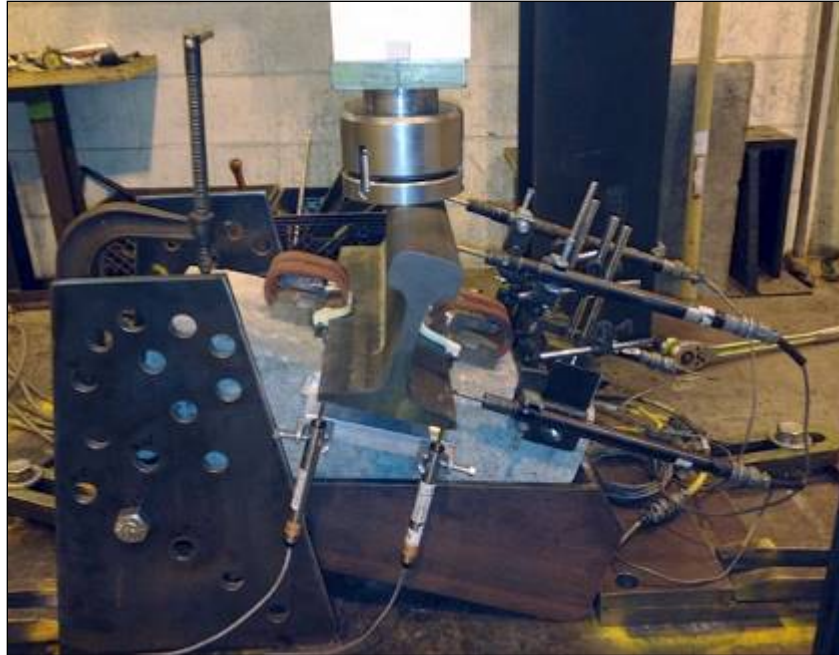
Figure 23. Lateral/Vertical Compliance Fixture
