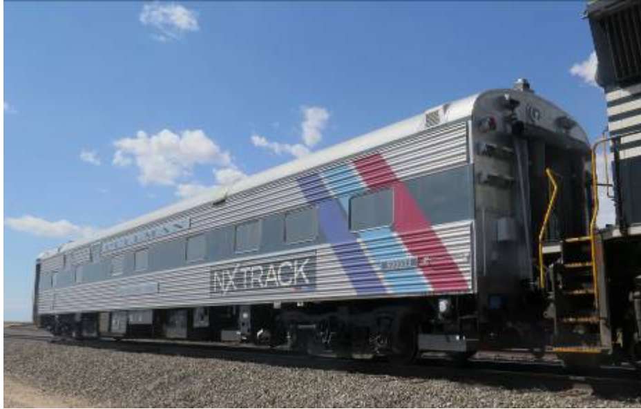
Figure 44. NxGen and NxTrack Track Geometry and Machine Vision Vehicle
