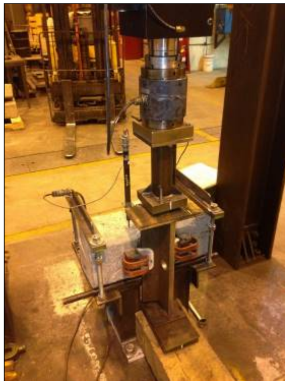
Figure 16. Rail Longitudinal Restraint Fixture
