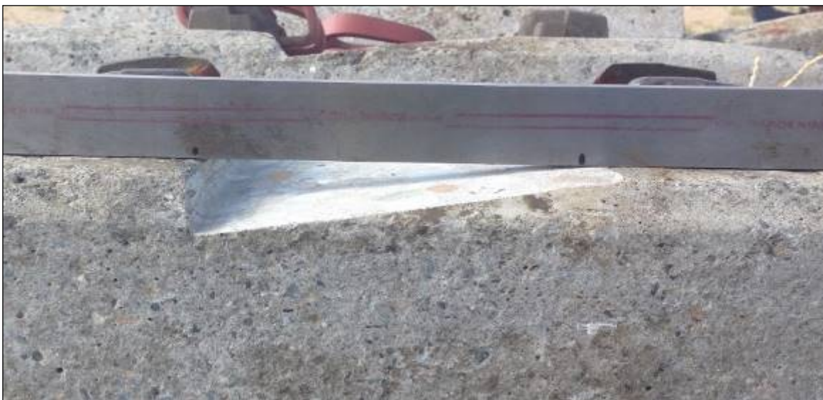
Figure 12. Example Showing Triangular RSD Depth Profile
