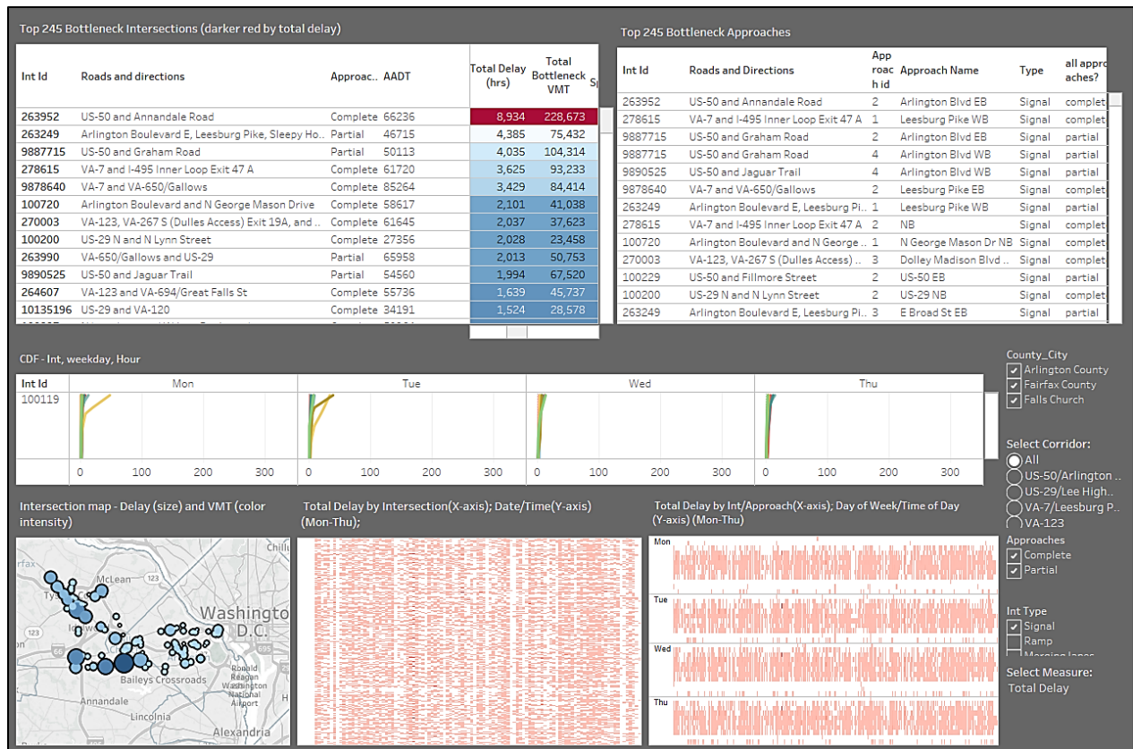
Figure 9. Dashboard of Visualization Tool. The dashboard includes Intersection Bottleneck Rank Table (top left), Approach Bottleneck Rank Table (top right), Cumulative Distribution Functions (CDFs) (center), Map view (bottom left), Intersection Delay Heatmap (bottom center), and Approach Delay Heatmap (bottom right).
