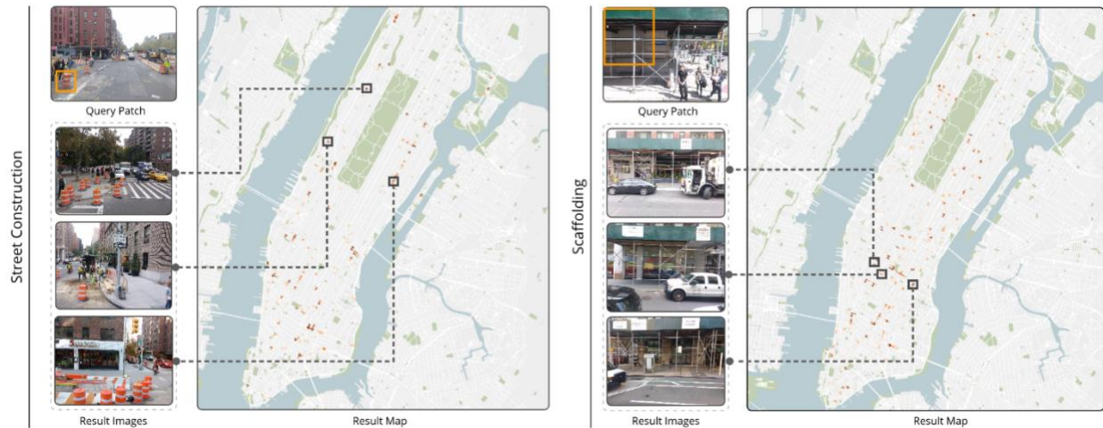
Figure 18: Using Urban Portfolio to assess construction zone safety compliance. The left image shows results from a query for images containing traffic drums that are common to street renovation. The right image shows results from querying for scaffolds, commonly installed during building renovations in NYC.
