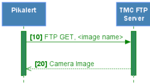
Figure 5-44. Sequence Diagram: Pikalert Retrieves Camera Images for RWIS Stations from TMC FTP Server.
