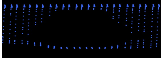
Figure 5.16 Culvert in LiDAR Data
