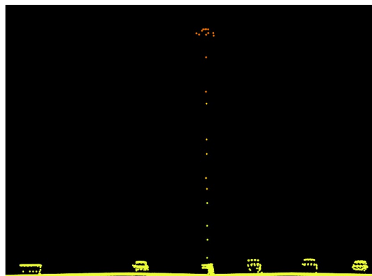
Figure 5.10 Light Pole in LiDAR Data
