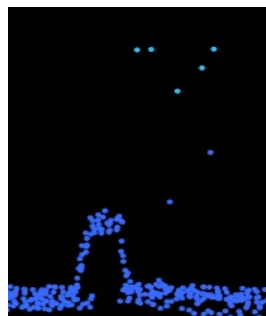
Figure 5.6 Small Traffic Signal in LiDAR Data
