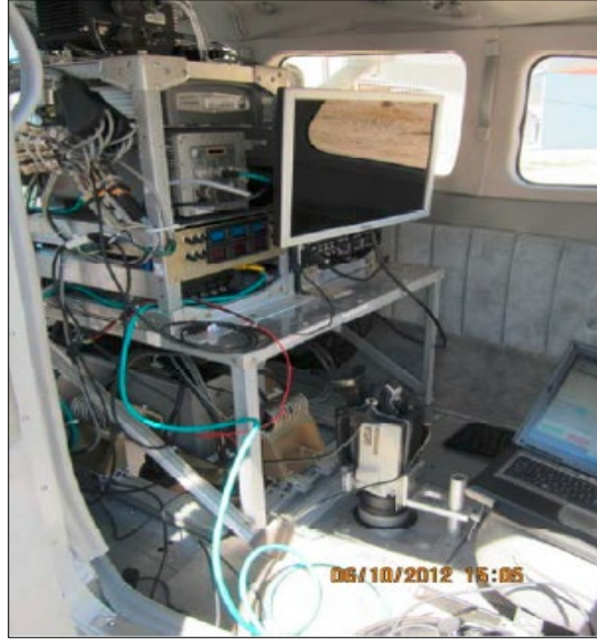
Figure 4.2 The Onboard Integrated Remote Sensing System
