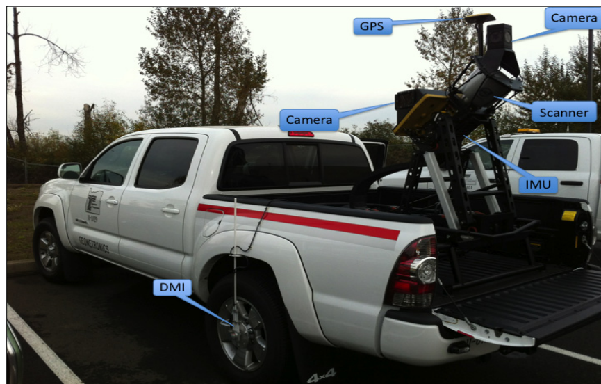
Figure 3.3 Mobile LiDAR System (Topcon IP-S2 HD system operated by Oregon DOT)
