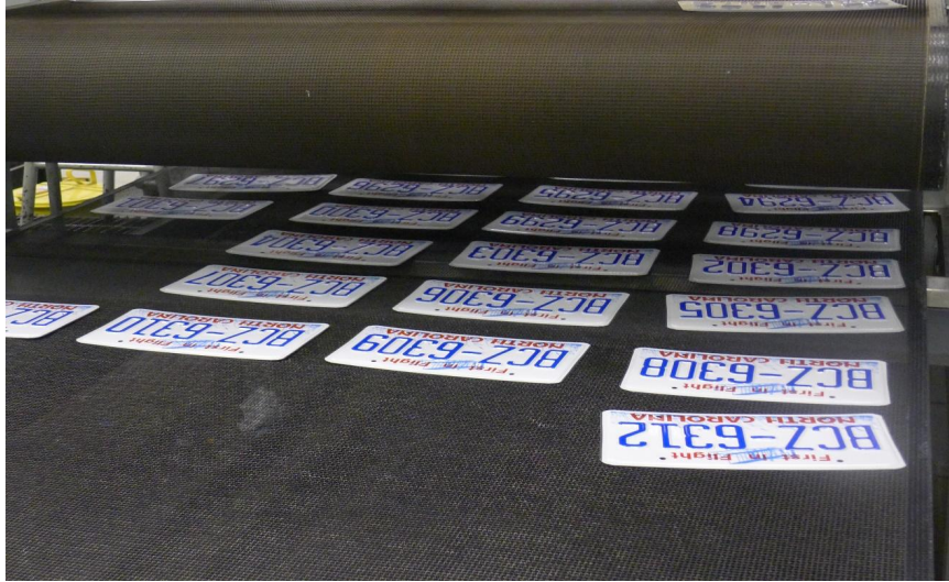
Figure 9. Painted license plates passing through the oven for drying.
