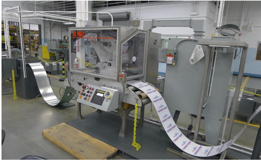
Figure 5. Image of the aluminum straightening and reflective sheeting application process.
