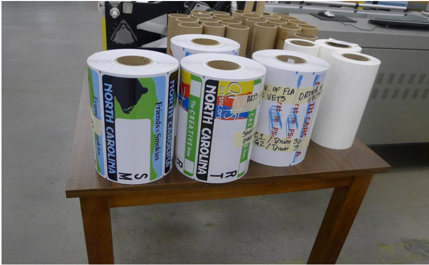
Figure 14. Rolls of graphically designed and digitally printed specialty license plate sheeting.
