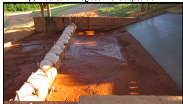
(h) Curlex Bloc sediment deposition
