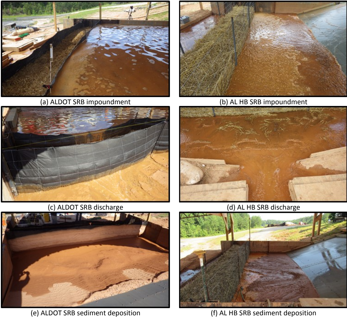
Figure 43. SRB performance observations.
