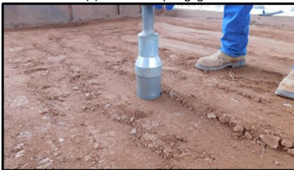
(e) obtaining density sample
