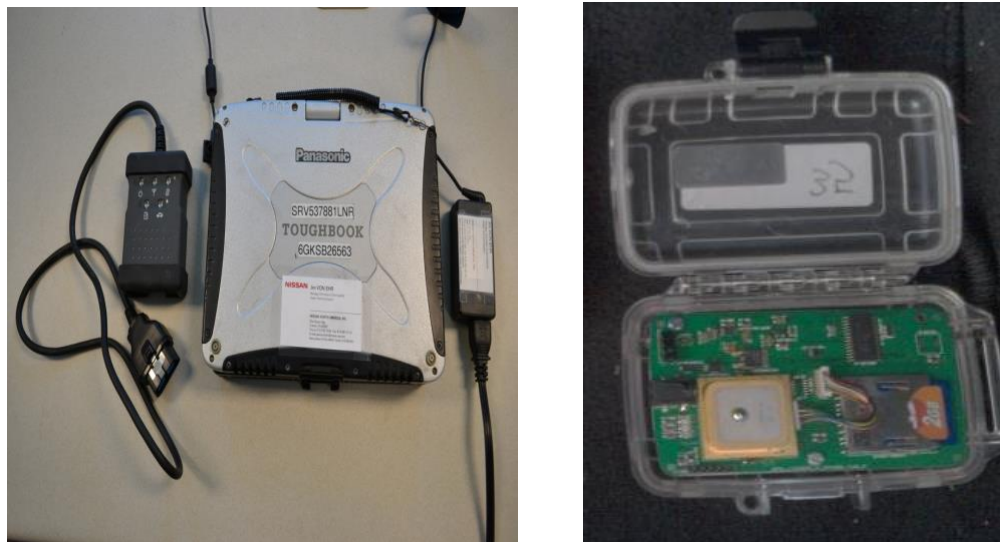
Figure 1. Data collection equipment: (left) CONSULT III plus kit to collect test vehicle’s energy consumption and other vehicle activities data; (right) GPS data logger.
