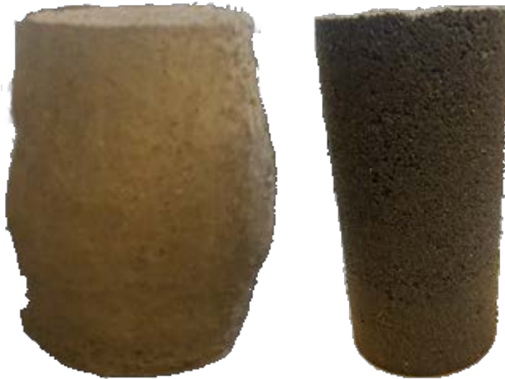
Figure 19 Specimen after (left) and before (right) shearing
