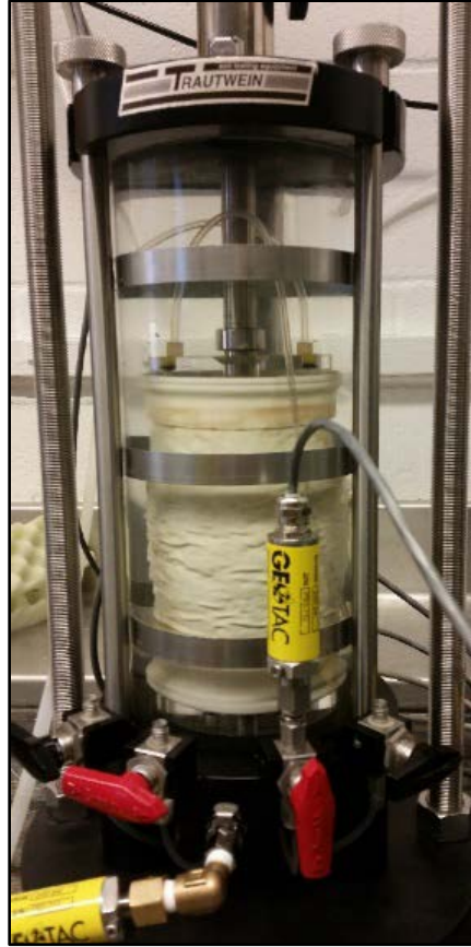
Figure 18 Failed specimen in loading frame
