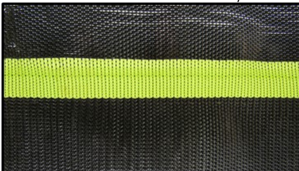
(e) woven monofilament – green stripe narrow filament – variable density
