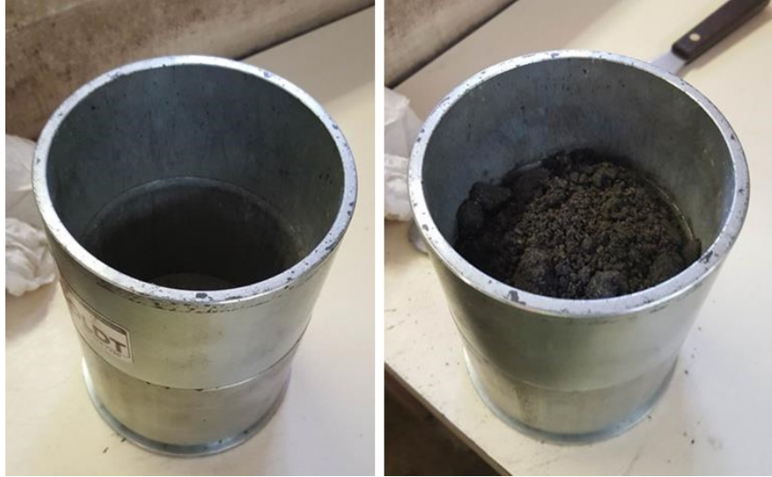
Figure 4. Preparing Mold for Marshall Compaction: (Left) mold for Marshall specimen; (Right) filled mold for Marshall specimen
