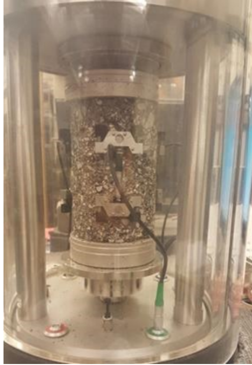
Figure 12. Dynamic Modulus Test Specimen in Asphalt Mixture Performance Tester
