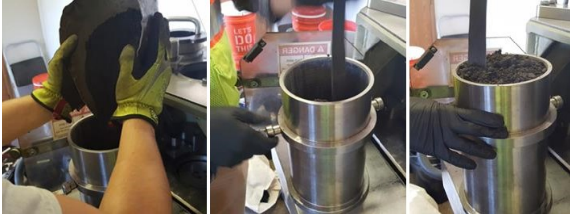
Figure 6. Preparing Mold for Dynamic Modulus Specimens: (Left) placing CCPR mixture into mold; (Middle) rodding mixture after filling bottom half; (Right) rodding mixture after filling top half. CCPR = cold central plant recycling.
