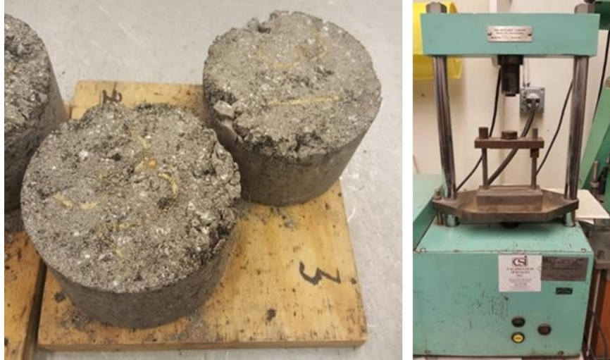
Figure 9. ITS Testing: (Left) ITS specimen; (Right) ITS apparatus. ITS = indirect tensile strength.
