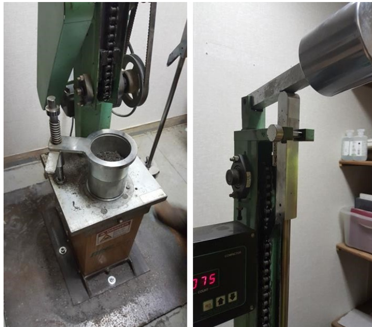
Figure 5. Setting Mold Into Marshall Hammer: (Left) loading mold into apparatus; (Right) setting up Marshall hammer.
