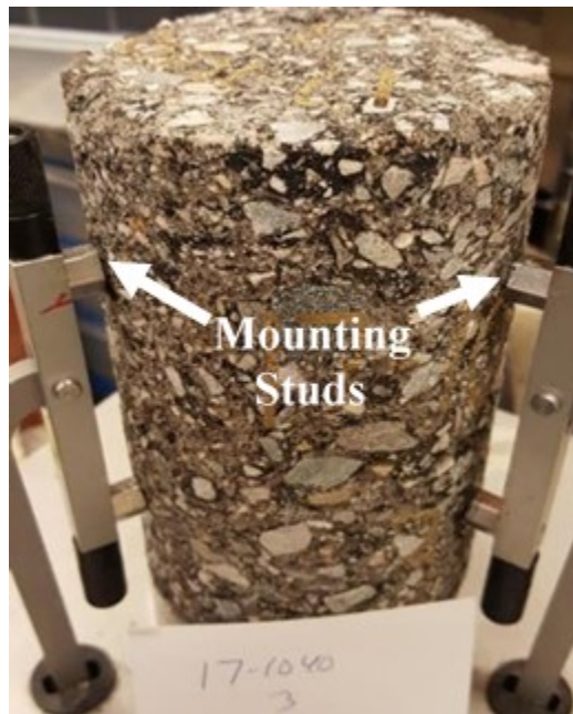
Figure 11. Mounting Studs Affixed to Dynamic Modulus Test Specimen
