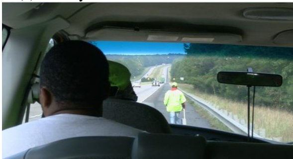
(c) Visual survey and record distresses
