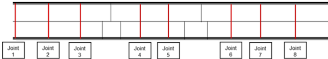
Figure 2.9 Faulting reading taken at 8 th original joint
