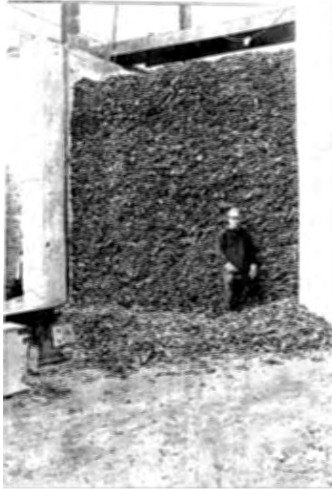
Figure 6.24 Vertical wall of tire chips after completion of test with Pine State Recycling
