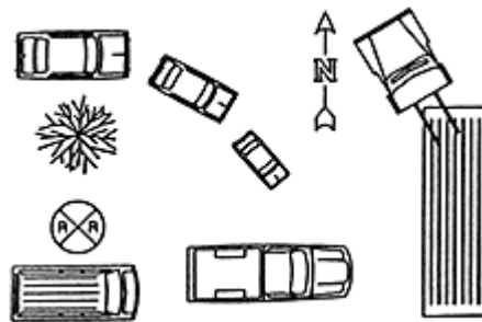
Figure 2: Examples of shapes or symbols included with EDCAD. Each shape may be enlarged, reduced or rotated to any angle.
