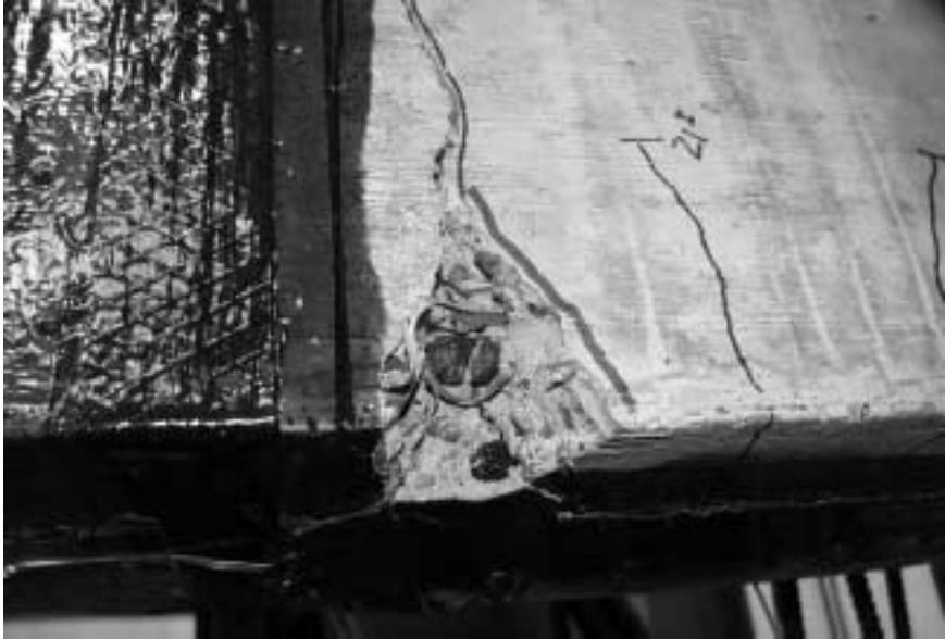
Figure 8.8 Detail Showing Fatigue Fracture of Reinforcing Bar in Specimen A-F4
