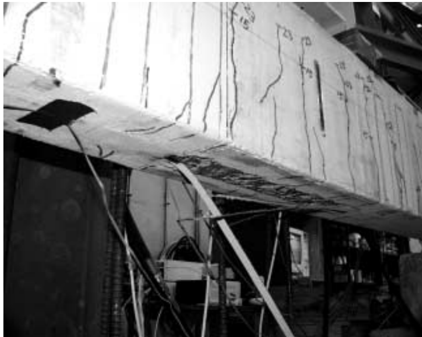
Figure 6.20 Bottom View of Specimen A-LT2 after Rupture of the CFRP Composite
