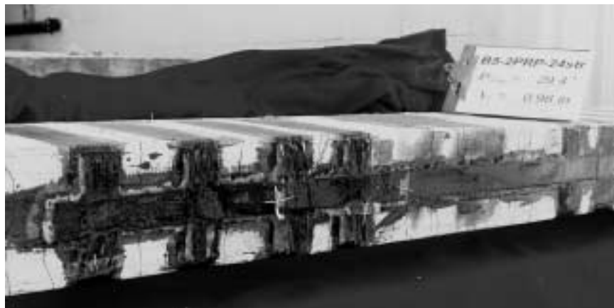
Figure 6.11 Bottom View of Specimen B5 after Debonding
