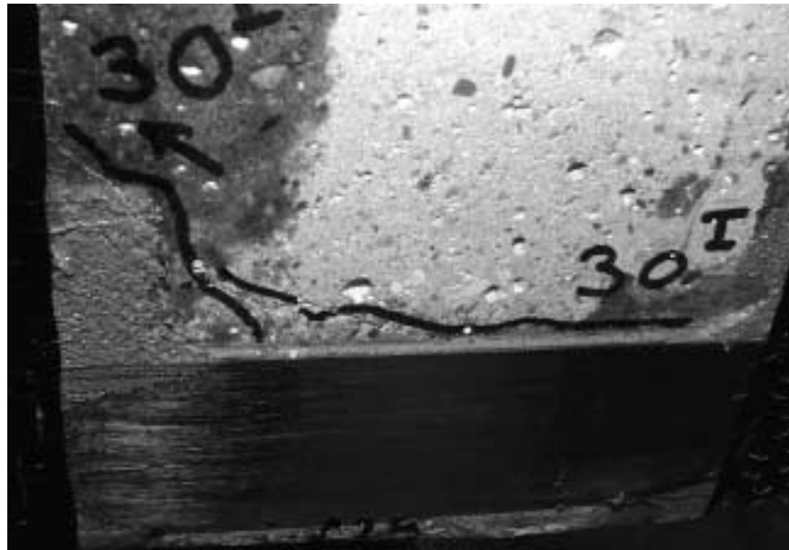
Figure 8.17 Detail Showing Propagation of Debonding Along the Top Edge of the Composite Laminate in Specimen D-F4 during the First Cycle of Loading
