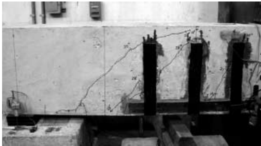
Figure 8.14 Shear Crack that Formed During Cycling of Specimen D-F3
