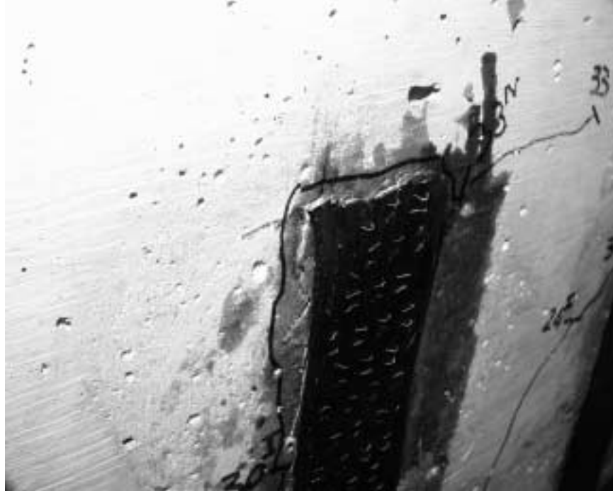
Figure 8.18 Debonding of Vertical Composite Straps During Cycling of Specimen D-F4
