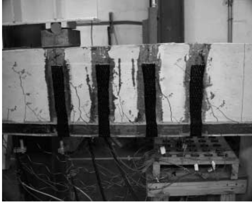
Figure 6.16 Formation of Debonding Cracks in Specimen D4
