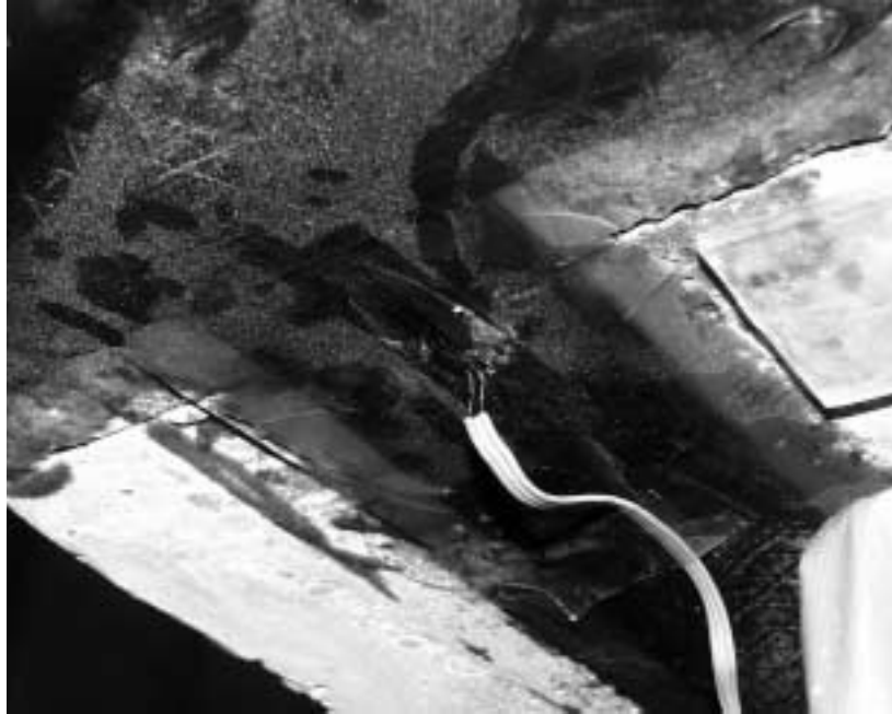
Figure 8.4 Local Debonding of CFRP Composite after 100,000 Cycles of Loading in Specimen A-F3
