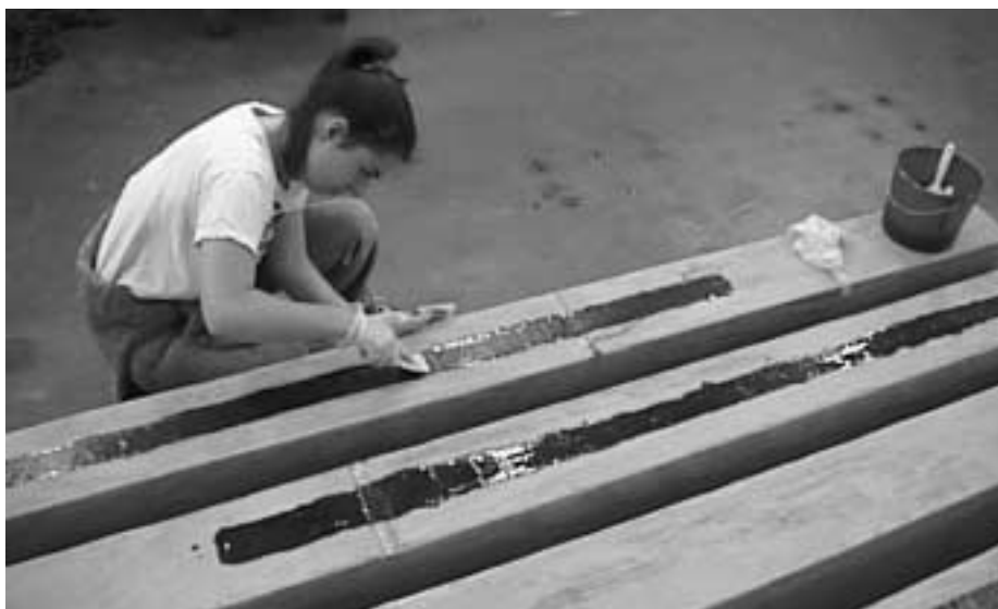
Figure 4.4 Composite Systems A and B: Unidirectional Carbon Fibers
