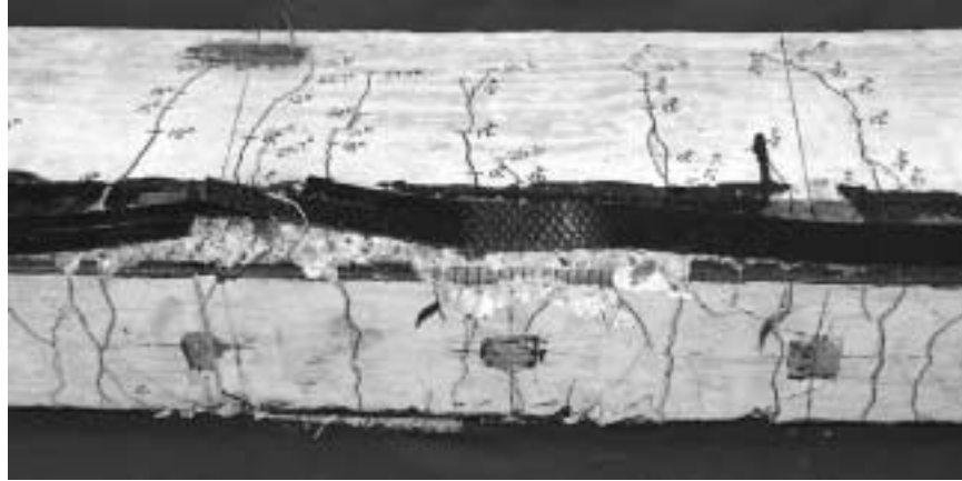
Figure 6.13 Rupture of CFRP Composite in Specimen B3 after Failure
