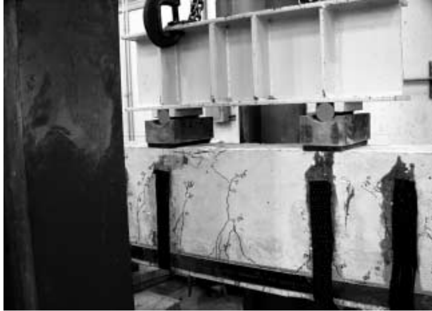
Figure 8.15 Crushing of the Concrete in the Compression Zone after Debonding of the CFRP Plate on the Opposite Side of Specimen D-F3
