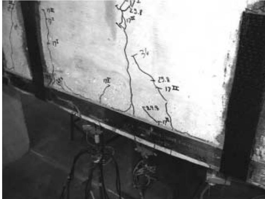
Figure 8.11 Formation of Debonding Cracks in Specimen D-F2
