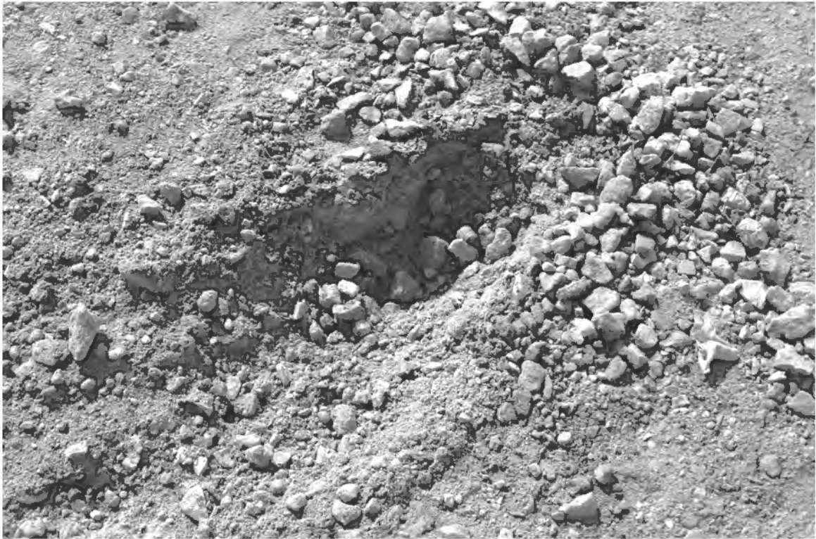
Figure 8. Support After Test 414587-1.
