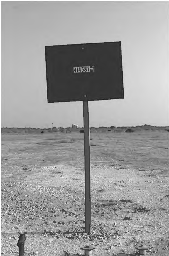
Figure 4. Recycled Plastic Sign Support Before Test 414587-1.
