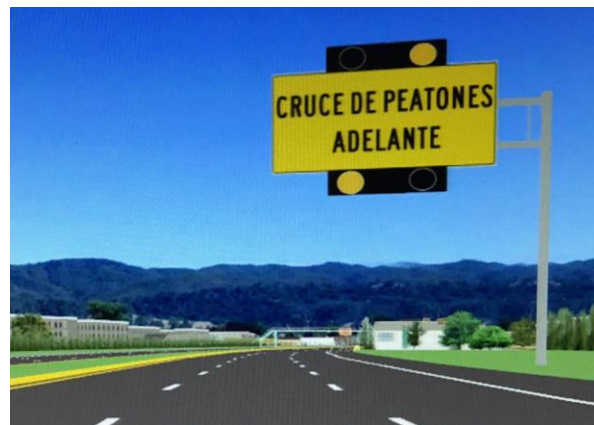
Figure 4.8 - Overhead pedestrian warning sign with flashing beacons and the legend "CRUCE DE PEATONES ADELANTE"
