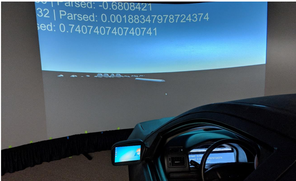
Figure 4.2 – Integration of Unity-based simulator and RTI vehicle cabin
