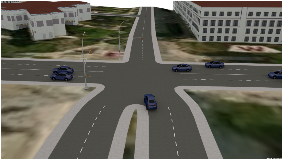
Figure 4.2: Side view of simulated intersection containing 30 connected autonomous vehicles. Each vehicle is simulated separately as a high-fidelity vehicle in Chrono but share the same virtual environment and scenario through the Synchrono multi-agent simulation framework.
