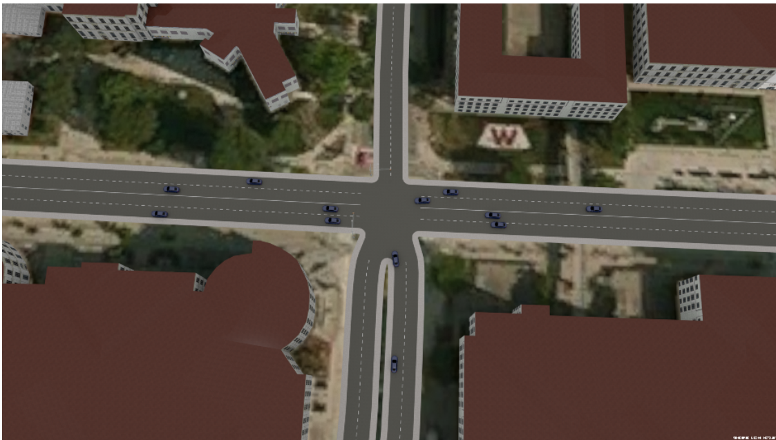
Figure 4.1: Top view of simulated intersection containing 30 connected autonomous vehicles. These vehicles use communication and simulated sensor data to safely navigate the congested roadway.
