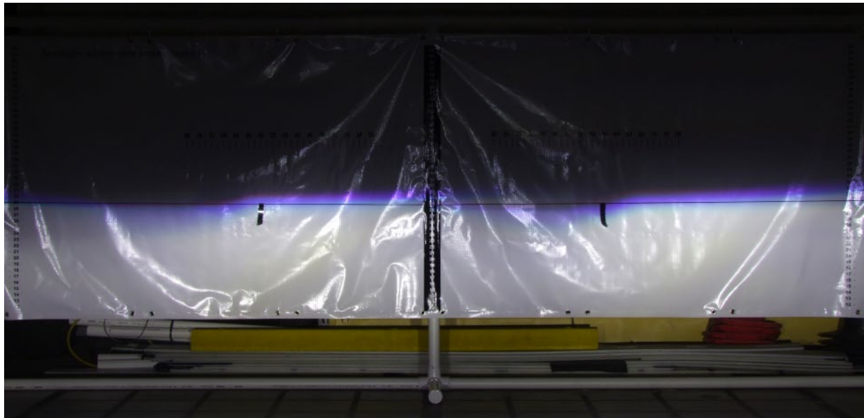
Figure 11. 2015 Lexus LS460L - Headlamp Projection Pattern (Aimed)
