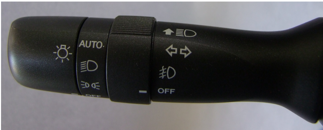
Figure 9. 2015 Lexus LS460L Sedan - Headlighting System Control
