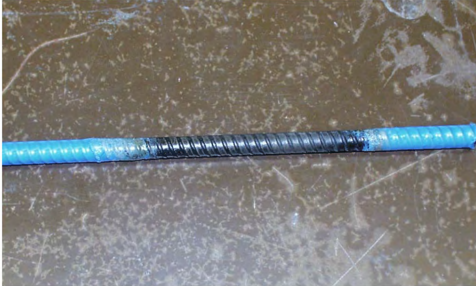
Figure 4.8: Nylon Coating Removed for Control Specimens
