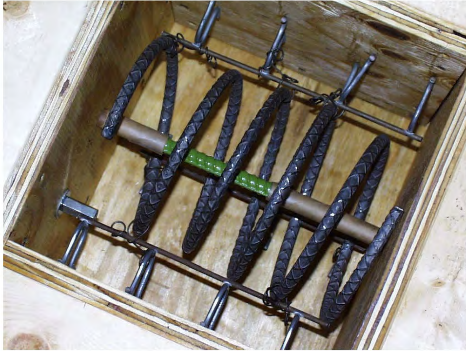
Figure 4.10: Typical Reinforcing Steel and Test Bar Setup
