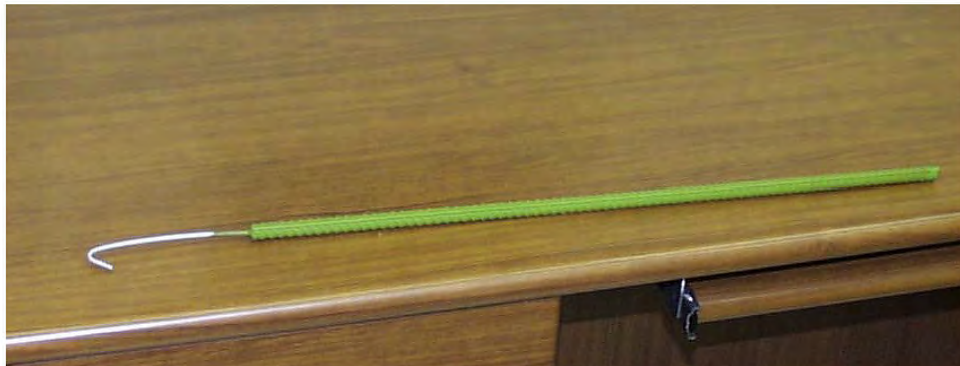
Figure 4.5: Typical PVC-Coated Bar
