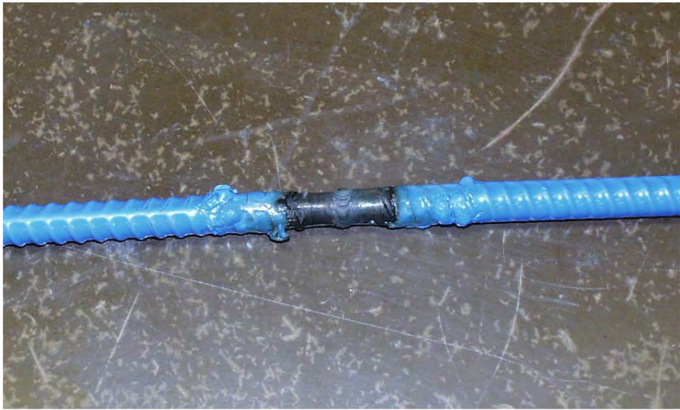
Figure 4.7: Typical Nylon-Coated Bar Weld
