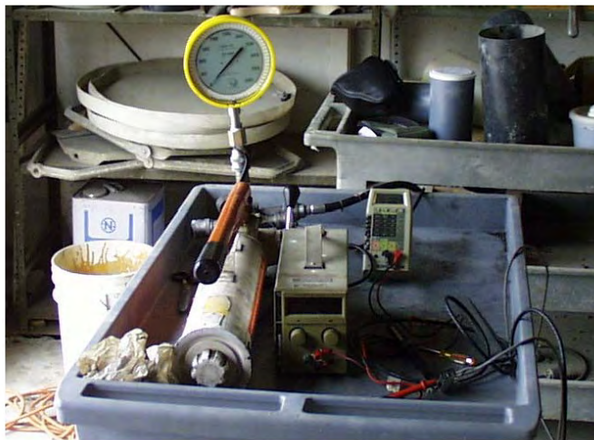
Figure 4.19: Hand Pump and Load Cell Output
