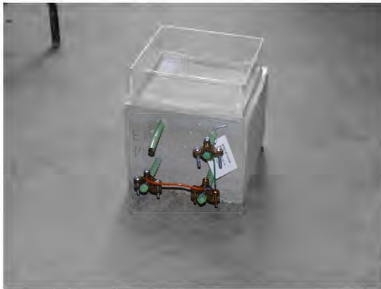
Figure 3.2: Completed Macrocell Specimen
