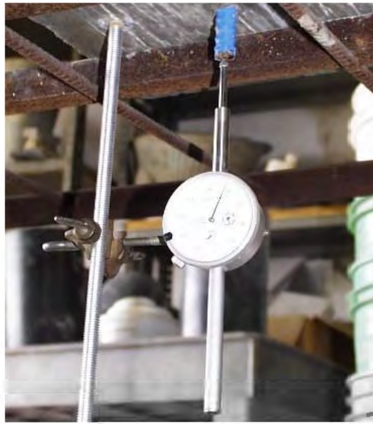
Figure 4.20: Slip Measured by Linear Displacement Gauge
