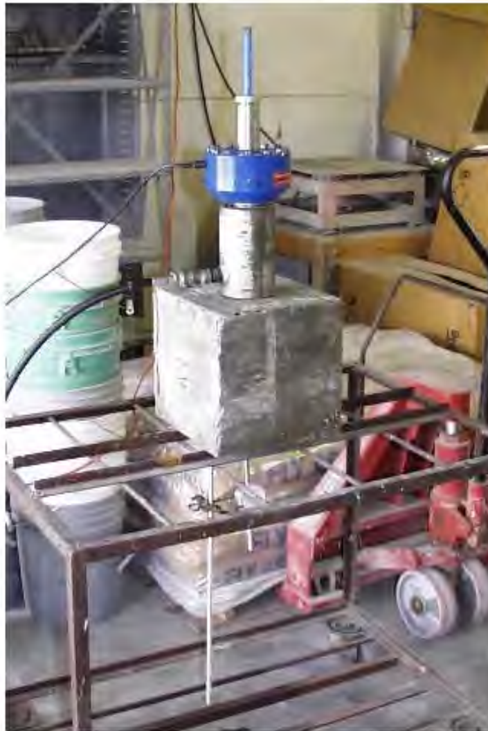
Figure 4.21: Complete Pullout Test Loading Setup
