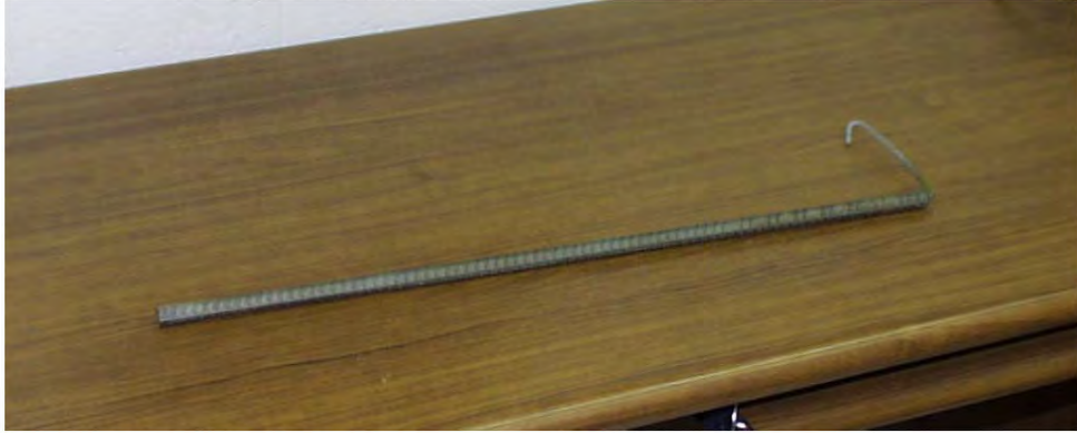
Figure 4.6: Typical Bar After Removal of PVC Coating
