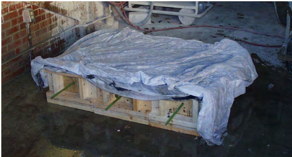
Figure 4.13: Curing of Pullout Specimens
