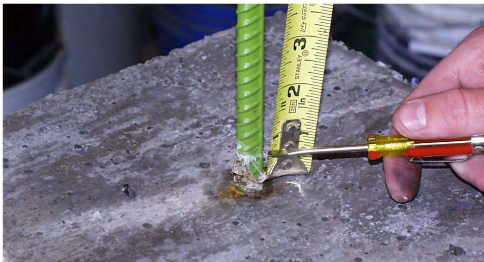
Figure 5.4: Typical PVC Pullout Failure
