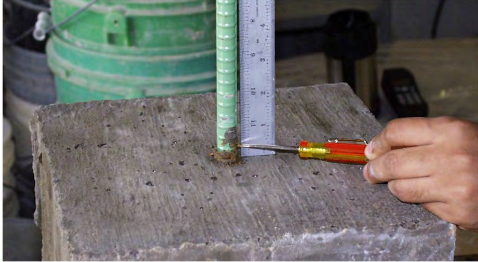
Figure 5.5: Typical Epoxy Pullout Failure
