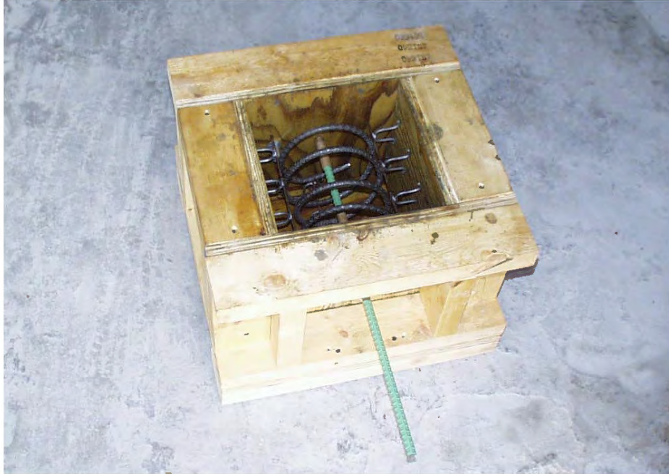
Figure 4.9: Typical Form for Pullout Specimens
