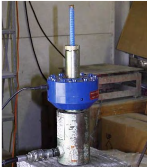
Figure 4.18: Hydraulic Ram, Load Cell, and Grips
