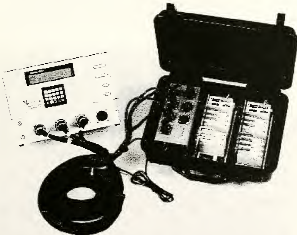
Figure 17 Controller Interface Device Connected to NEMA TS1 Compliant Controller [Bullock and Catarella, 1997]
