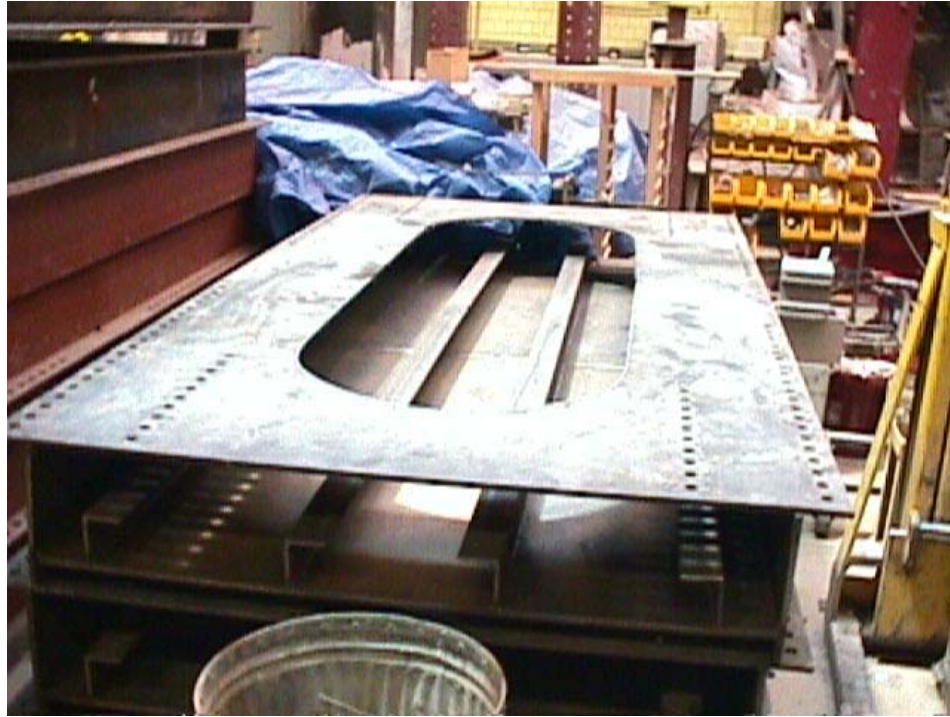
Figure 3-13: Case 4 with viewport cut into middle flange prior to testing.
