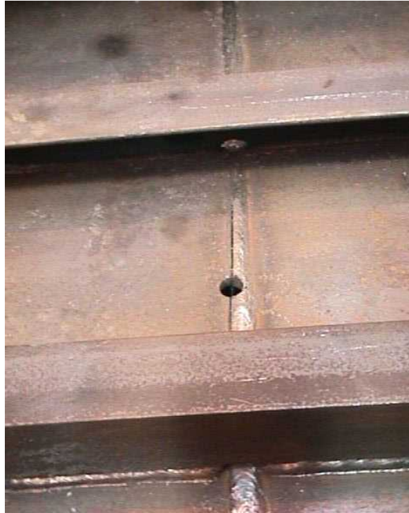
Figure 3-14: Typical initial crack introduced in specimen with reciprocating saw.
