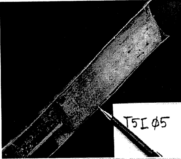
(a.) Permanganate impacted core at 5-ft. depth (the soil redox is dramatically elevated through core beyond the obvious purple staining).
