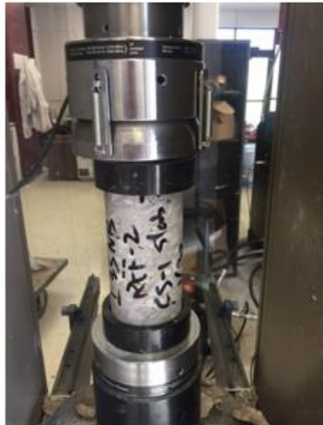
(a) CS test set-up
