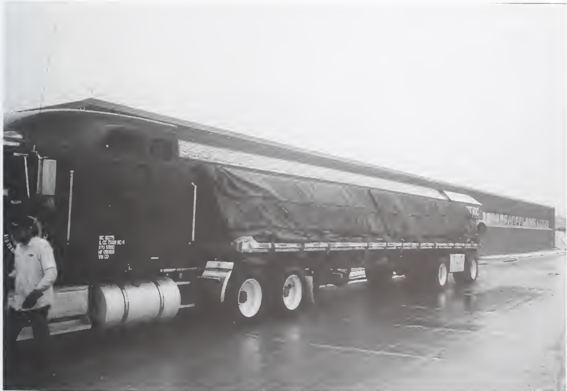
Pipe tubing being tarped and secured on flatbed
