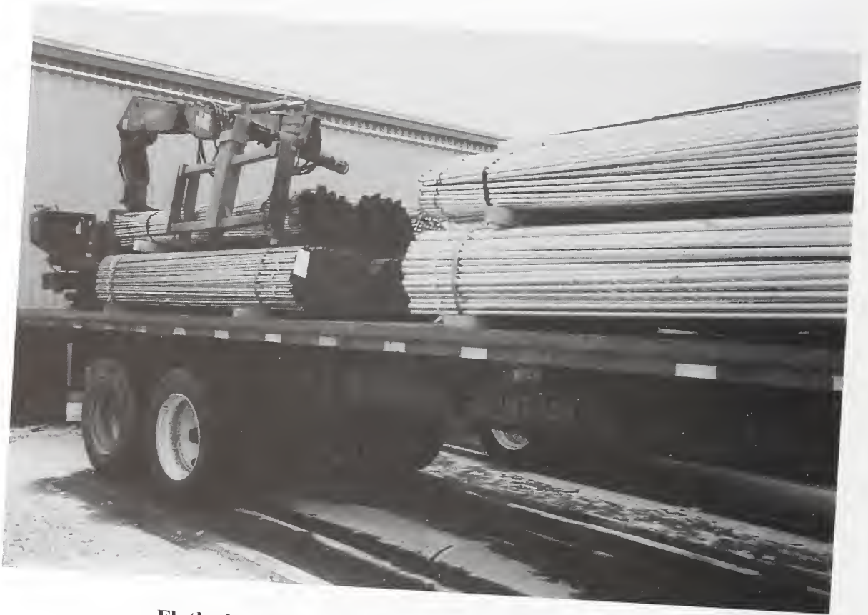
Flatbed with "kangaroo" lift for loads of pipe tubing
