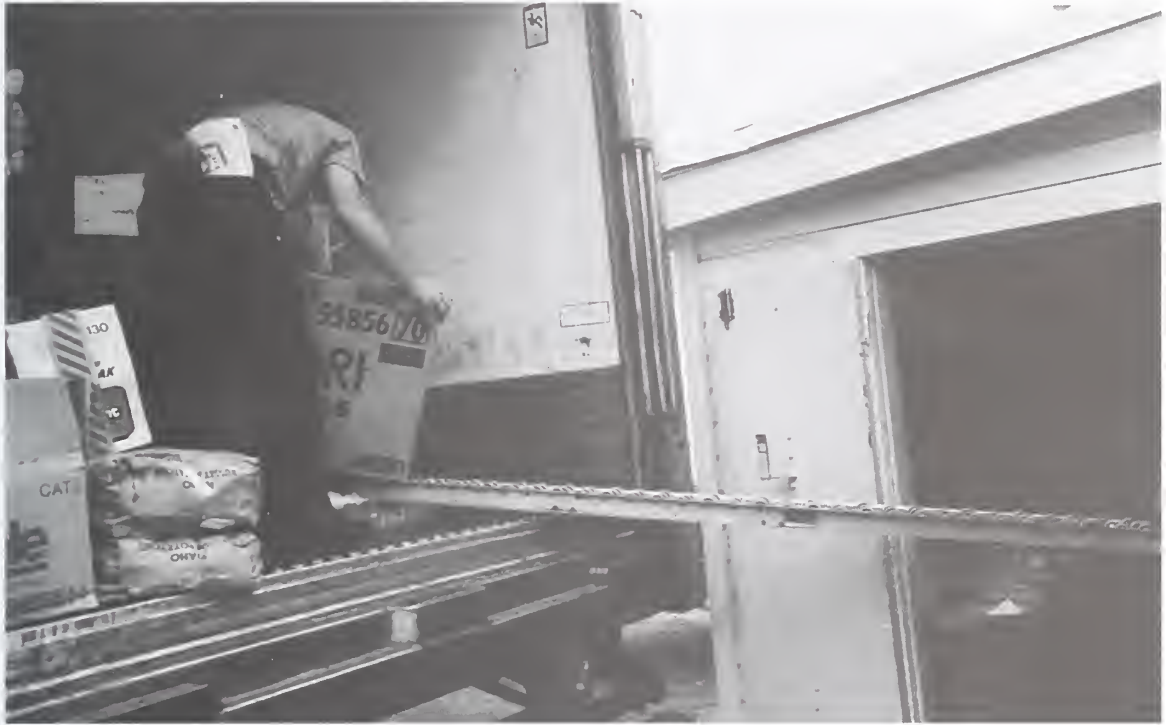
Roller conveyor set into place from truck to store receiving area
