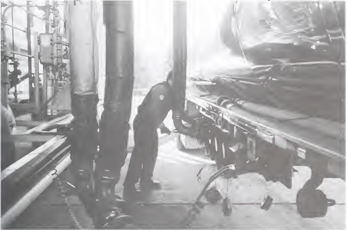
Driver hooks up connectors from gasoline storage tank pumps to tank truck compartments
