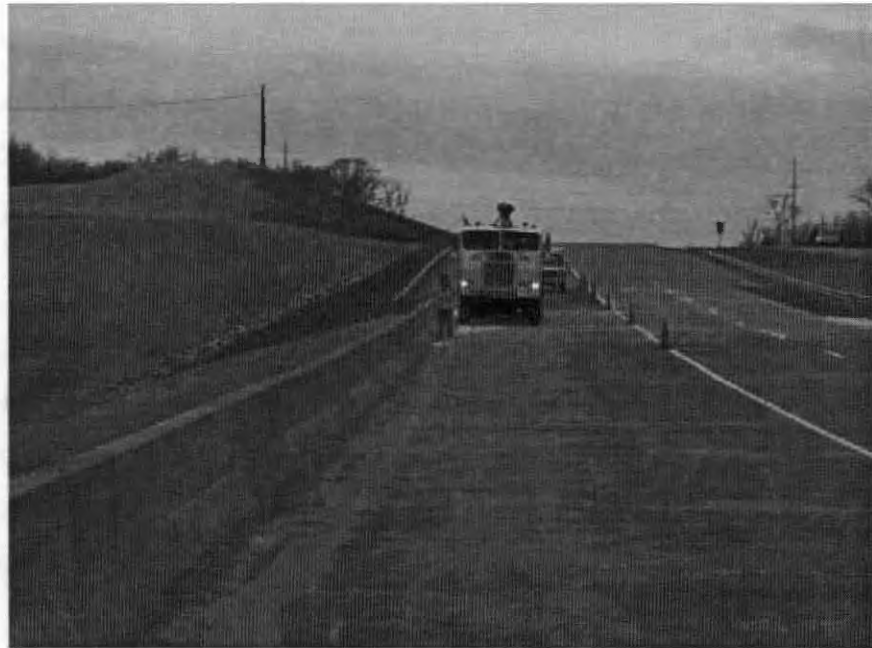
Figure 7.1 Load truck and markings on the bridge for the load test
