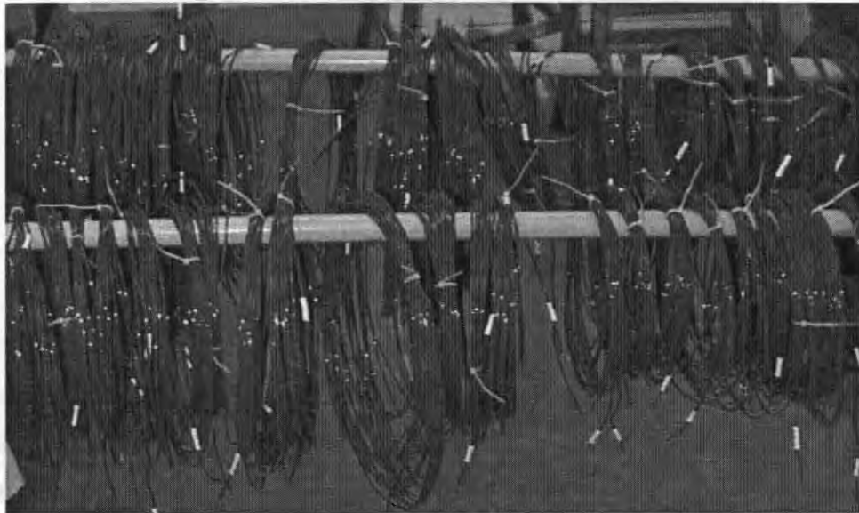
Figure 2.7 Thermocouples after welding, labeling and sealing
