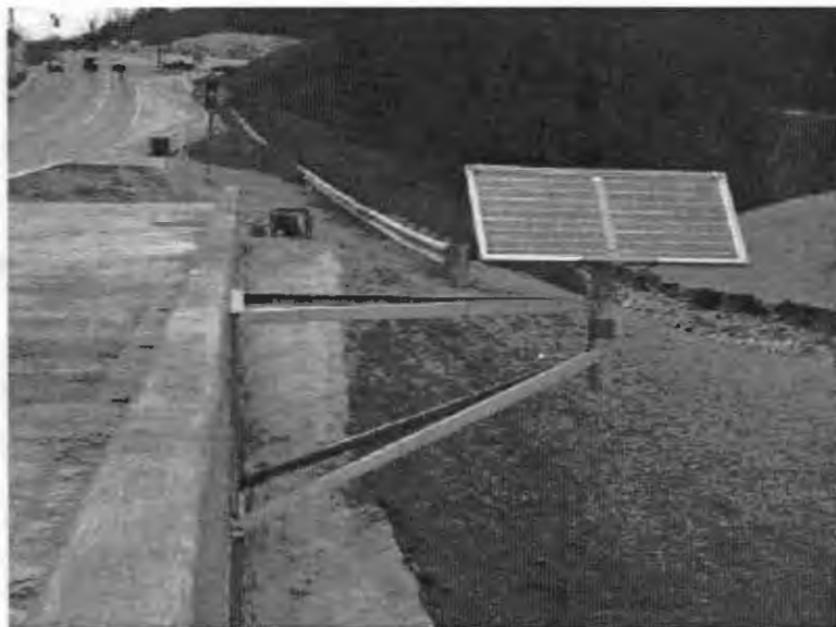
Figure 2.19 Solar power source for long-term remote data acquisition
