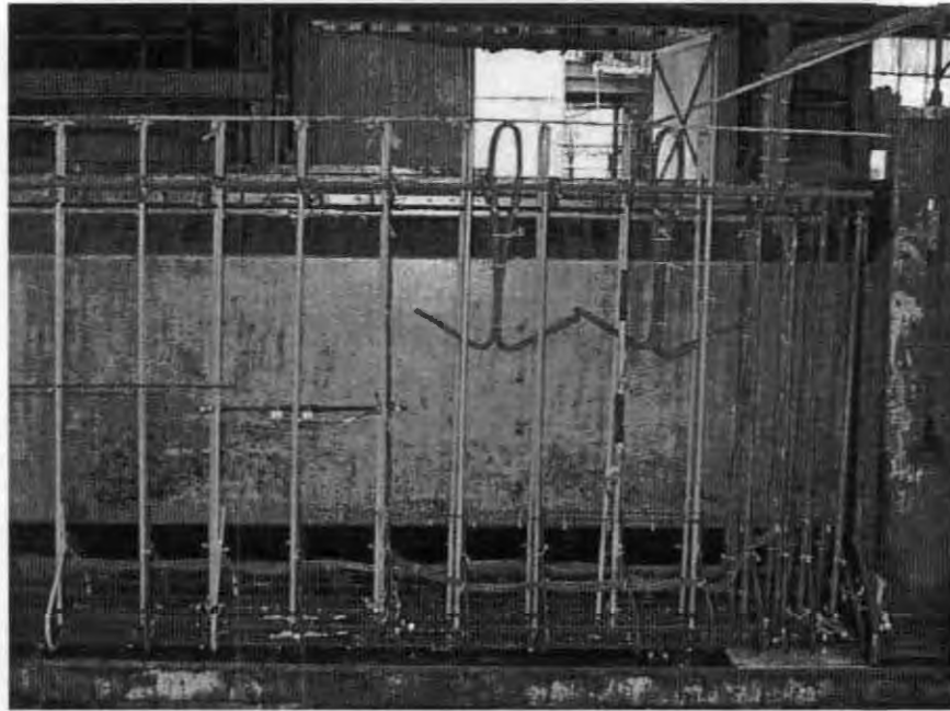
Figure 2.14 Photograph of the girder showing the end cross-section instrumentation, instrumented stirrup, and wire bundles
