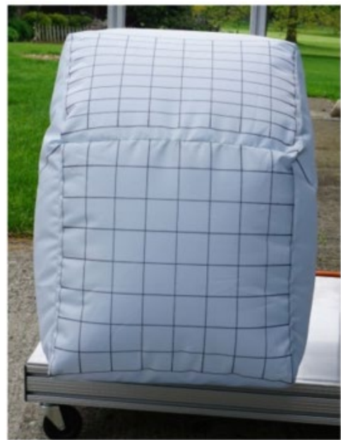
Figure 16. Compressed Air Inflation of the Airbag to Ascertain Geometry and Shape
