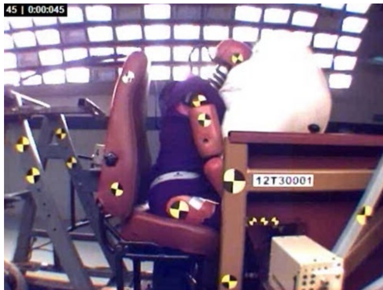
Figure 1. Sled Test Evaluation of the CEPS under a 23-g Trapezoidal Crash Pulse
