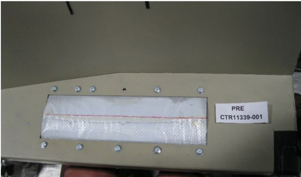
Figure 24. SIPS Module Cover and Tear Seam
