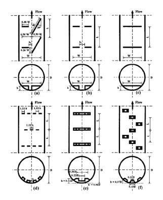
Figure 4.3. (a) Offset; (b) slotted weir; (c) weir baffle; (d) spoiler: (e) Alberta fishweir (AFW); and (f) Alberta fish baffle (Ead et al., 2002).
