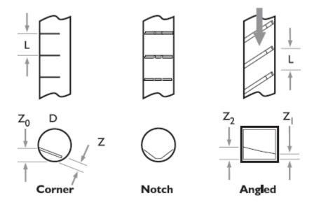
Figure 4.4. Recommended styles of baffles for round and box culverts in Washington (Bates et al., 2003).
