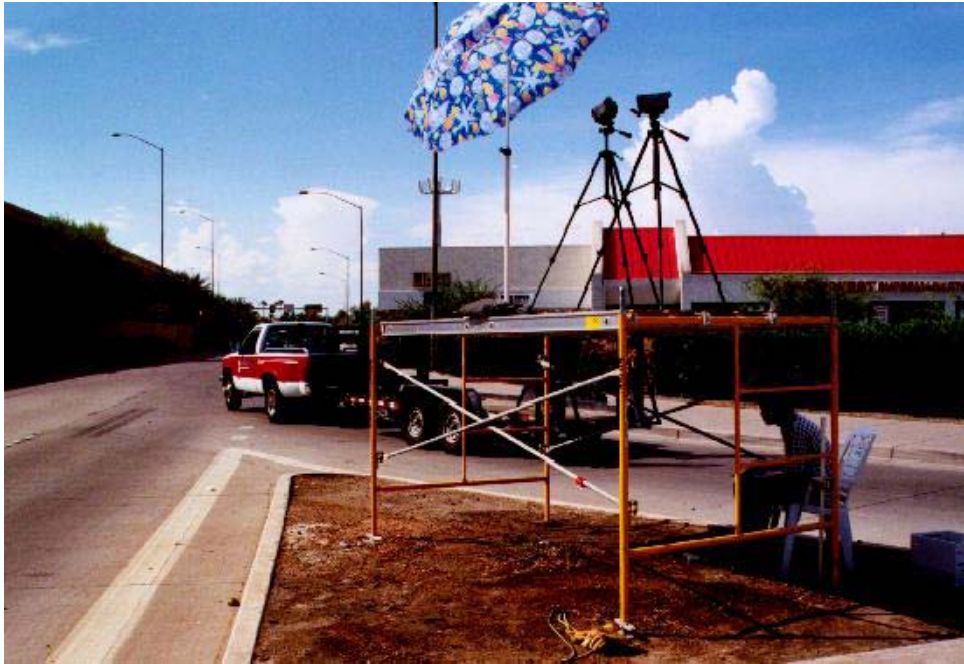
Figure 11. Typical video recording station.
