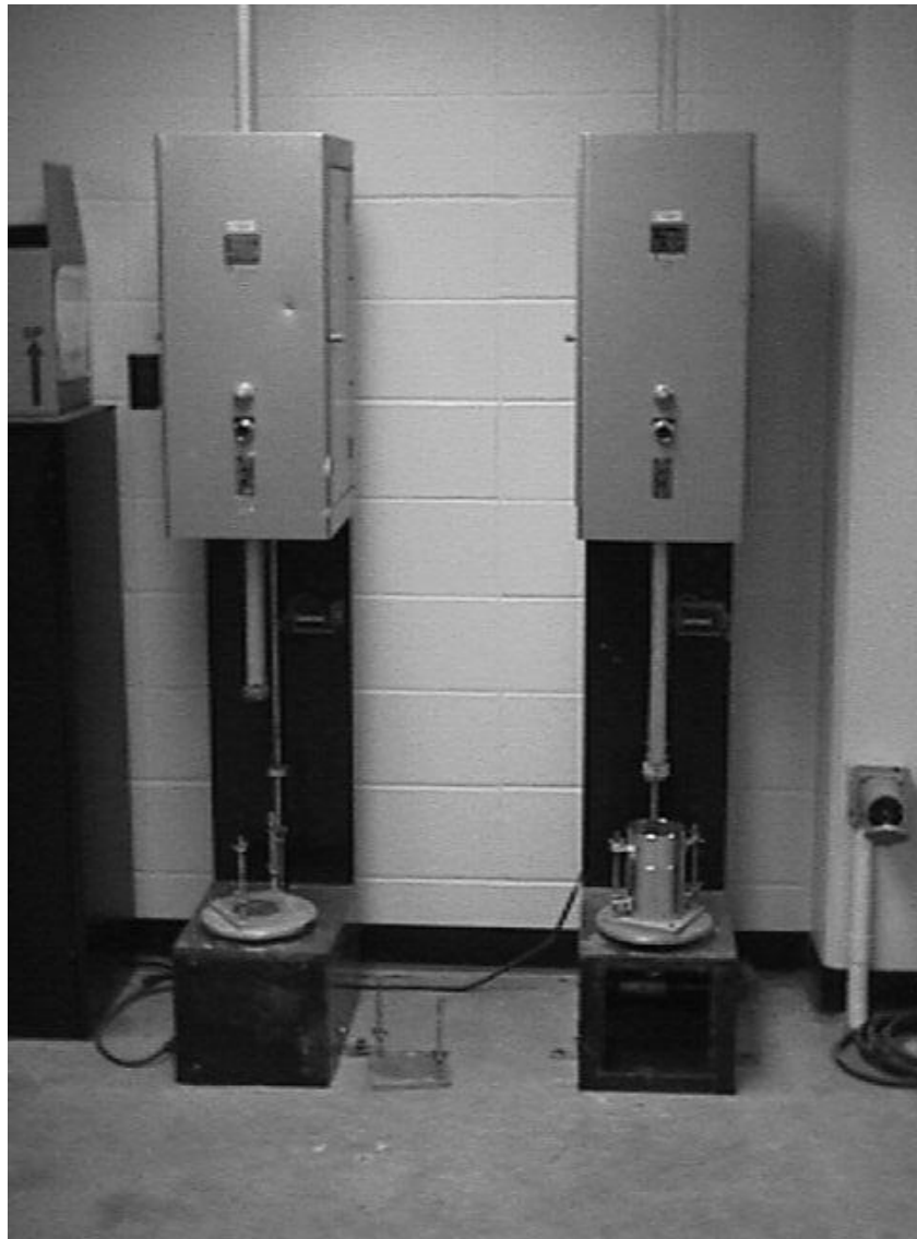
Figure 3.2: Mechanical rammer used for Modified Proctor (ASTM D-1557) Compaction Tests
