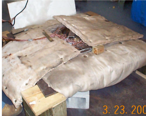
Figure 7.22 Induction heating coils for heating the hub-girder.
