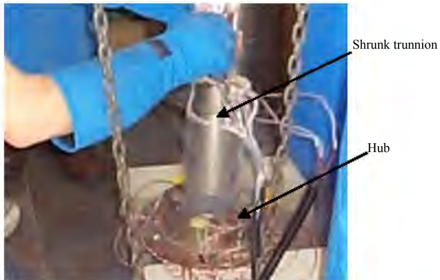
Figure 6.1 Cooled trunnion being inserted into the hub.
