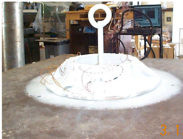
Figure 7.21 Hub-girder sub-assembly (Step 2 completed).
