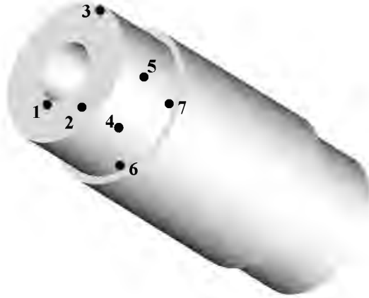
Figure 7.1 Gages on trunnion of AP1.
