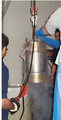
Figure 7.25 Cold trunnion taken out of the dewar.
