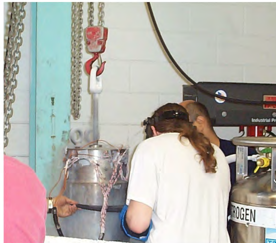
Figure 7.7 Measurement of shrunk diameter of cold trunnion with a micrometer.
