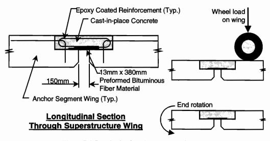
Figure 7.4 Longitudinal sections-cast-in-place joint
