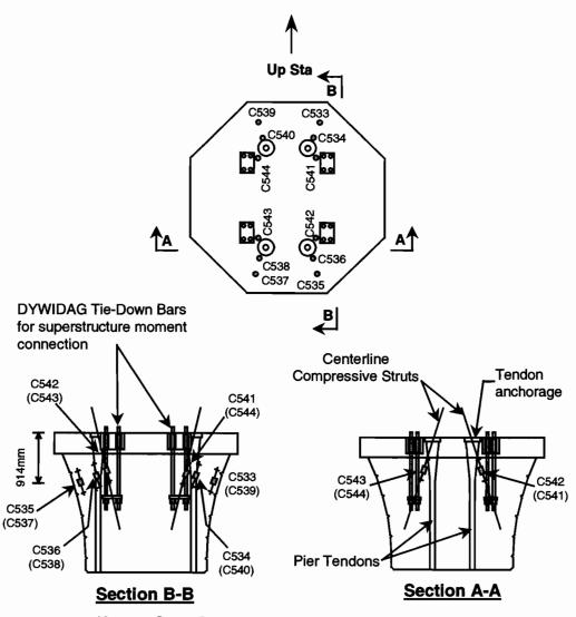
(Gauges C533, C535, C537, C539 located at 75mm clear cover.) (Gauges C534, C536, C538, C540 located at 455mm clear cover.)
