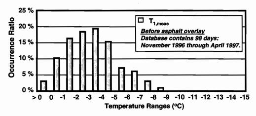
Figure 4.29 Statistical occurrence of daily minimum  $T_{1,meas}$  values on Ramp P before application of the asphalt blacktop
