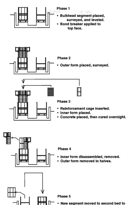
Figure 1.36 Typical segment-per-day casting sequence
