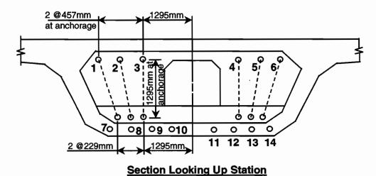
Figure 3.9 Mainlane girder D5 tendon profiles-end view
