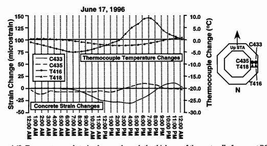
Figure 4.69 Temperature and strain changes through the thickness of the west wall of segment PC16-5
