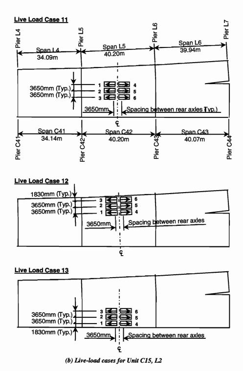
Figure 5.51 (a) and (b) Live-load cases for Unit C15, L2
