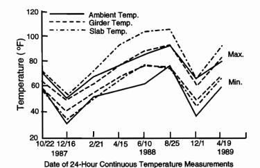
Figure 4.18 Temperature distributions through the depth of the section for the US 190 Atchafalaya River Bridge study by Pentas et al. [37]
