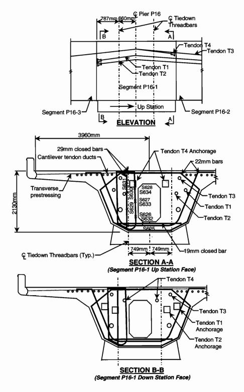
Figure 6.27 Ramp P girder anchor segment P16-1 details
