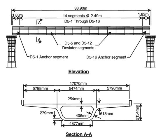
Figure 1.20 Cross section and elevation-Span D5
