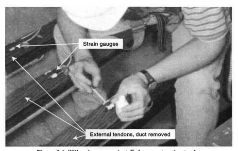
Figure 2.6 "S" series gauges installed on prestressing tendon
