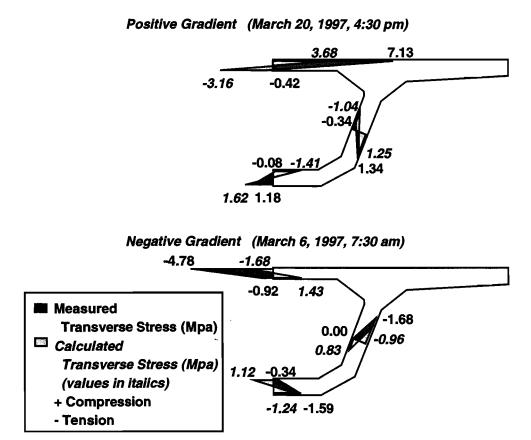
Figure 4.40 Comparison of measured and calculated transverse flexural stresses from positive and negative thermal gradients for P16-17
