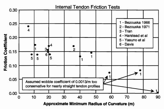
Figure 3.5 Results from previous friction tests
