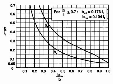
Figure 5.10 Values of the effective flange with coefficient  $b_m/b$ , for the given values of  $b/l_i$  (Figure 4.6.2.6.2-2 from the AASHTO LRFD Bridge Design Specifications [9])
