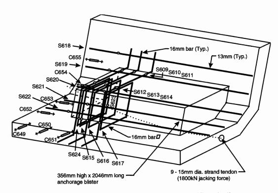
Figure 6.35 Ramp P girder segment P16-4 anchorage blister details
