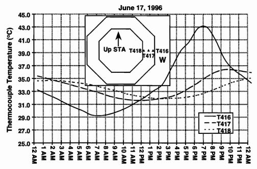
Figure 4.60 Temperatures recorded through the thickness of the west wall of segment PC16-5
