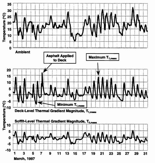
Figure 4.24 Measured thermal gradient magnitudes on Ramp P for the month of March 1997
