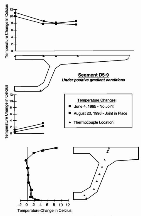
Figure 7.23 Measured temperatures for thermal gradient load case
