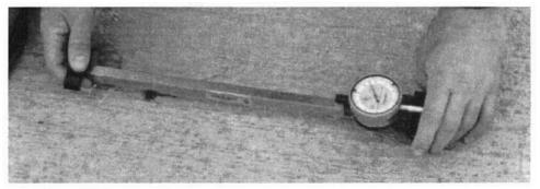
Figure 2.25 The Demec extensometer
