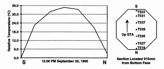
Figure 4.88 Maximum measured gradient shape during curing of capital segment PC16-8
