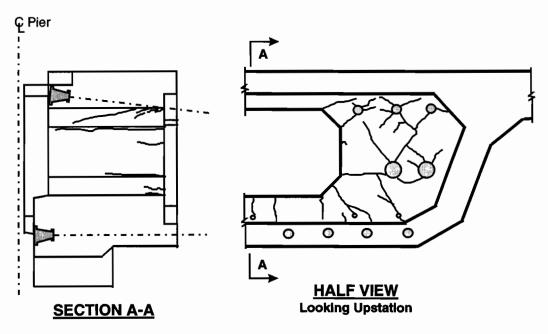
Figure 6.18 Crack patterns in segment D5-16 diaphragm
