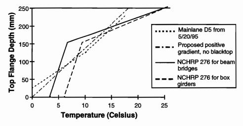
Figure 4.101 Recommended positive top flange design gradient for transverse design
