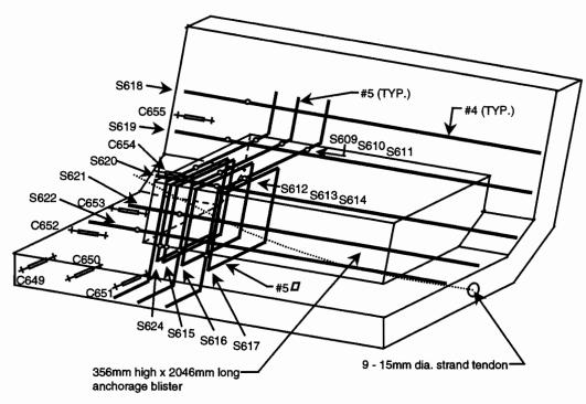
Figure 2.61 Segment P16-4 anchorage blister strain gauge locations
