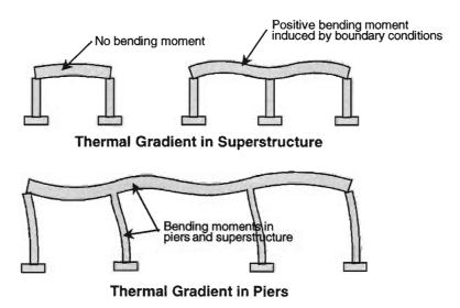
Figure 1.47 Structural response to thermal gradients
