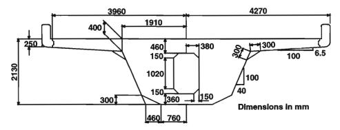
Figure 1.31 Ramp P anchor segment dimensions
