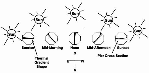
Figure 4.15 Thermal gradient orientations at different times of the day
