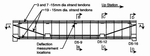
Figure 2.36 Elevation of mainlane girder D5 with deflection measurement locations
