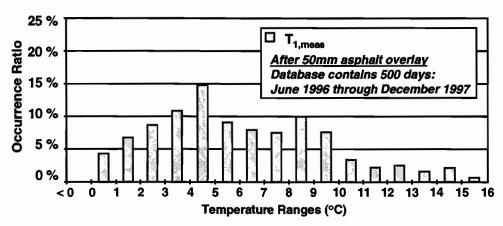
Figure 4.48 Statistical occurrence of daily maximum  $T_{I,meas}$  values on mainlane girder D5 after application of the asphalt blacktop
