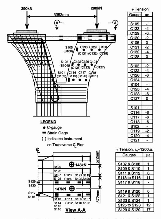
Figure 6.12 Measured strains in pier D6 capital from live-load case 5
