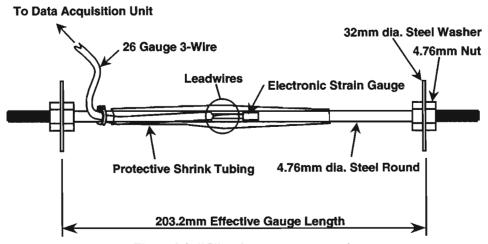
Figure 2.8 "C" series gauge construction
