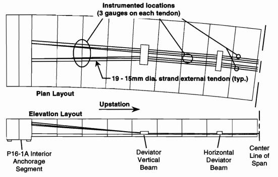
Figure 2.54 Ramp P tendon gauge locations
