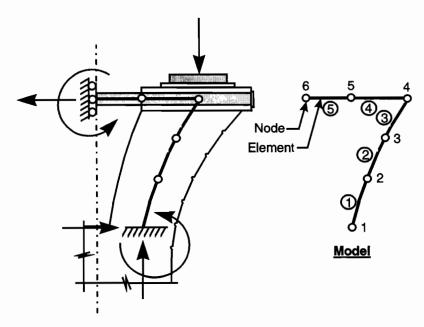
Figure 6.10 Frame model for mainlane pier D6
