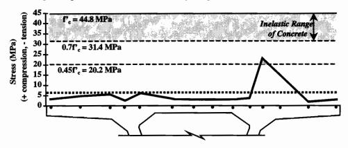
P16-17 (Midspan): Dead Load + Prestressing + Negative Thermal Gradient
