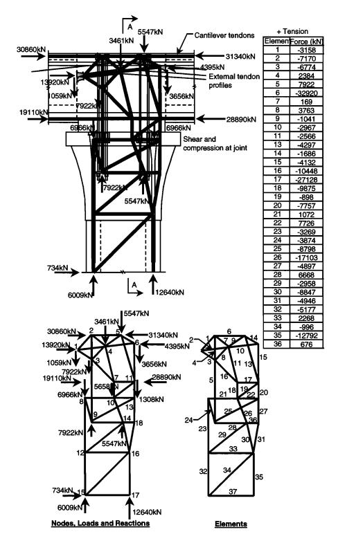
Figure 6.29 Strut-and-tie model at pier P16 - Side view
