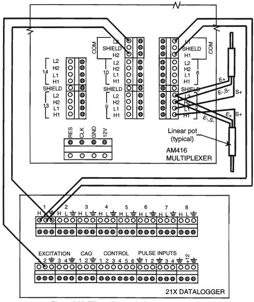
Figure 2.23 Wiring diagram for linear potentiometers
