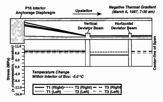
Figure 4.42 Measured stress changes in the Ramp P external tendons from the maximum negative gradient
