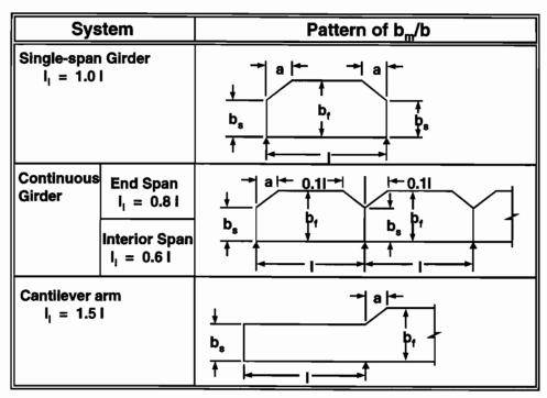
Figure 5.8 Pattern of effective flange width coefficients,  $b_f$  and  $b_s$  (Figure 4.6.2.6.2-1 from the AASHTO LRFD Bridge Design Specifications [9])
