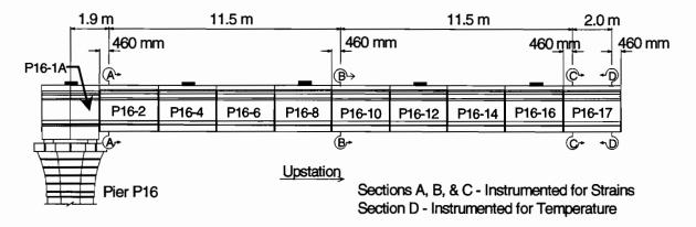
Tiltmeter plate location (symmetric about pier P16)
