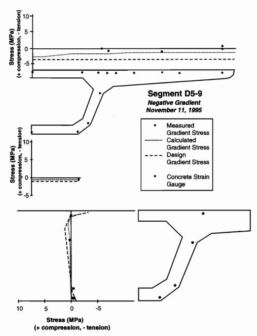
Figure 4.56 Comparison of measured and calculated negative thermal gradient stresses for segment D5-9 (November 11, 1995)
