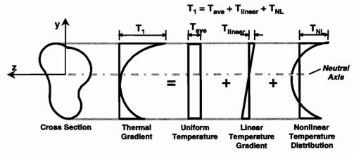
Figure 4.3 Components of a nonlinear thermal gradient
