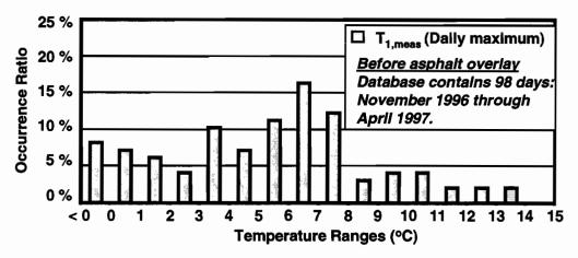
Figure 4.27 Statistical occurrence of daily maximum  $T_{I,meas}$  values on Ramp P before application of the asphalt blacktop
