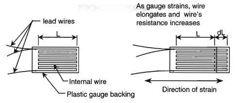
Figure 2.3 Electronic strain gauge
