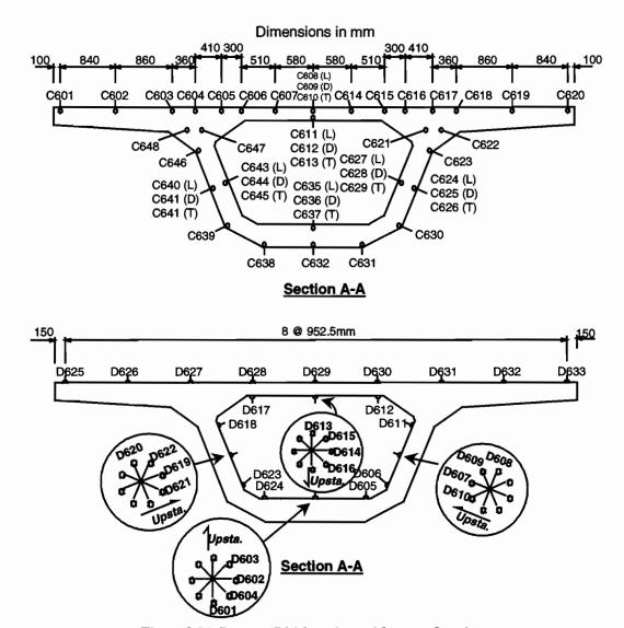
Figure 2.56 Segment P16-2 sections with gauge locations
