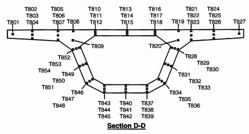
Figure 2.59 Segment P16-17 section with thermocouple locations
