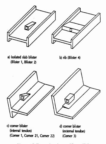
Figure 6.7 Types of anchorage blisters [54]
