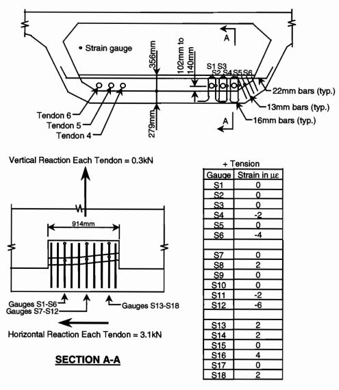
Figure 6.15 Measured strains in the deviator reinforcing bars from live-load case 2
