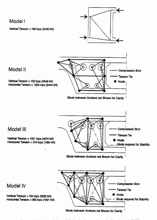
Figure 6.5 Strut-and-tie model of a diaphragm from the San Antonio Y [7]
