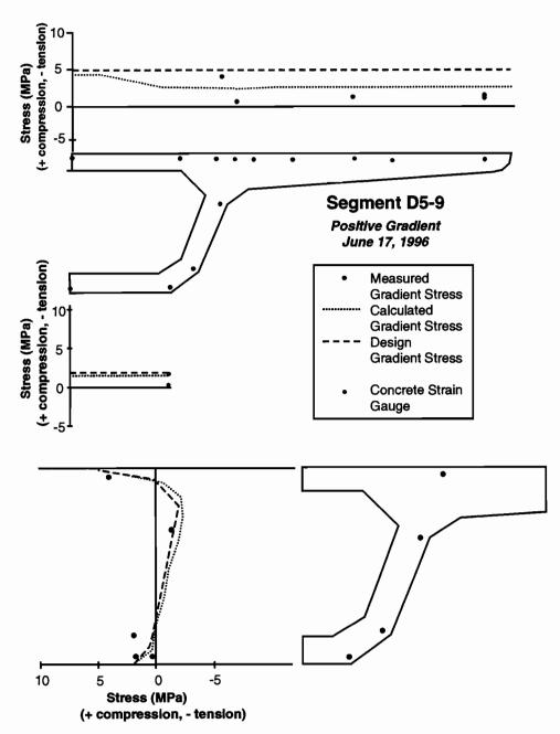
Figure 4.54 Comparison of measured and calculated positive thermal gradient stresses for segment D5-9 (June 17, 1996)
