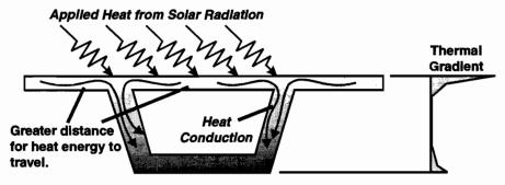
Figure 4.2 The effects of cross-section shape on thermal gradient shape
