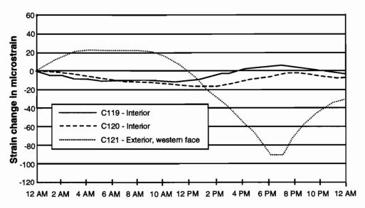
Figure 4.95 Measured concrete strains in the pier D6 capital over a sunny day
