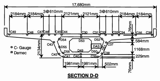
Figure 2.40 Longitudinal strain gauge locations for segment D5-16
