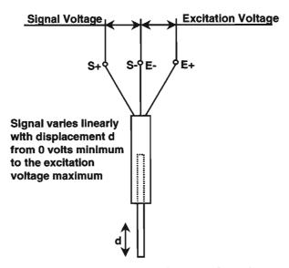
Figure 2.14 Linear potentiometer schematic
