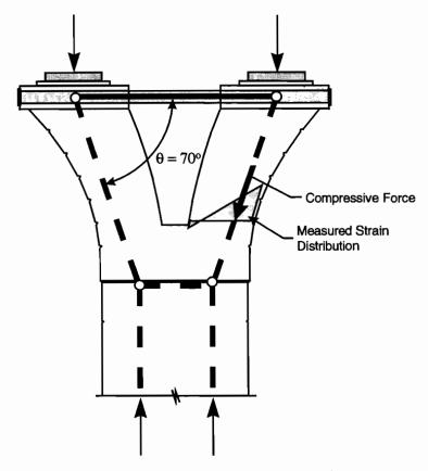
Figure 6.9 Simple strut-and-tie model for mainlane pier D6
