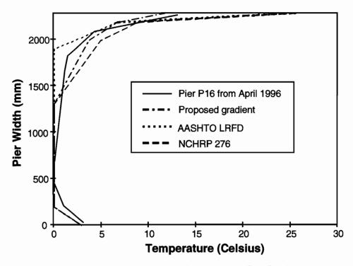
Figure 4.104 Recommended positive design gradient for piers
