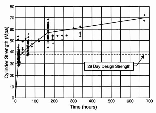
Figure 2.69 Concrete compressive strengths for mainlane D
