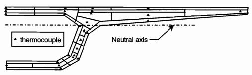
Figure 4.51 Division of the mainlane girder D5 cross section into tributary areas for each thermocouple gauge
