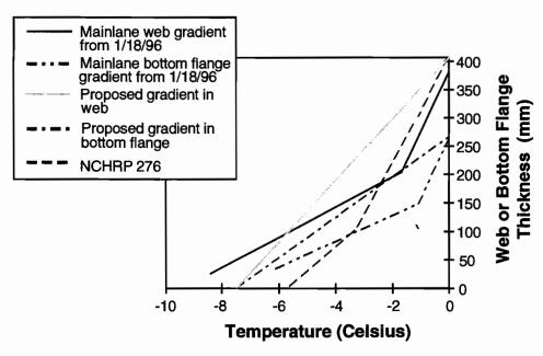
Figure 4.103 Recommended web and bottom flange negative design gradient for transverse design
