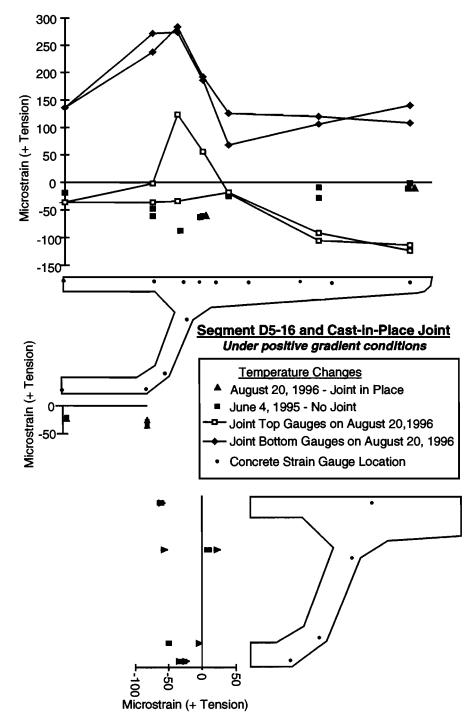
Figure 7.25 Measured strains in segment D5-16 and cast-in-place joint from thermal gradient load case
