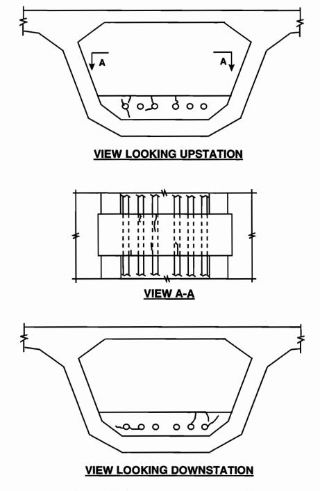
Figure 6.33 Crack patterns in segment P16-10
