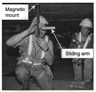
Figure 2.28 Taking deflection measurements
