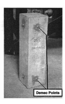
Figure 2.64 Concrete modulus of elasticity test specimen
