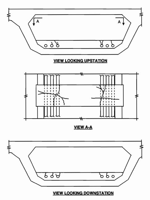
Figure 6.14 Crack patterns in the segment D5-12 deviator
