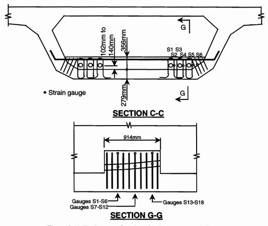
Figure 2.41 Strain gauge locations for deviator segment D5-12
