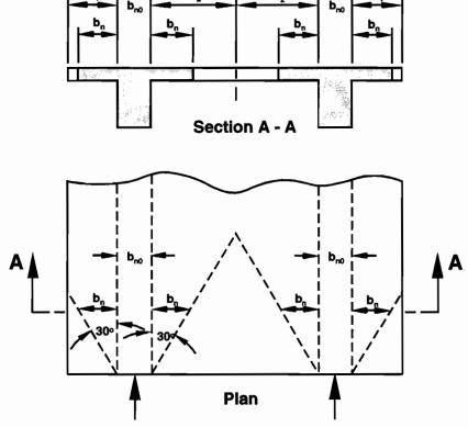
Figure 5.11 Effective flange widths,  $b_m$  for normal forces (Figure 4.6.2.6.2-4 from the AASHTO LRFD Bridge Design Specifications [9])
