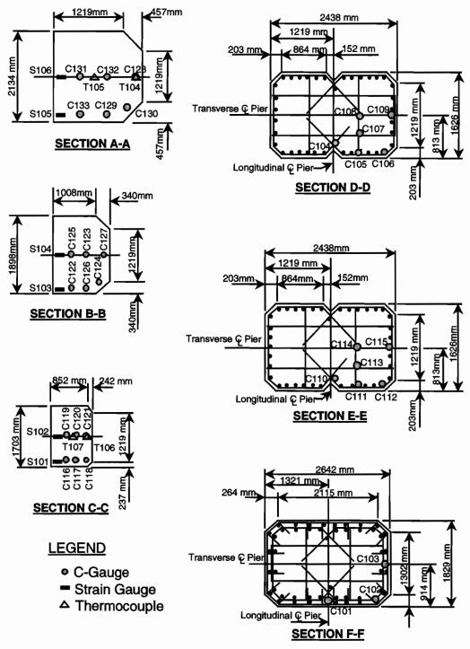
Figure 2.34 Y-pier sections showing gauge locations
