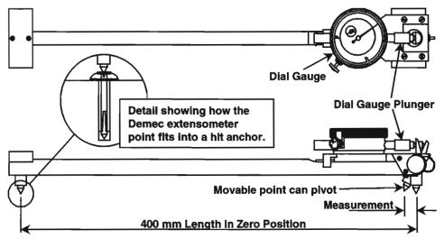
Figure 2.26 Demec extensometer schematic
