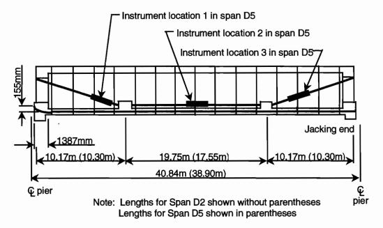
Figure 3.8 Mainlane girder D5 tendon profiles-elevation
