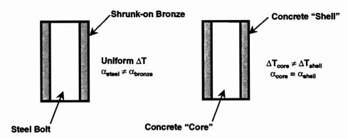
Figure 4.14 Response of solid column to thermal gradients
