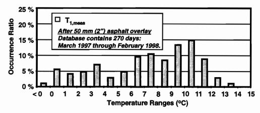
Figure 4.28 Statistical occurrence of daily maximum  $T_{1,meas}$  values on Ramp P after application of the asphalt blacktop
