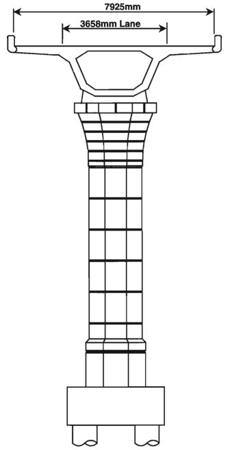
Figure 1.8 Ramp superstructure section
