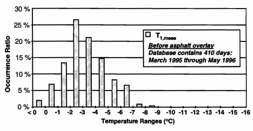
Figure 4.49 Statistical occurrence of daily minimum  $T_{I,meas}$  values on mainlane girder D5 before application of the asphalt blacktop
