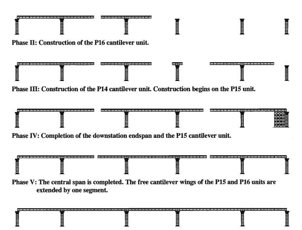
Phase VI: Final bearing adjustaments are made on P17. The upstation 54.9 m span is completed. The same process is repeated on the downstation half of the bridge.
