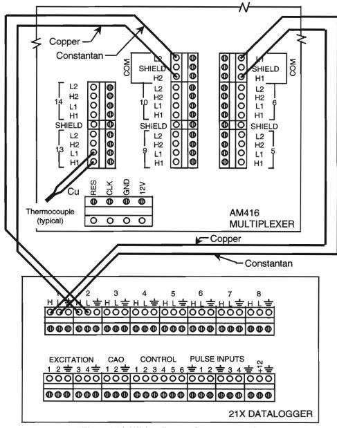
Figure 2.22 Wiring diagram for thermocouples
