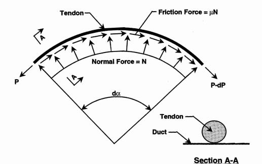
Figure 3.1 Friction loss model
