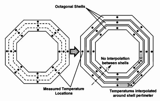
Figure 4.70 Concentric octagonal model for temperature representation
