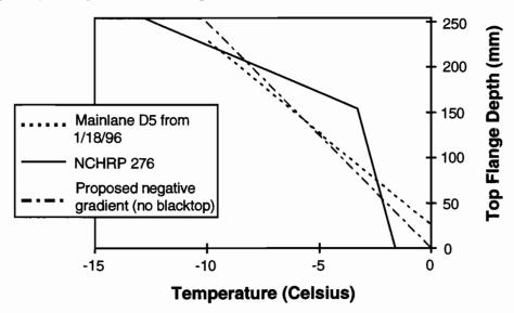
Figure 4.102 Recommended top flange negative design gradient for transverse design
