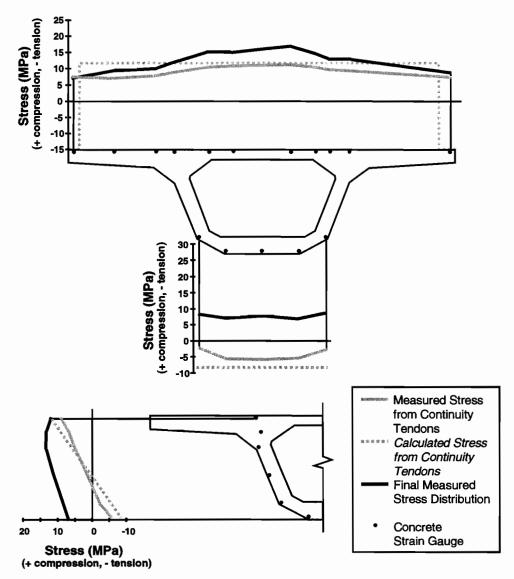
Figure 5.39 Longitudinal stresses in segment P16-2 after stressing of the continuity tendons for span P16
