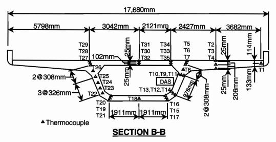
Figure 2.39 Thermocouple locations for segment D5-9
