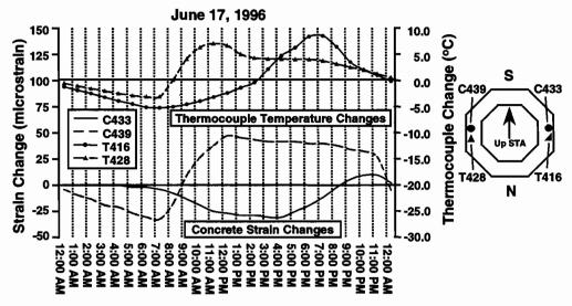
Figure 4.67 Temperature and strain changes on the east-west axis of segment PC16-5
