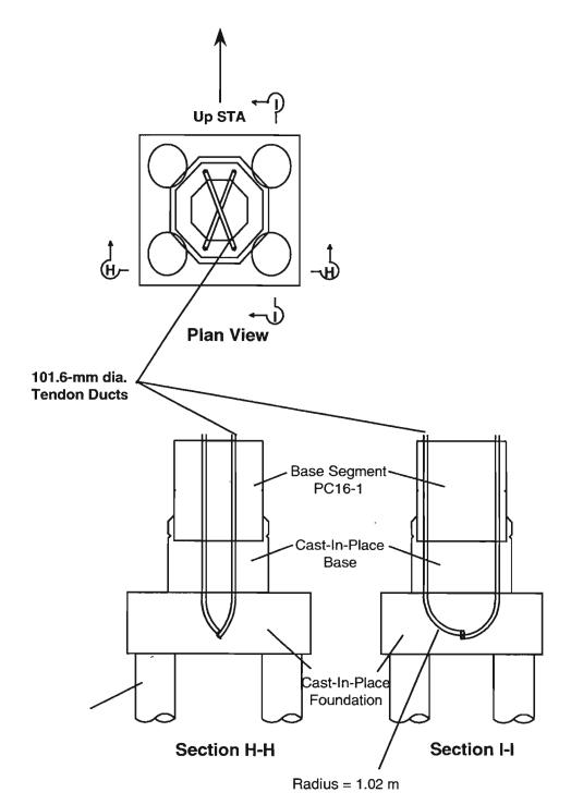
Figure 1.40 U-shaped tendon ducts located in pier foundation
