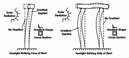
Figure 4.13 Response of a multiple column bridge pier to a thermal gradient
