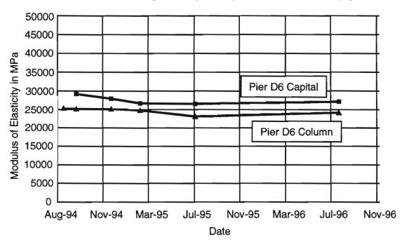
Figure 2.65 Modulus of elasticity test results for mainlane pier D6
