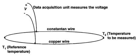
Two temperatures induce a current in the circuit.
