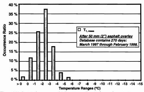
Figure 4.30 Statistical occurrence of daily minimum  $T_{1,meas}$  values on Ramp P after application of the asphalt blacktop
