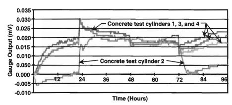
Figure 2.21 C-gauge output recorded during temperature effects test
