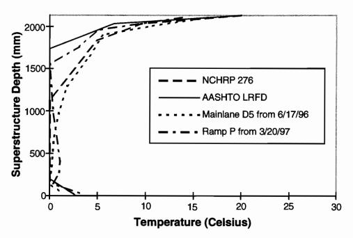
Figure 4.98 Positive design gradients and measured gradients, 50mm of blacktop
