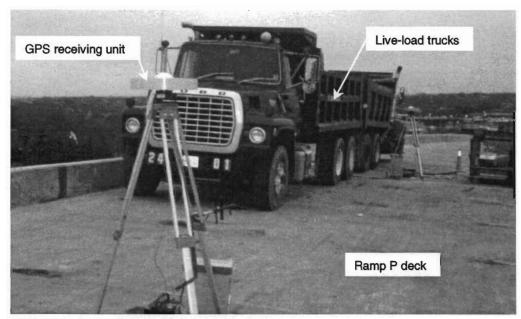
Figure 2.29 GPS deflection measurement equipment
