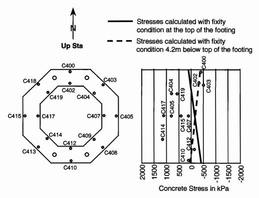
Figure 5.64 Stresses in pier segment PC16-1 from placement of superstructure segment P16-17
