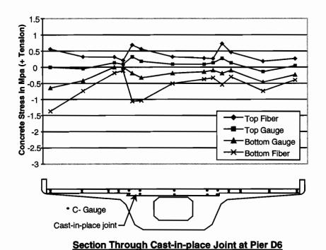
Figure 7.10 Cast-in-place joint stresses-load case 3
