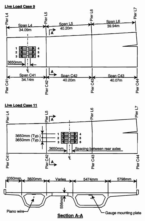
Figure 7.20 Live-load cases-Units C15 and L2
