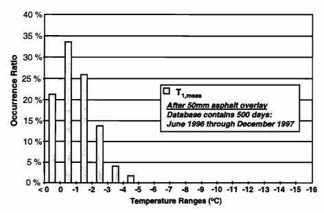
Figure 4.50 Statistical occurrence of daily minimum  $T_{1,meas}$  values on mainlane girder D5 after application of the asphalt blacktop
