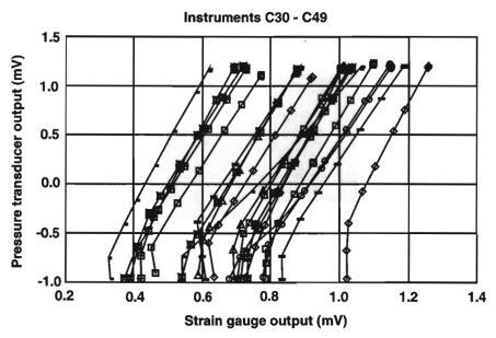
Figure 2.10 C-gauge calibration
