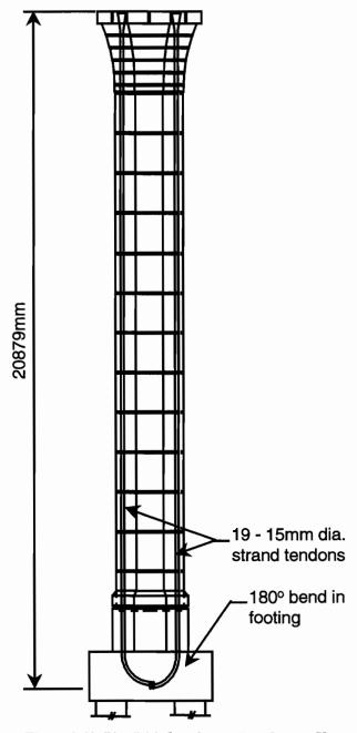
Figure 3.13 Pier P16 elevation and tendon profiles
