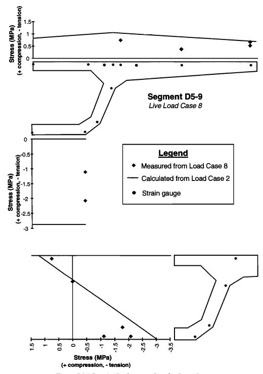
Figure 5.26 Longitudinal stresses from load case 8
