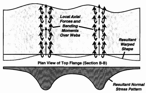
Figure 4.10 Girder response to an applied positive thermal gradient when warping occurs
