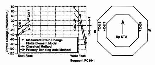
Figure 4.75 Calculated strain changes and strain changes recorded by strain gauges in segment PC16-1, east-west axis, maximum positive gradient
