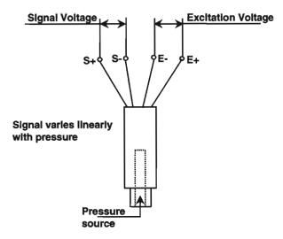
Figure 2.15 Pressure transducer schematic
