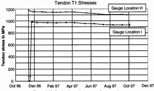
Figure 3.12 Strain change in ramp tendons over time
