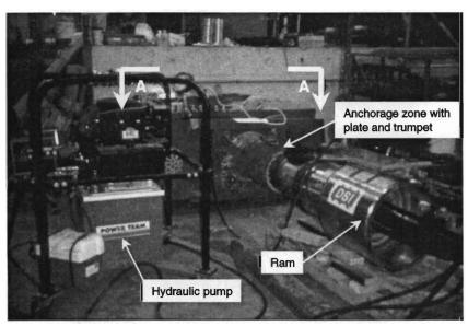
Figure 2.32 Epoxy sleeves tested during the bench test
