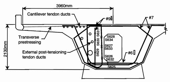
Figure 2.55 Anchor segment P16-1A section with gauge locations
