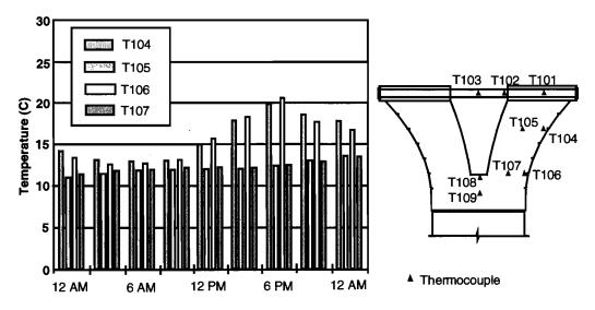
Figure 4.90 One-day cycle of pier D6 capital concrete temperatures
