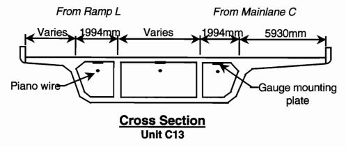
Figure 5.57 Cross section of Unit C13
