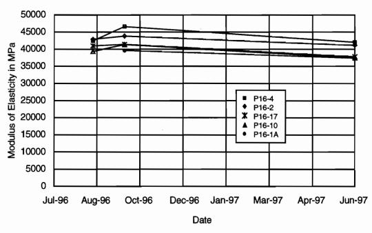
Figure 2.68 Modulus of elasticity test results for Ramp P superstructure
