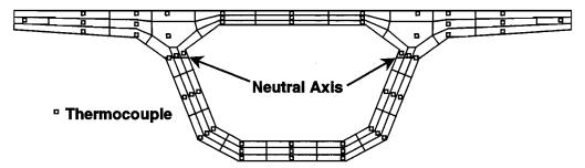
Figure 4.31 Division of the Ramp P cross section into tributary areas for each thermocouple gauge
