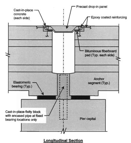
Figure 7.2 Original joint details from contract plans for U.S. 183
