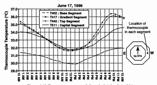
Figure 4.61 Temperatures measured along the height of pier P16
