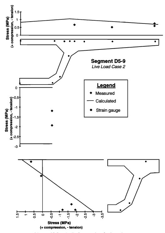
Figure 5.25 Longitudinal stresses from load case 2
