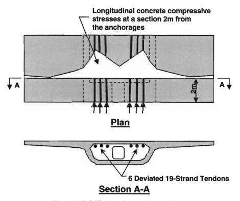
Figure 1.49 Diffusion of post-tensioning forces
