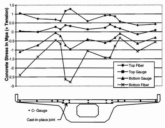
Section Through Cast-in-place Joint at Pier D6
