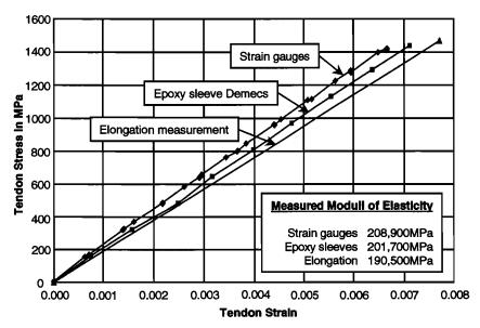
Figure 3.7 Instrumentation calibration from bench test
