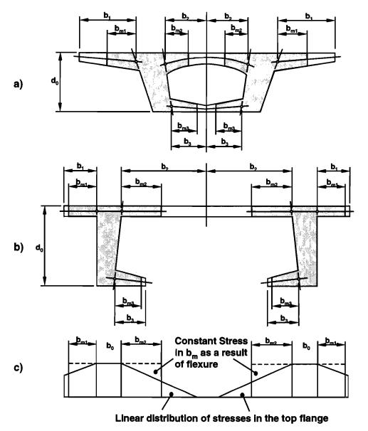
Figure 5.9 Cross sections and corresponding effective flange widths,  $b_{mo}$  for flexure and shear (Figure 4.6.2.6.2-3 from the AASHTO LRFD Bridge Design Specifications [9])
