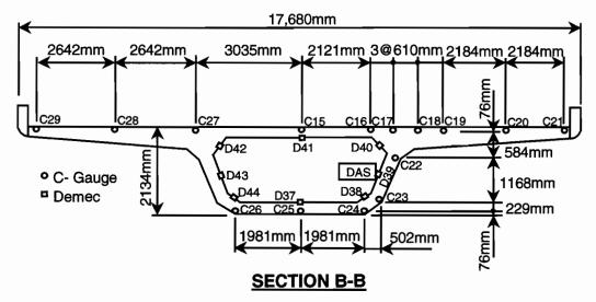
Figure 2.38 Strain gauge locations for segment D5-9
