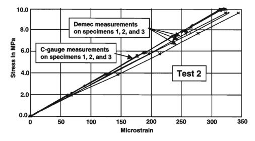
Figure 2.9 C-gauge tested against the Demec extensometer
