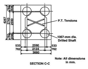
Figure 1.34 Typical sections: large ramp pier
