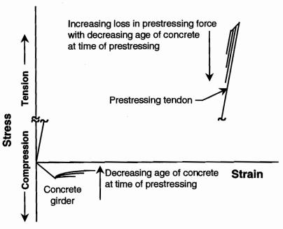
Figure 3.2 Prestress force loss from creep and shrinkage
