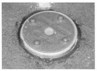
Figure 2.30 Tiltmeter gauge mounting plate
