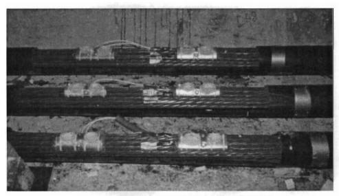
Figure 2.31 Epoxy sleeve strain measurement system
