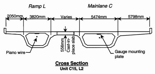
Figure 5.50 Cross section of Unit C15, L2
