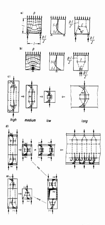
Figure 6.1 Typical strut-and-tie models [52]
