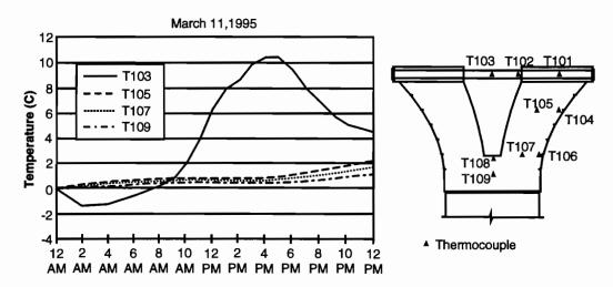
Figure 4.92 Pier D6 capital pipe temperature versus concrete core temperature, typical sunny day
