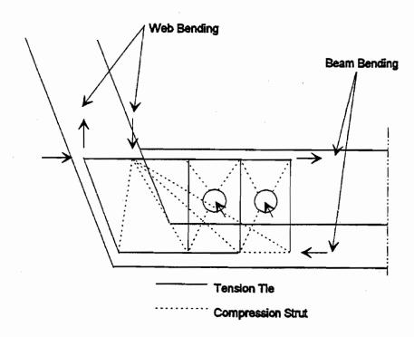
Figure 6.6 Strut-and-tie model of a deviator from the San Antonio Y (after Roberts et al [7])
