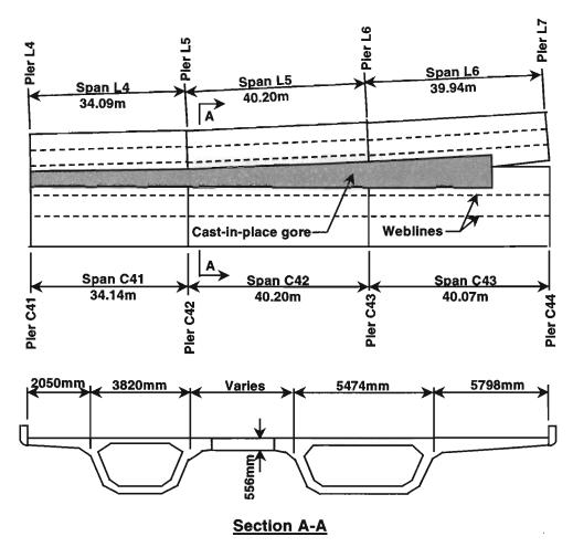
Figure 1.45 Plan and section of modified Unit C15-L2
