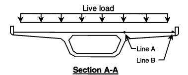
Figure 5.2 Top flange stresses in a continuous box girder
