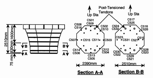
Figure 2.50 Segment PC16-8 bottom C-gauge locations
