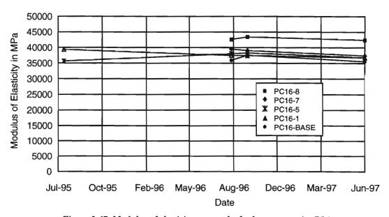
Figure 2.67 Modulus of elasticity test results for large ramp pier P16
