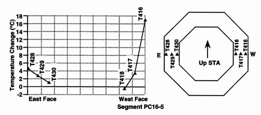
Figure 4.74 Temperature changes along the east-west axis recorded by thermocouples in segment PC16-5, maximum positive gradient
