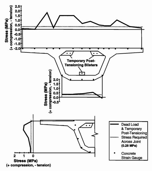
Figure 5.33 Diffusion of force from temporary post-tensioning in segment P16-10
