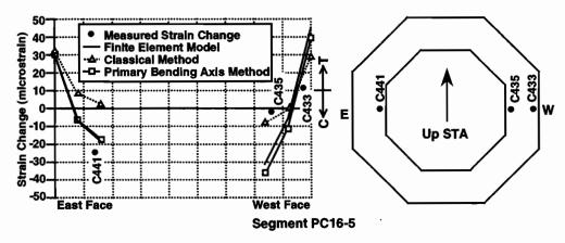
Figure 4.82 Calculated strain changes and strain changes recorded by strain gauges in segment PC16-5, east-west axis, maximum negative gradient
