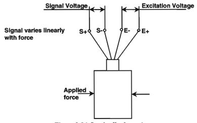
Figure 2.16 Load cell schematic
