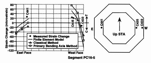
Figure 4.76 Calculated strain changes and strain changes recorded by strain gauges in segment PC16-5, east-west axis, maximum positive gradient
