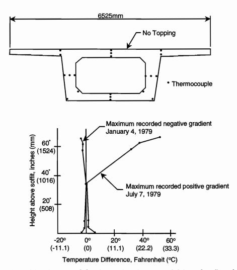
Figure 4.16 Thermocouple locations and maximum recorded thermal gradients for the Hoffman, McClure and West study [32]
