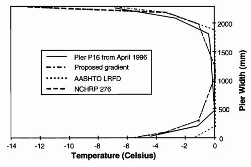
Figure 4.105 Recommended negative design gradient for piers
