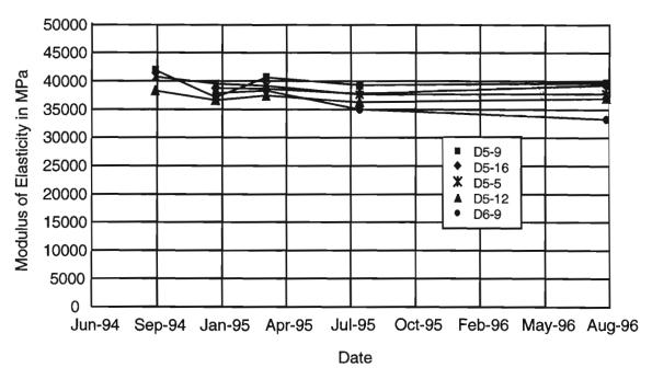
Figure 2.66 Modulus of elasticity test results for mainlane superstructure Unit D2
