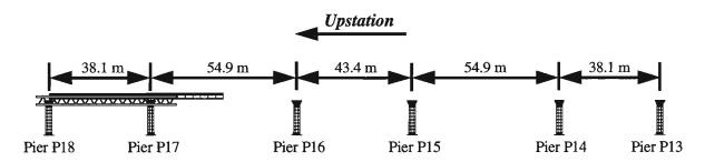
Phase I: Construction of the P17 cantilever unit and the completion of the upstation endspan.
