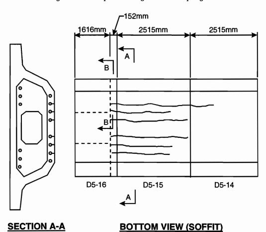
Figure 6.19 Crack patterns in the bottom flange of segments D5-16, D5-15 and D5-14
