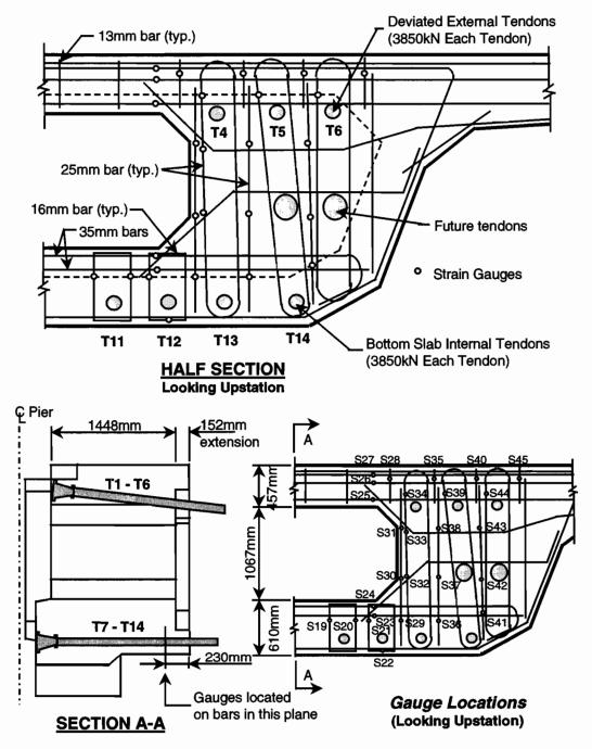
Figure 6.17 Mainlane anchor segment D5-16 details
