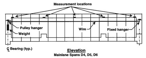
Figure 2.27 Piano wire deflection measuring system schematic
