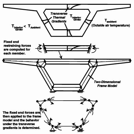
Figure 4.8 Transverse analysis for thermal gradients
