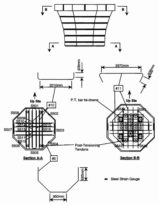
Figure 2.51 Segment PC16-8 S-gauge locations on rebar
