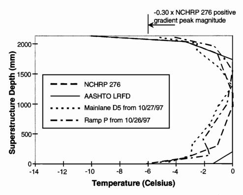
Figure 4.100 Negative design gradients and measured gradients, 50mm of blacktop
