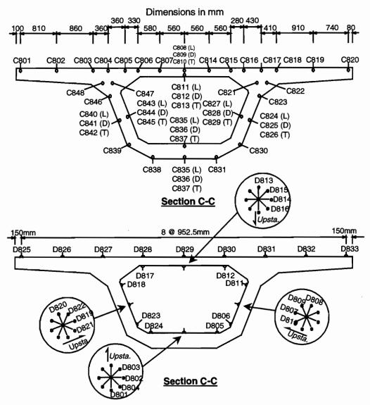
Figure 2.58 Segment P16-17 sections with strain gauge locations
