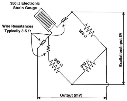
Figure 2.4 Wheatstone bridge circuit
