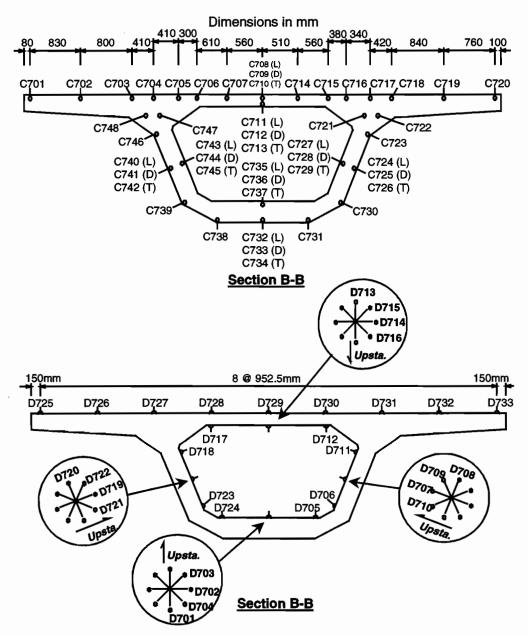
Figure 2.57 Deviator segment P16-10 sections with gauge locations
