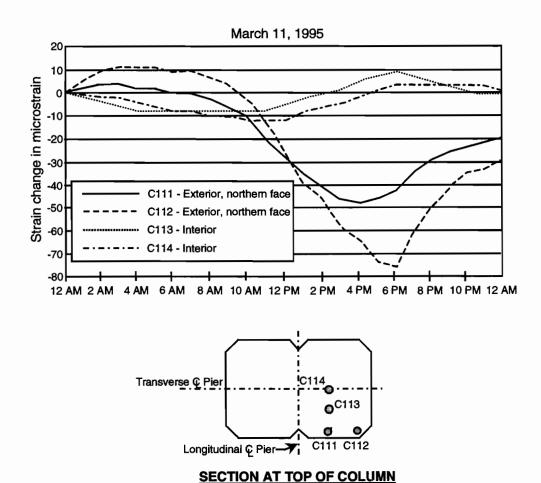
Figure 4.96 Measured concrete strains at the top of pier D6 column over a sunny day
