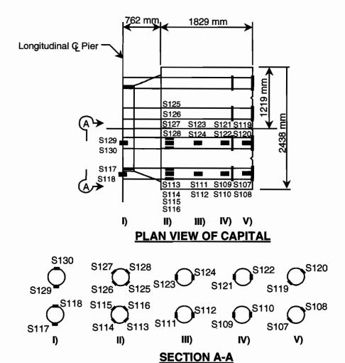
Figure 2.35 Plan view of Y-pier showing gauge locations
