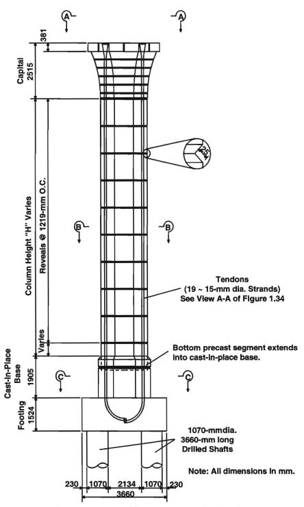
Figure 1.33 Typical large ramp pier: elevation view
