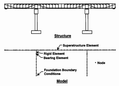
Figure 5.5 Beam model of a box girder bridge
