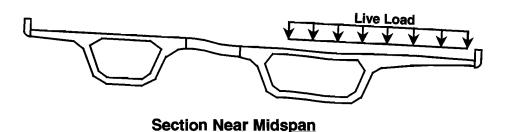
Figure 5.4 Response of twin single-cell box girders to live load
