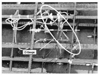
Figure 2.11 Installation of C-gauges
