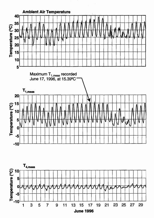
Figure 4.44 Measured thermal gradients on mainlane girder D5 for the month of June 1996
