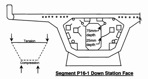
Figure 6.28 Crack patterns in segment P16-1
