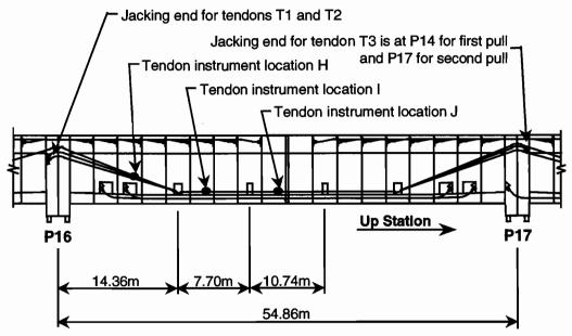
Figure 3.10 Ramp P tendon geometry-elevation
