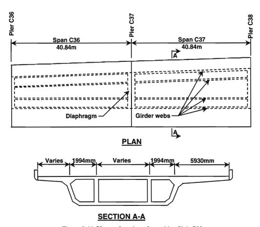
Figure 1.44 Plan and section of transition Unit C13
