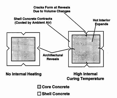
Figure 4.86 Mechanism for cracking of large monolithic members during curing
