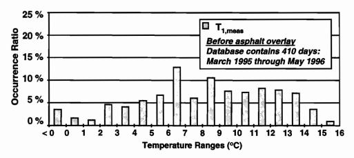
Figure 4.47 Statistical occurrence of daily maximum  $T_{l,meas}$  values on mainlane girder D5 before application of the asphalt blacktop
