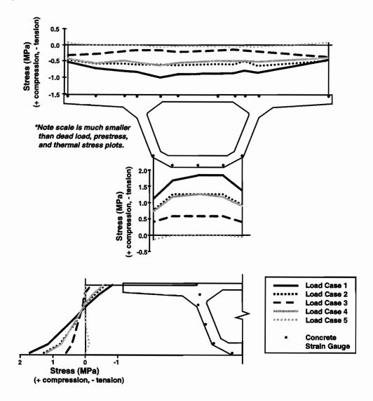
Figure 5.46 Measured live-load longitudinal stresses in segment P16-2
