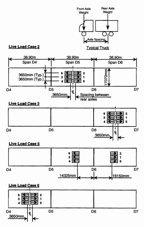
Figure 7.8 Live-load cases for Unit D2
