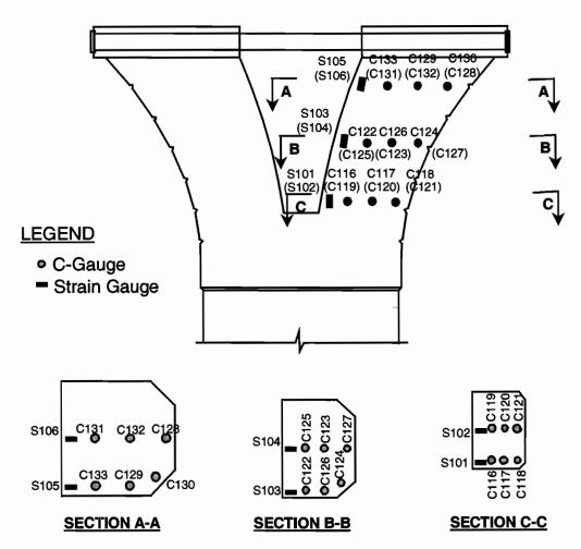
Figure 4.94 Pier D6 gauge locations
