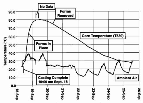
Figure 4.87 Comparison of internal curing temperature to ambient air temperature, capital segment PC16-8
