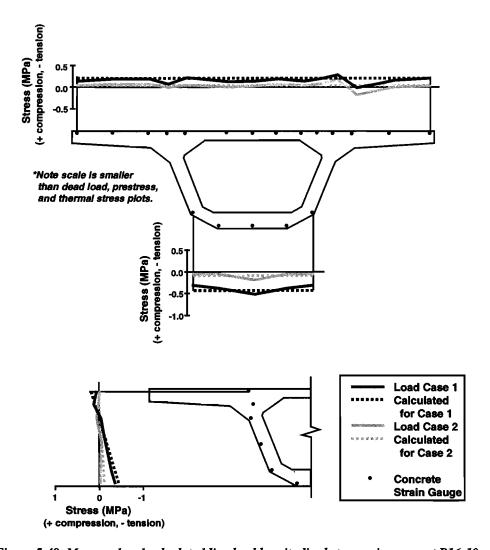
Figure 5.48 Measured and calculated live-load longitudinal stresses in segment P16-10
