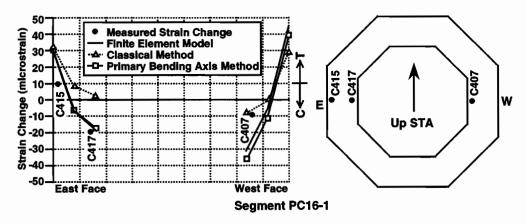
Figure 4.81 Calculated strain changes and strain changes recorded by strain gauges in segment PC16-1, east-west axis, maximum negative gradient
