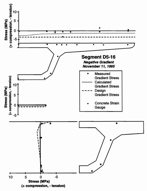
Figure 4.57 Comparison of measured and calculated negative thermal gradient stresses for segment D5-16 (November 11, 1995)
