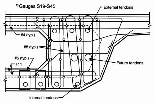
Figure 2.42 Strain gauge locations for anchor segment D5-16
