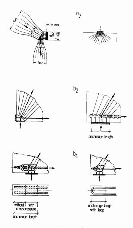
Figure 6.4 Anchorage details at nodes [52]
