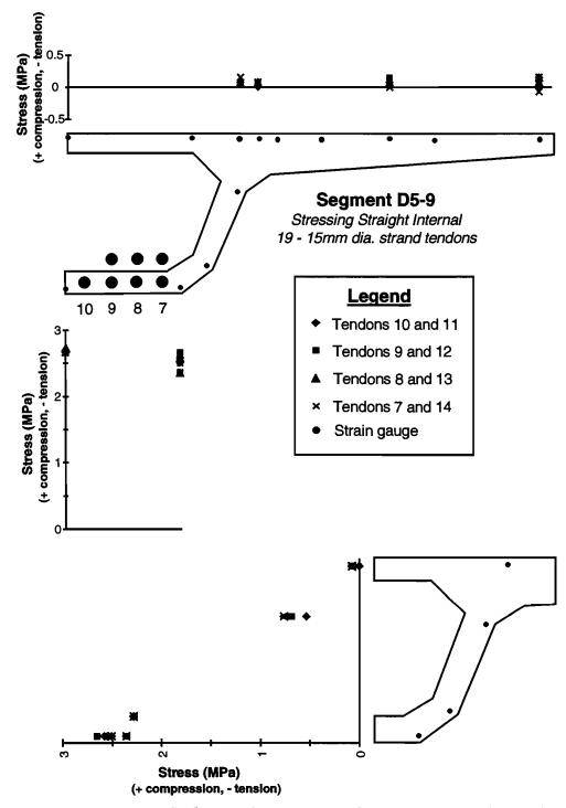
Figure 5.17 Longitudinal stresses in segment D5-9 from the tensioning of internal bottom flange tendons 7 through 14
