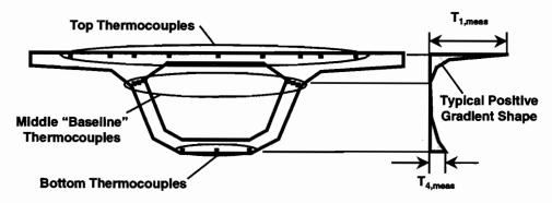
Figure 4.23 Thermocouples used to calculate thermal gradient magnitudes on the Ramp P superstructure
