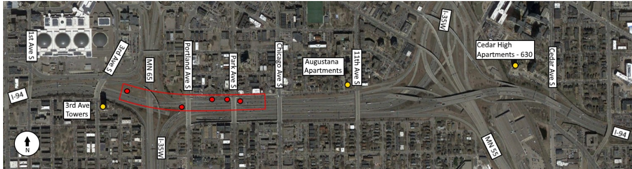
Figure 4-3 Rooftop stations (yellow dots), roadside stations (red dots) and radar coverage (red box). The roadside stations and their radars were installed to supplement the existing I-94 Field Lab equipment.
