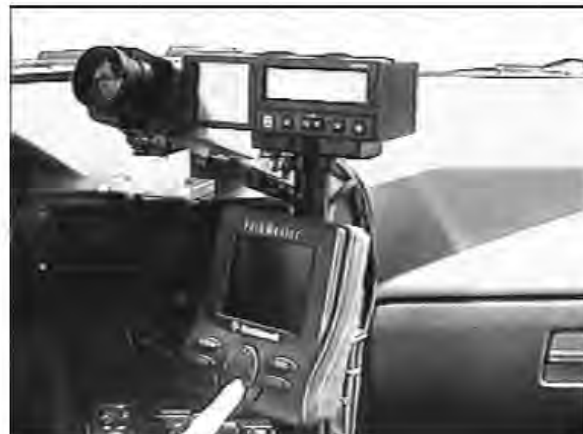
Navigation systems as installed Ali-Scout top, PathMaster bottom
