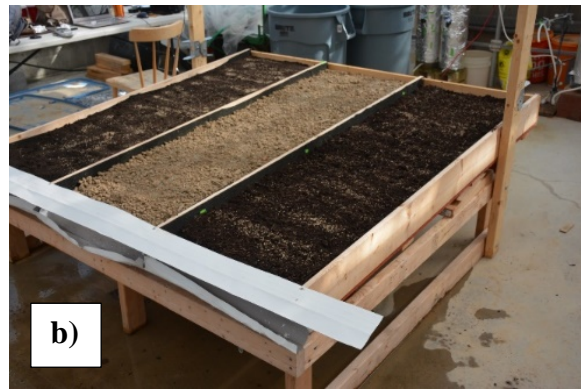
Figure 3-4: (a) Profile of the media and gravel/sand drainage layer at the bottom of the designed platform (b). Runoff is captured in the gutter system for collection and analysis with a rain guard to protect the effluent from dilution due to rainfall.
