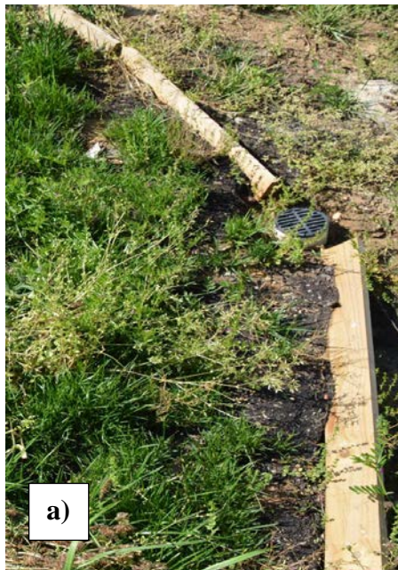
Figure 3-8: a) First flush water runoff sampling container. The weir was added to collect a larger volume of runoff from the slope for testing. b) Cheesecloth sediment bags for soil collection.
