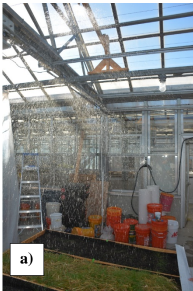
Figure 3-5: Rainfall simulator (a) producing the runoff collected in sample bottles (b).
