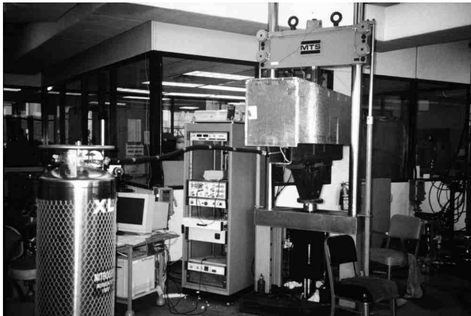
Figure 4. Three-Point Bend Flexure Test Data Acquisition System.
