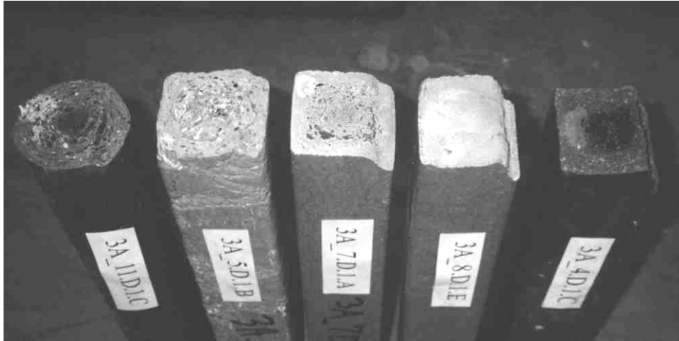
Figure 30. Typical Failure Pattern Observed for Sign Supports after Cantilever Flexure Test.
