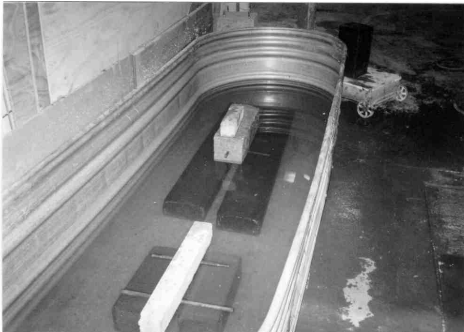
Figure 8. Hydrothermic Cycling Water Process Immersion Setup.
