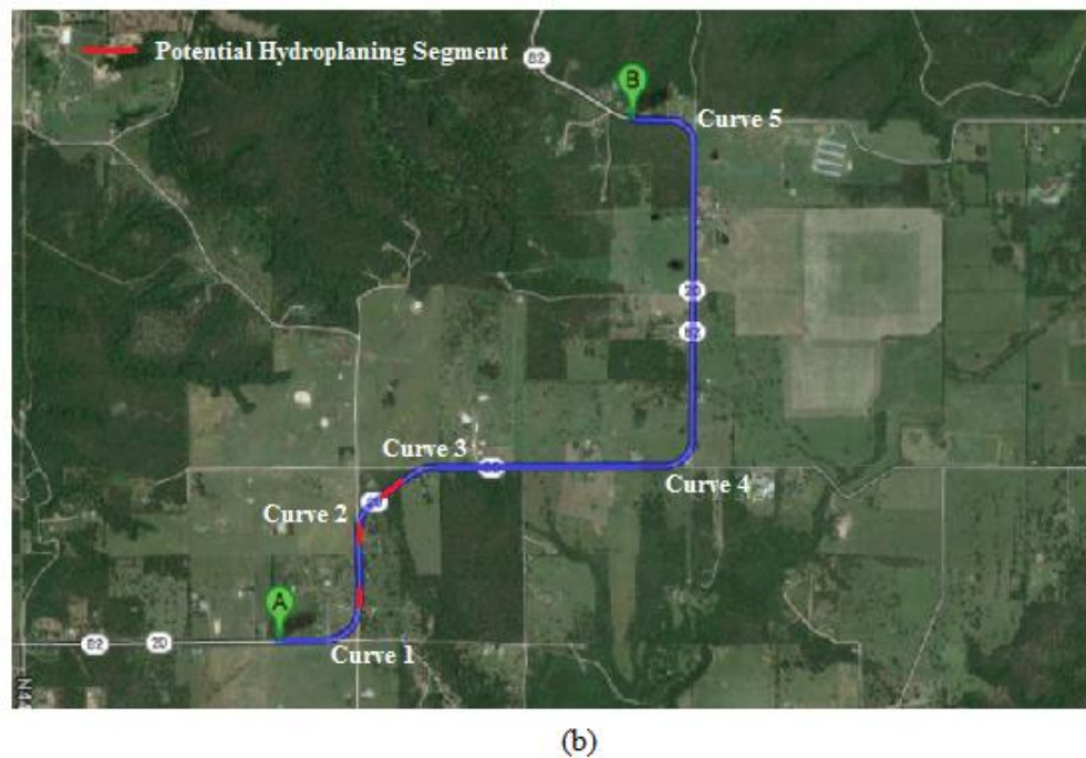
Figure 10 Hydroplaning Test Site: (a) Hydroplaning Speed; (b) Hazardous Segments
