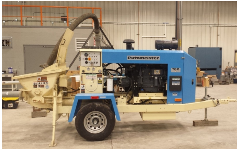
Figure 2 - Putzmeister TK 50 Concrete Pump
