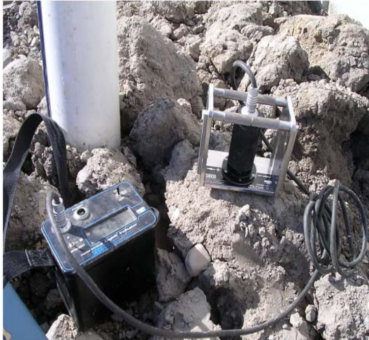
Figure 30: Digi-tilt Sensor and Readout Device (Masada, 2007)
