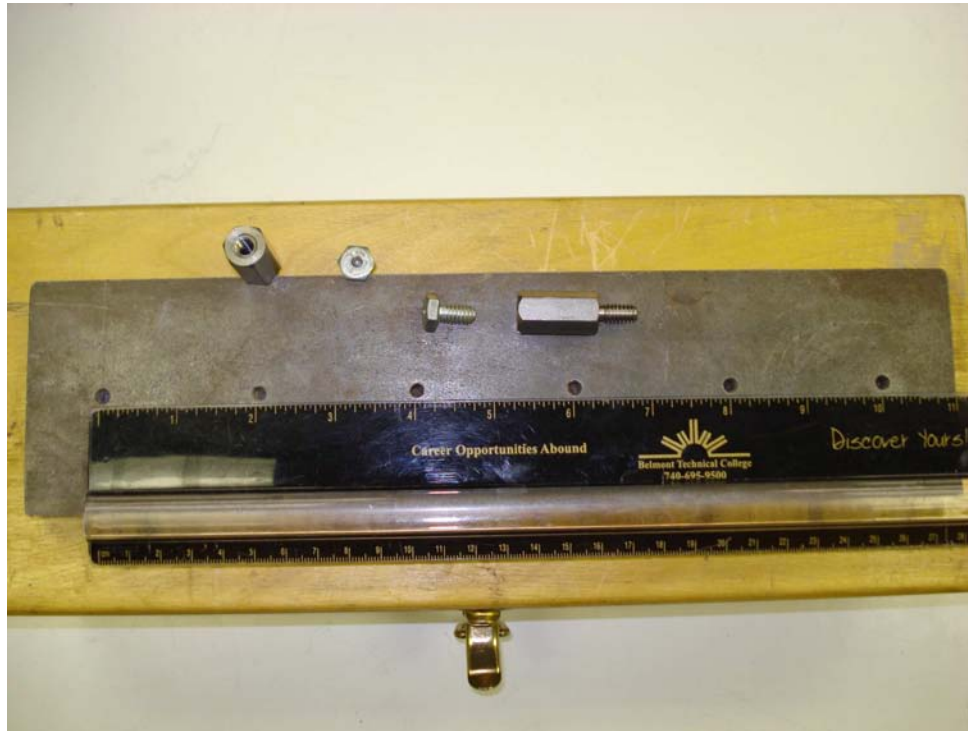
Figure 22: Calibration Plate with Metal Targets
