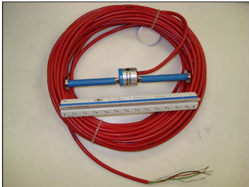
Figure 14: Geokon Model VCE-4200 Vibrating Wire Strain Gage
