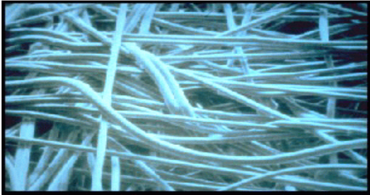
Micrograph of a Needle-Punched Non-Woven Geotextile
