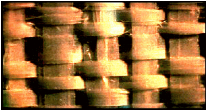
Micrograph of a Slit-film Woven Geotextile
