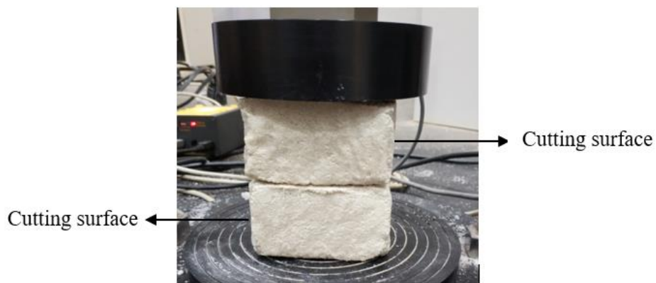
Figure 2-19. Brick compressive testing system for stacked two halves
