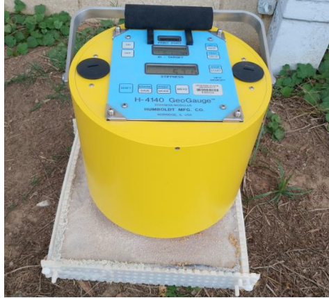
Figure 2-16. Photograph of Humboldt GeoGauge.
