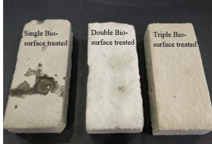
Figure 3-9. Surfaces of single, double, and triple bio-surface treated cement-treated samples after accelerated erosion
