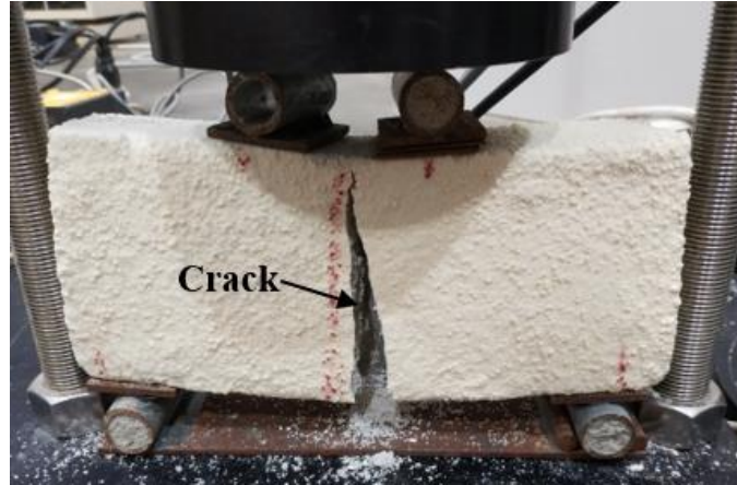
Figure 2-20. Four point bending testing system
