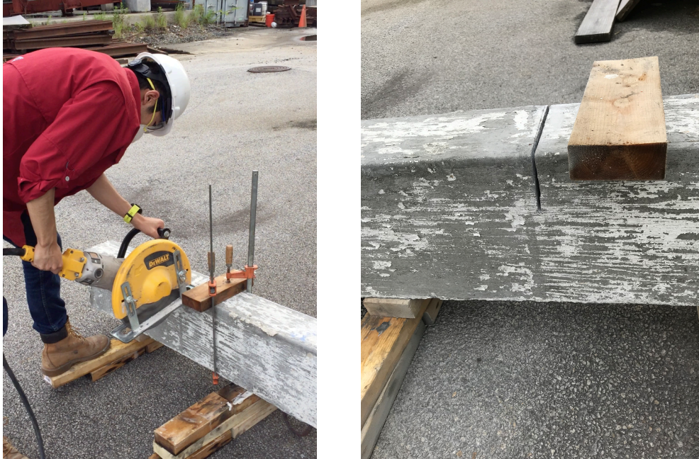
Figure 30. Notching of concrete beams with masonry saw.
