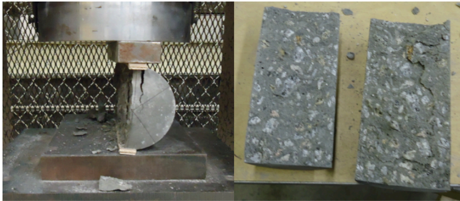
Figure 1. Undesired tensile splitting failure of initial 4 inch x 8 inch plain concrete specimen.
