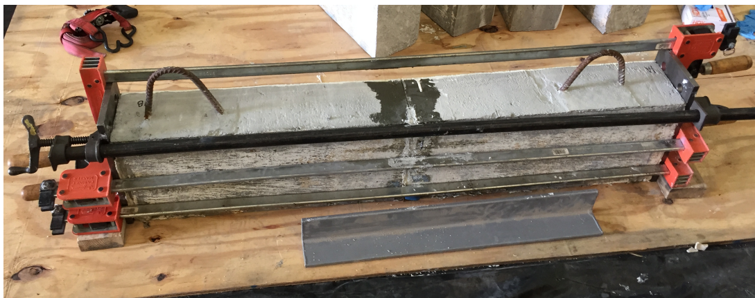
Figure 33. Preparation of epoxy-repaired beam: repaired beam clamped together for curing.
