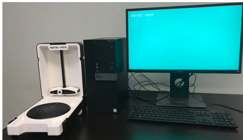
Figure 3. Matter and Form 3D Tabletop Scanner used for developing realistic aggregate models.
