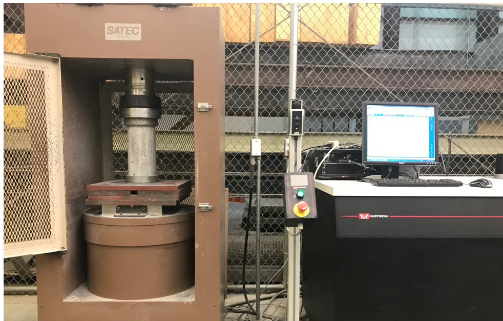
Figure 5. Uniaxial compression setup as outlined in ASTM C39.
