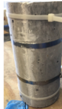
Figure 15. Preparation of epoxy-repaired cylindrical specimen prior to inclusion of epoxy.
