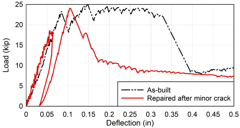
Figure 45. Load-deflection behavior of reinforced concrete beam repaired after minor cracks compared to as-built beam.
