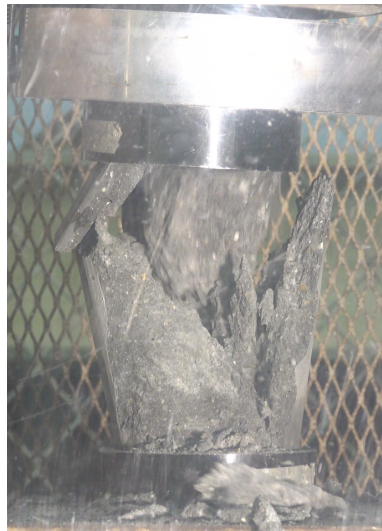
Figure 25. Typical failure pattern of a mortar specimen.
