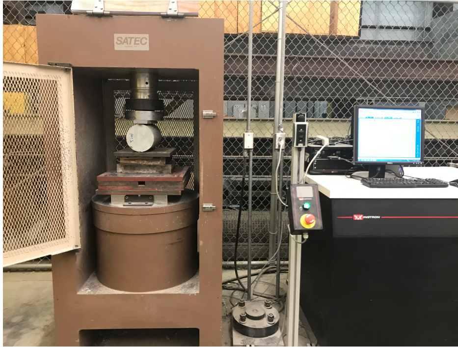
Figure 11. Splitting tension experimental setup.
