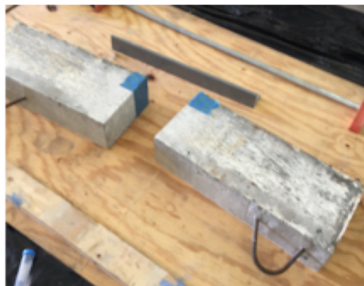
Figure 31. Preparation of epoxy-repaired beam: beam cut in half with masonry saw.
