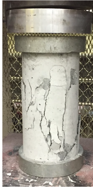
Figure 9. Typical plain concrete behavior indicative of a type 3 columnar failure.
