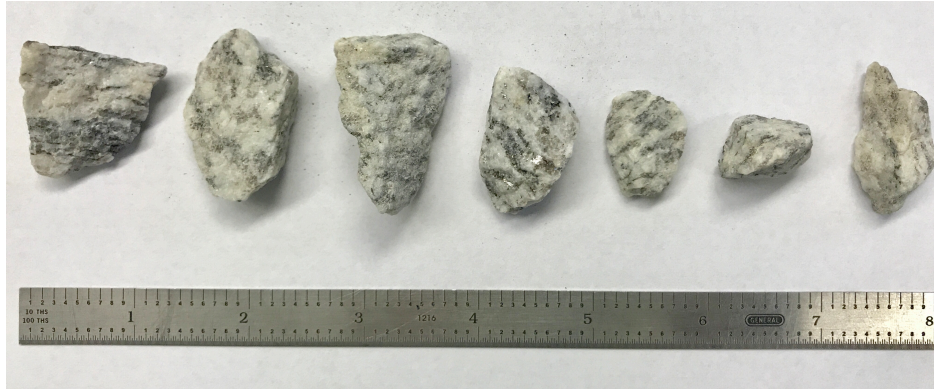
Figure 2. Granite-Gneiss aggregate used in concrete cylinder mix.
