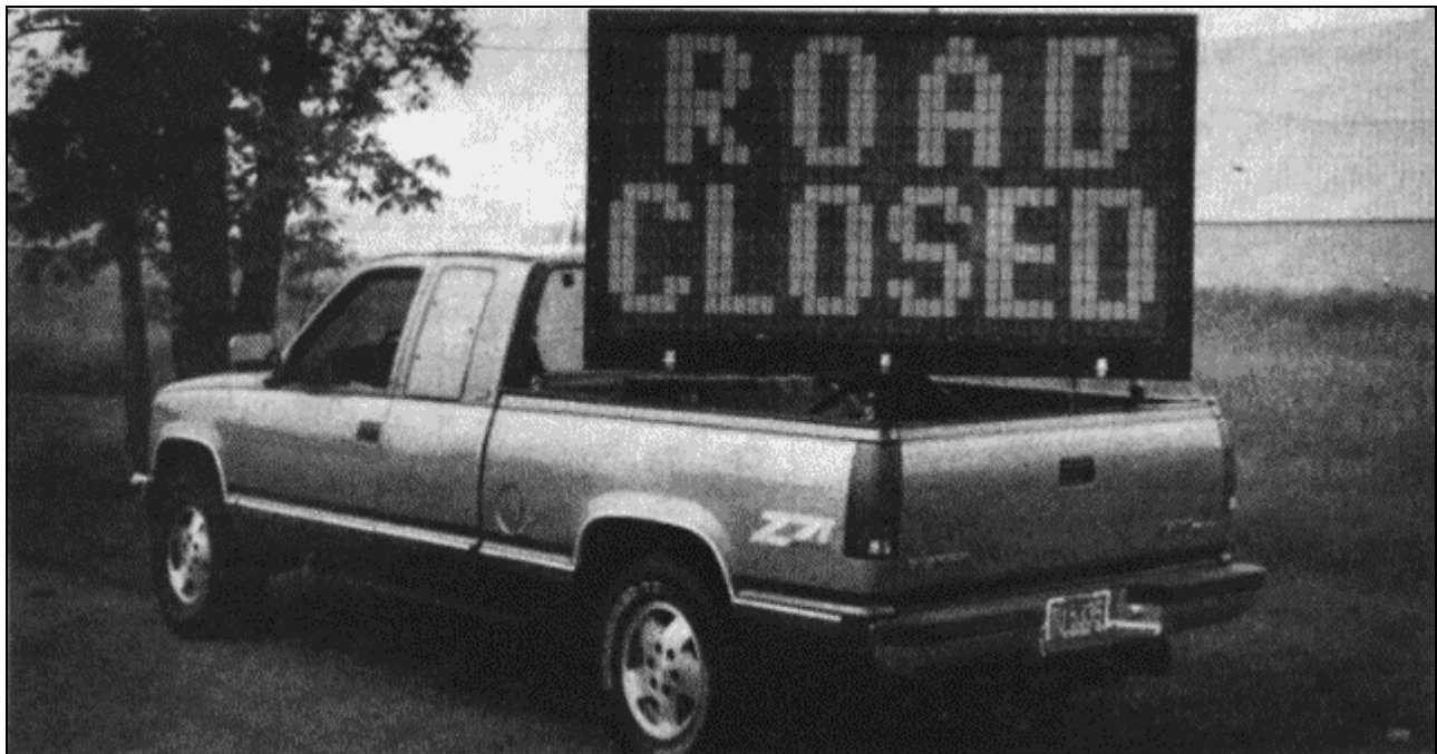
Figure 10-18. Major incident response units with portable CMS.
