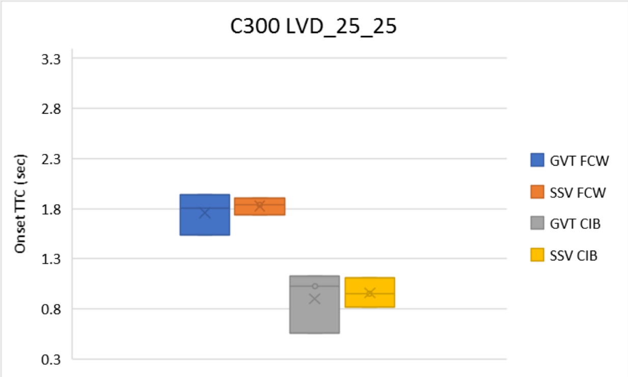
Figure B-10: FCW and CIB onset timings to both targets during LVD_25_25 scenario (Mercedes C300).
