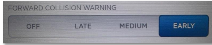
Figure 5: Tesla Model S FCW settings. The “earlier” setting was selected for all tests described in this report.
