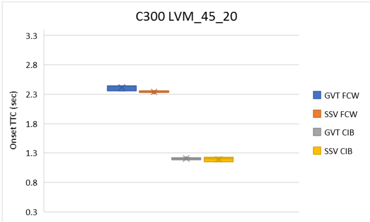
Figure B-15: FCW and CIB onset timings to both targets during LVM_45_20 scenario (Mercedes C300).
