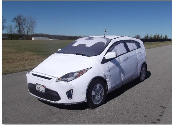
Figure 3: GVT (revision E) atop of the LPRV.
