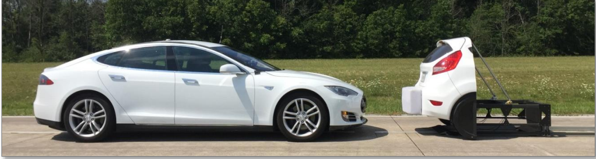
Figure 1: NHTSA's SSV (right) shown with the Tesla Model S evaluated in this study (left).
