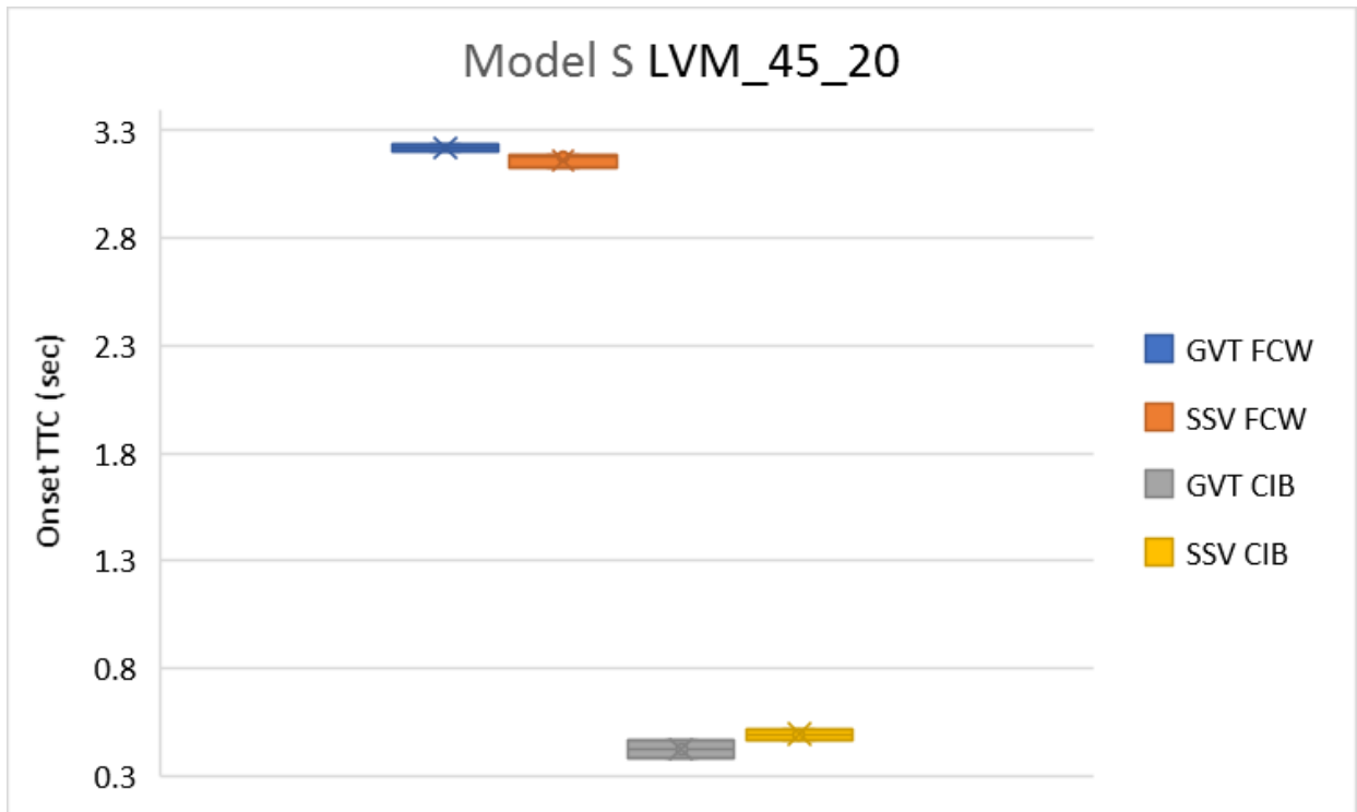
Figure B-24: FCW and CIB onset timings to both targets during LVM_45_20 scenario (Tesla Model S).
