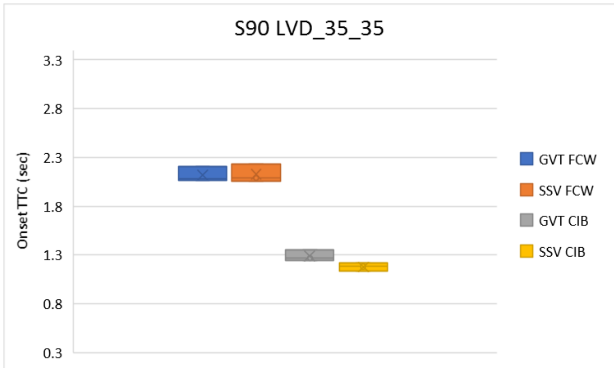
Figure B-2: FCW and CIB onset timings to both targets during LVD_35_35 scenario (Volvo S90).
