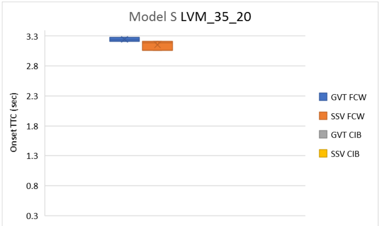
Figure B-23: FCW and CIB onset timings to both targets during LVM_35_20 scenario (Tesla Model S).
