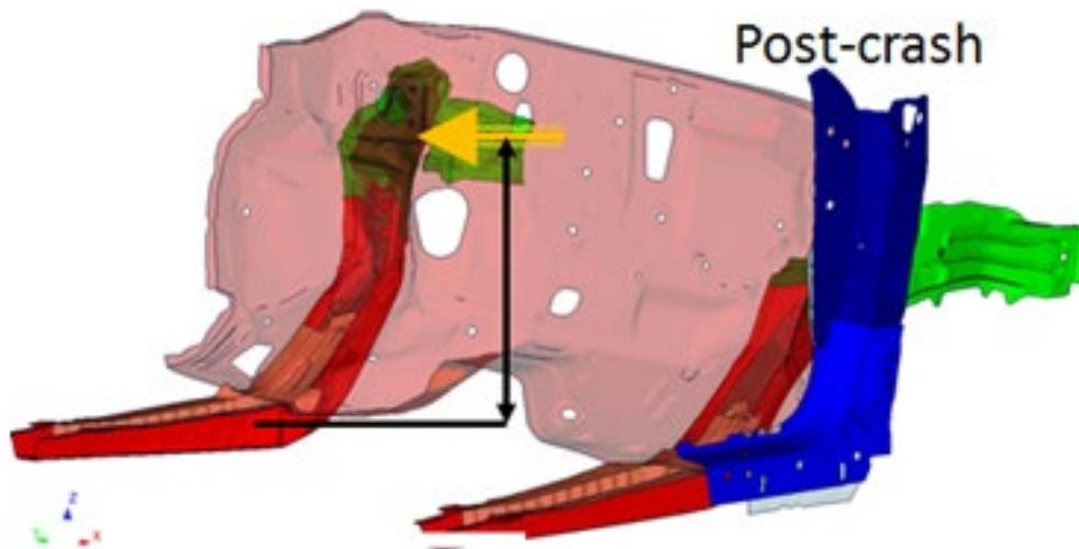
Figure 23(b) - Firewall in Left Oblique Impact Post-Crash
