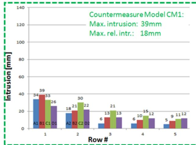
Figure 28(c) - Left Oblique Toe Pan Intrusion CM1
