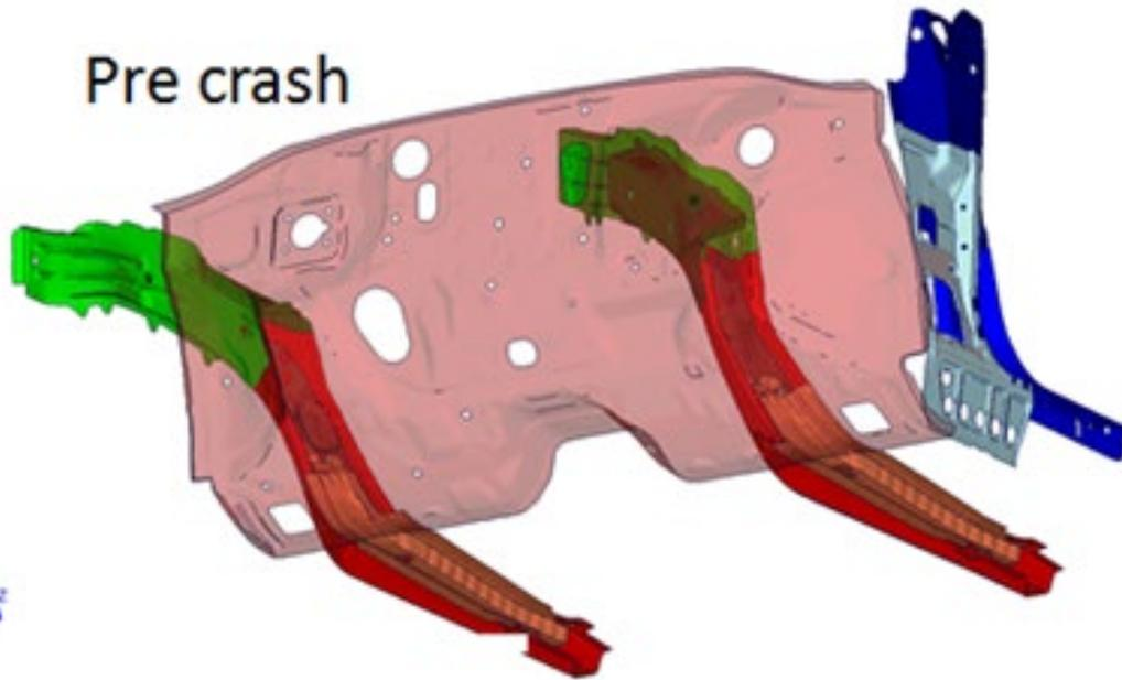
Figure 24(a) - Firewall and Mid-Rail in Right Oblique Impact Pre-Crash
