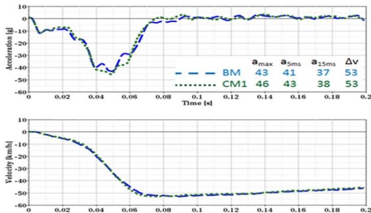
Figure 29(c) - CM1 Left Oblique Vehicle Pulse
