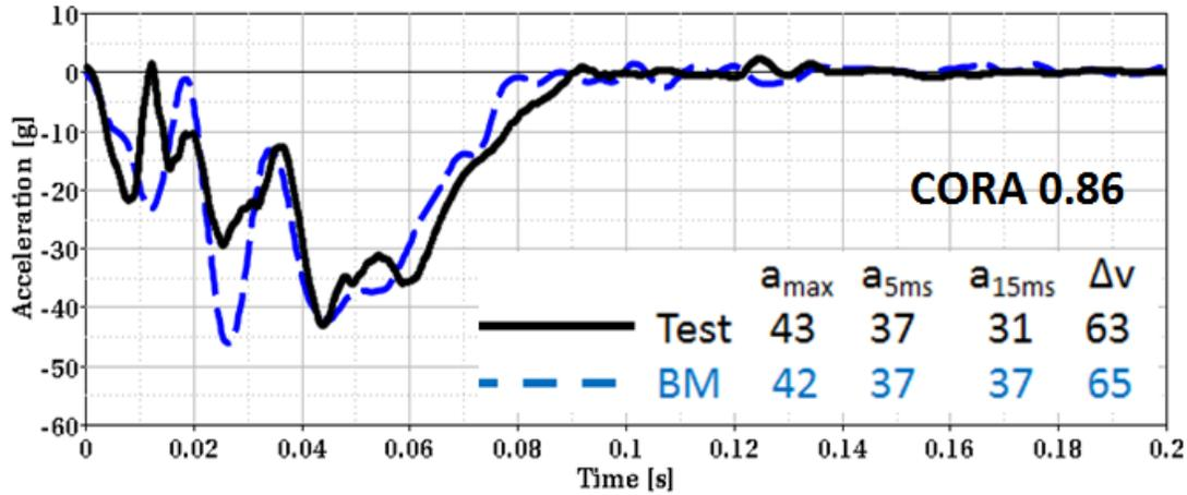
Figure 18(a) - 2015 NCAP Test Versus Simulation - Acceleration Pulse
