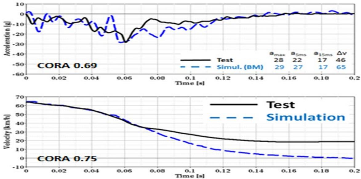
Figure 15(b) - IIHS SO Test Versus Simulation – Vehicle Pulse
