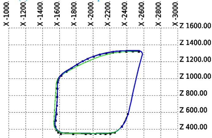
Figure 10 (b) - 2015 Left Oblique Test Versus Simulation – Door Sill
