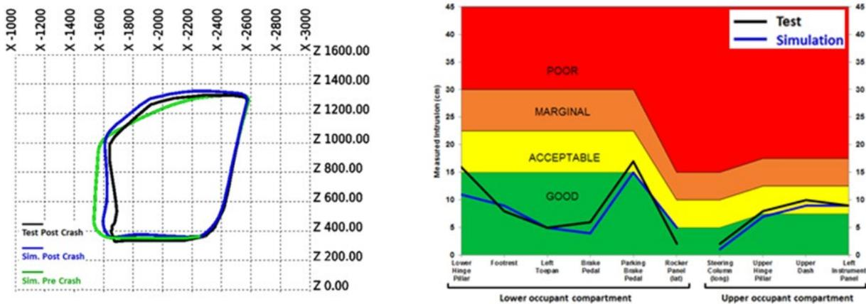
Figure 14 - IIHS SO - (b) Door Sill (c) Intrusion
