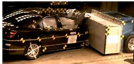
Figure 12(a) - Right Oblique Test Versus Simulation - Overall
