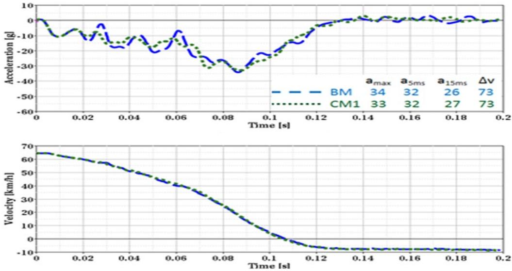
Figure 33(c) - CM1- IIHS MO Vehicle Pulse
