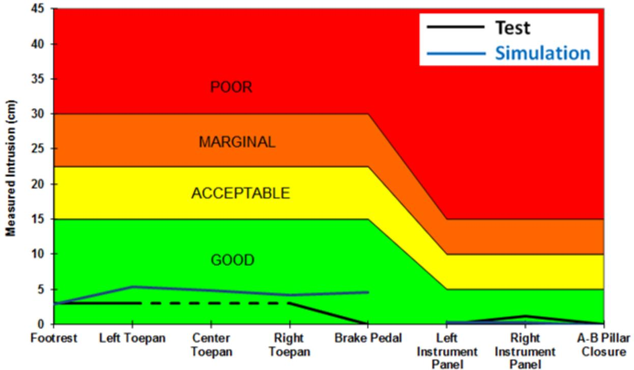
Figure 17(b) - NCAP Test Versus Simulation - Intrusion Chart
