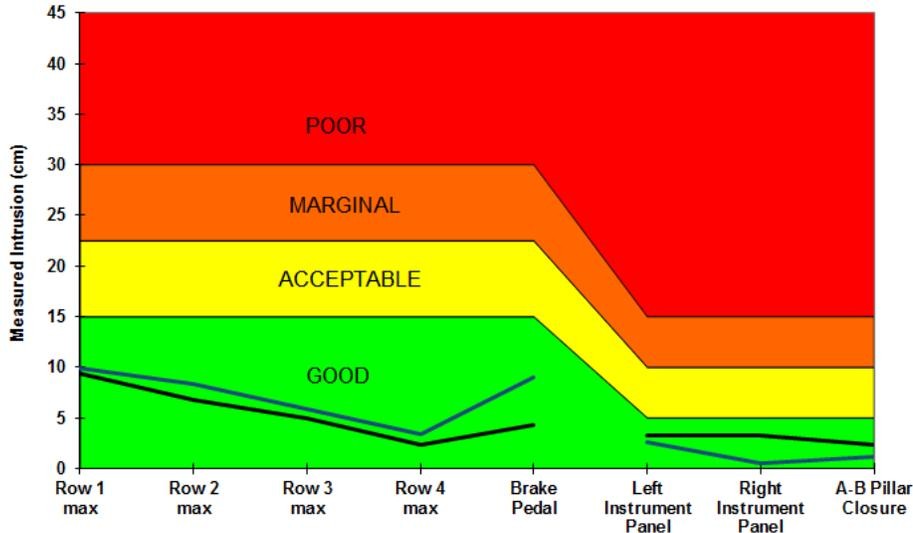
Figure 10 (c) - 2015 Left Oblique Test Versus Simulation - Intrusion
