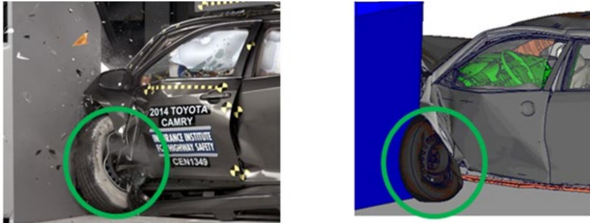
Figure 14(a) - IIHS SO - Overall Test and Simulation
