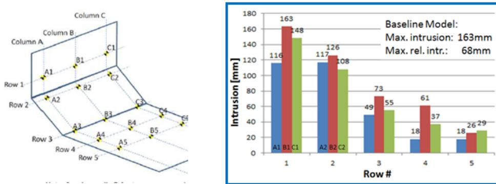
Figure 46 - Right Oblique Toe Pan Intrusion (a) Measurement Points, (b) BM
