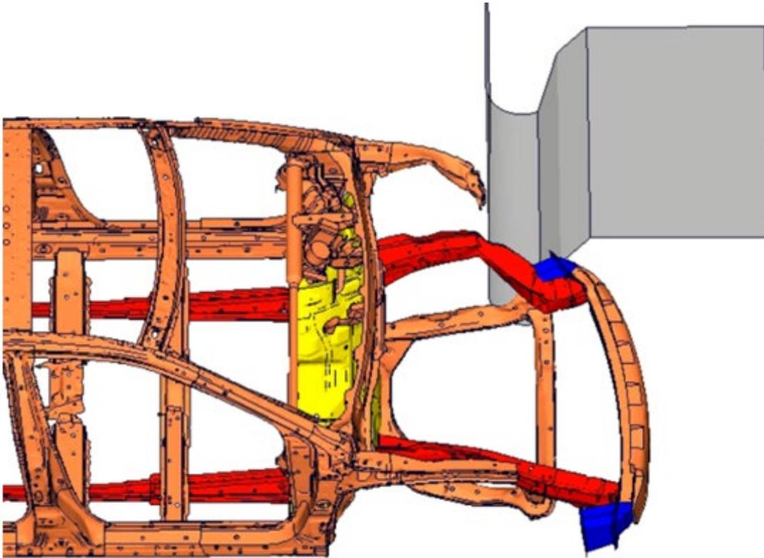
Figure 15(a) - IIHS SO Test Versus Simulation - FE Model BIW
