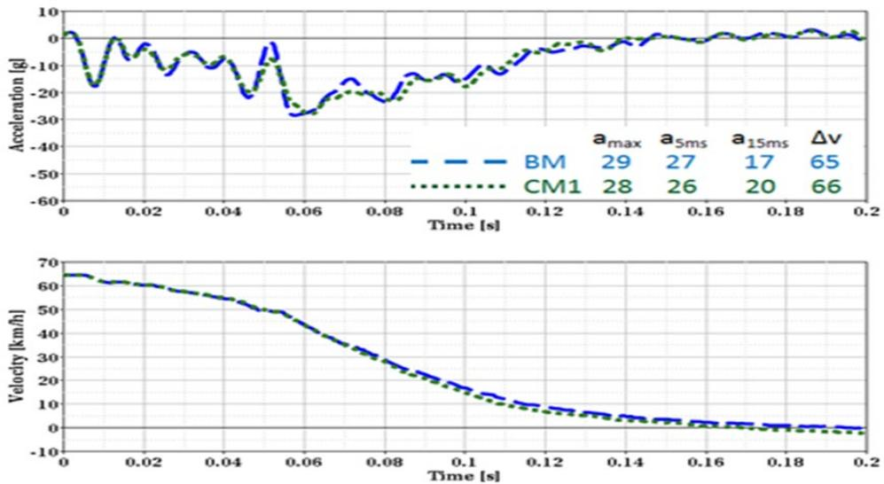
Figure 32(c) - CM1- IIHS SO Vehicle Pulse
