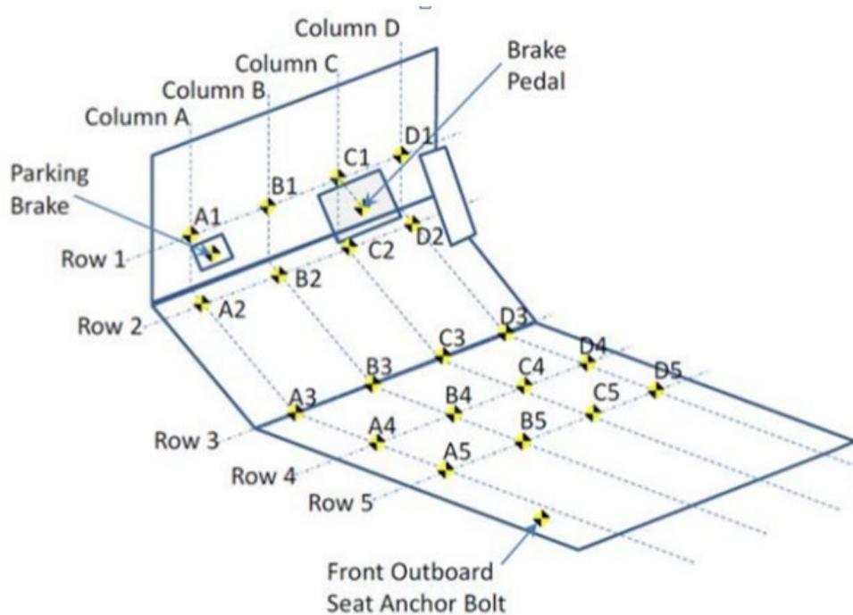
Figure 5 - (c) Oblique Toe-Pan Intrusion Measurement Points
