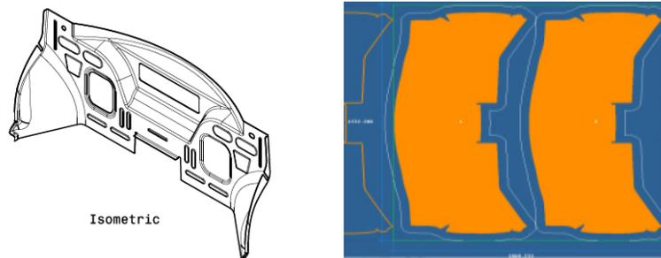
Figure 8 - Example Part (a) CAD Design and (b) Untrimmed Blank
