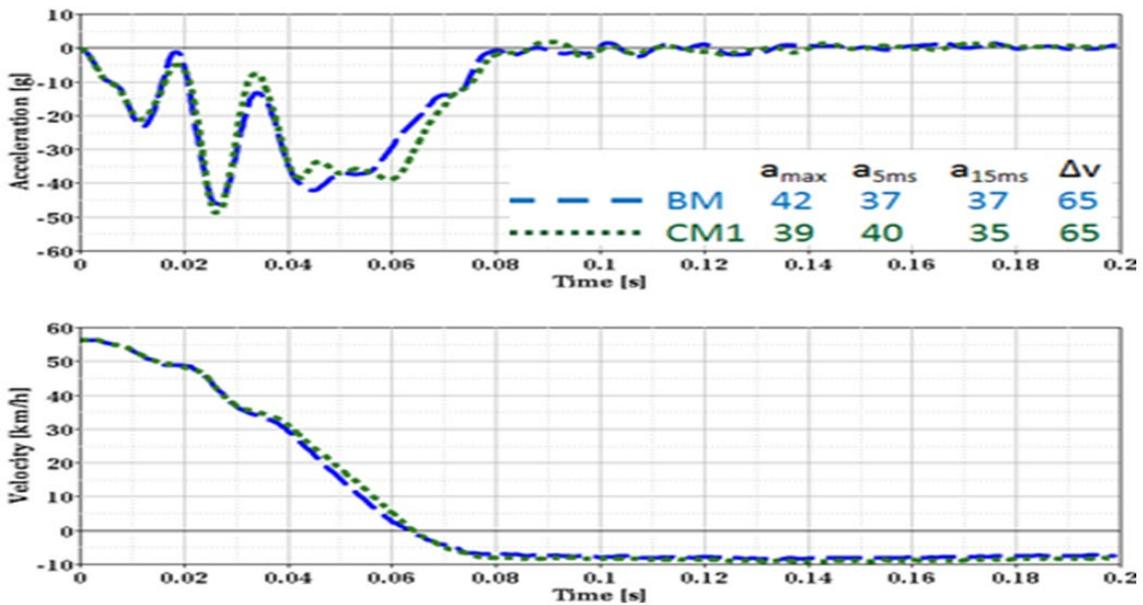
Figure 34(c) - CM1- NCAP Vehicle Pulse
