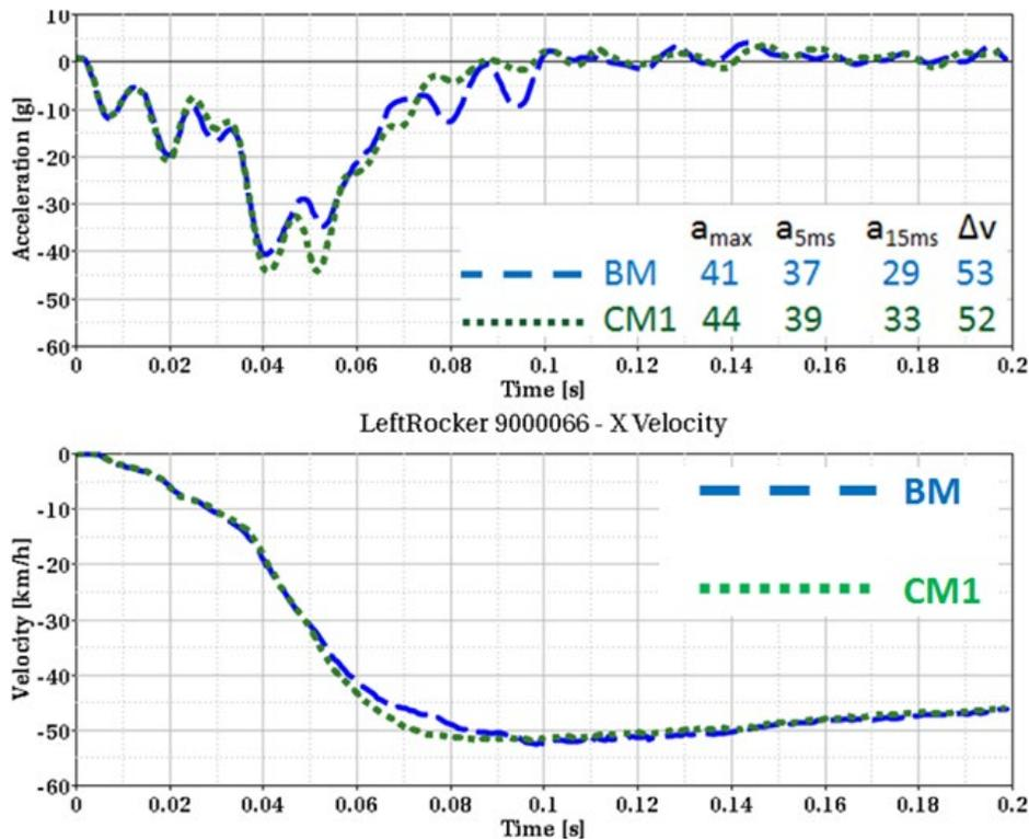
Thus, CM1 fulfills all design goals defined in Chapter 5 for the right oblique impact configuration. The absolute maximum intrusion was reduced from 163 mm to 78 mm, which is equivalent to a 52 percent reduction.
