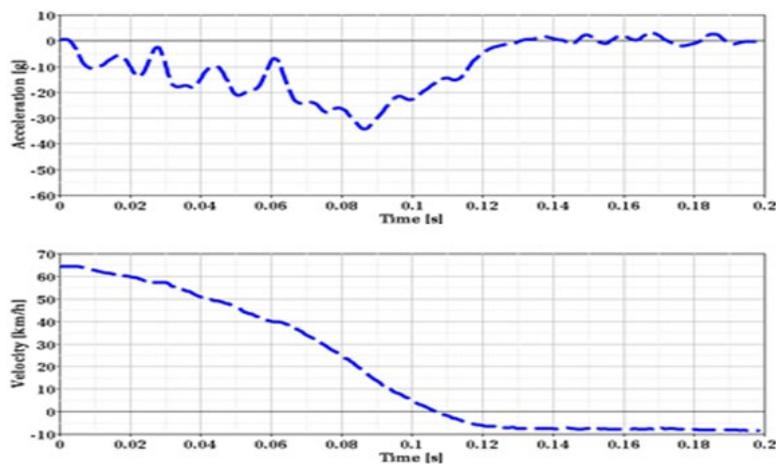
Figure 16(c) – MO Vehicle Pulse
