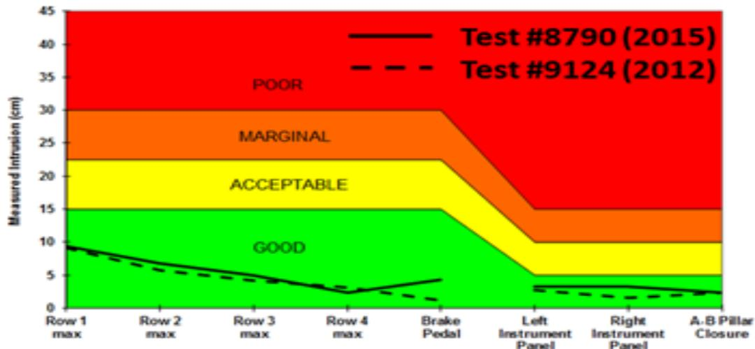
Figure 9 (b)- 2012 & 2015 Left Oblique Test Results – Intrusion
