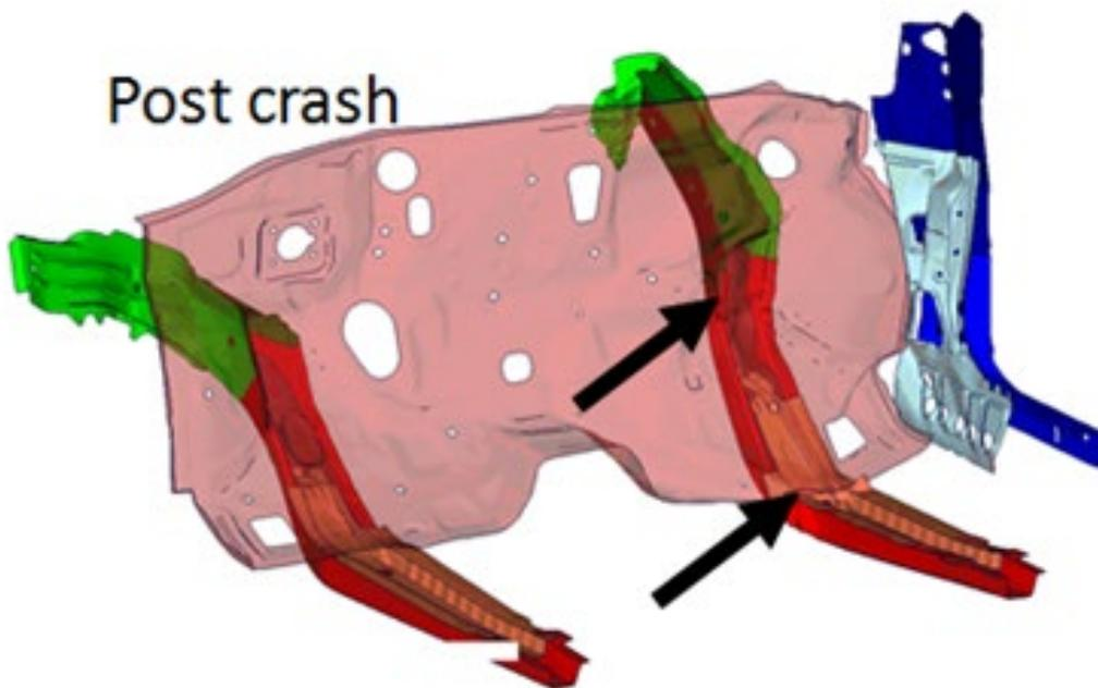
Figure 24(b) - Firewall and Mid-Rail in Right Oblique Impact Post-Crash
