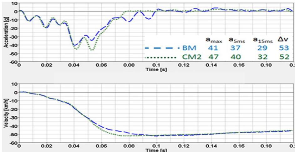
Figure 39(c) - CM2 Right Oblique Vehicle Pulse
