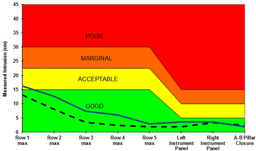
Figure 12(a) - Right Oblique Test Versus Simulation - Intrusion
