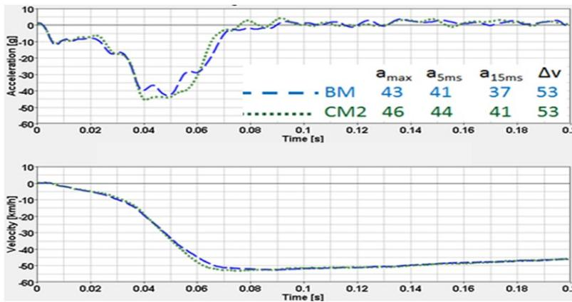
Figure 37(c) - CM2 Left Oblique Vehicle Pulse
