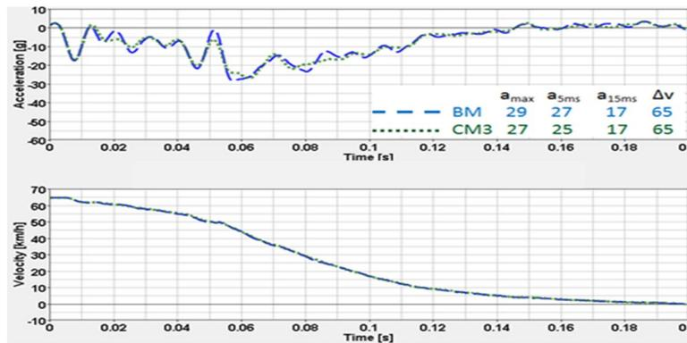
Figure 48 - CM3 IIHS SO (a) Intrusion (b) Door Sill (c) Vehicle Pulse
