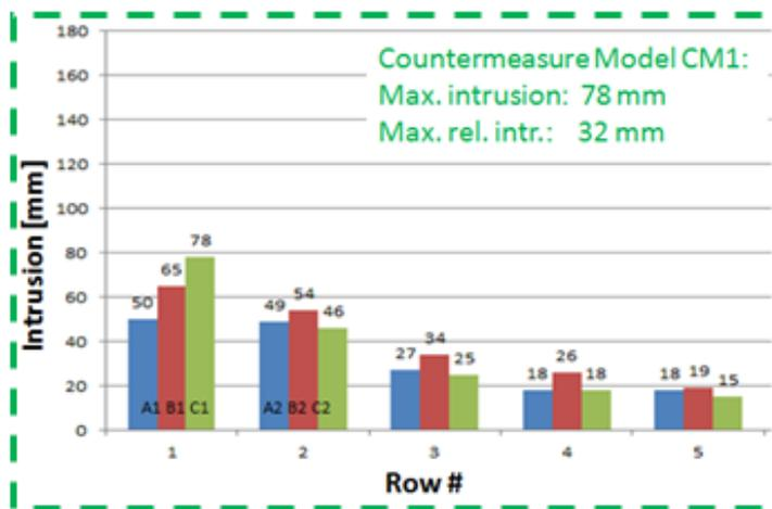
Figure 30(c) - Right Oblique Toe Pan Intrusion CM1
