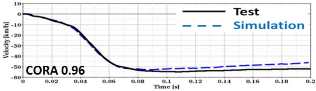
Figure 11(a) - 2015 Left Oblique Test Versus Simulation - Vehicle Pulse
