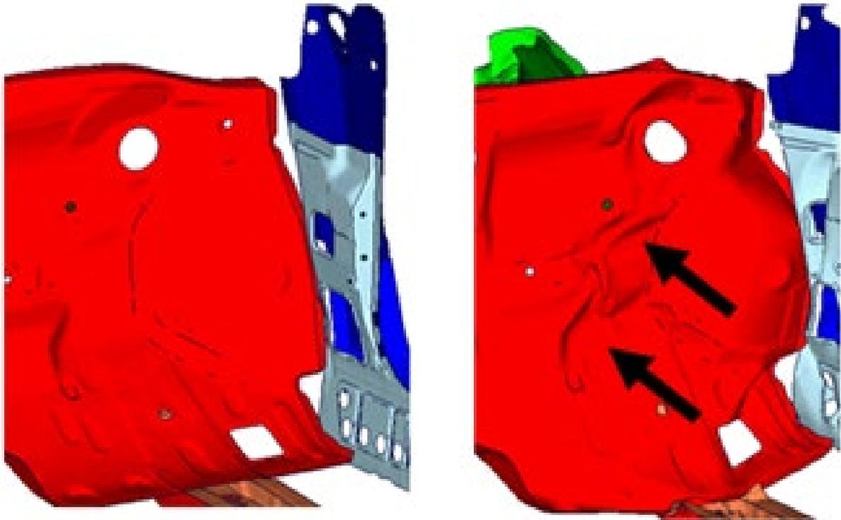
Figure 22(b) – Firewall in Passenger Side Oblique Impact
