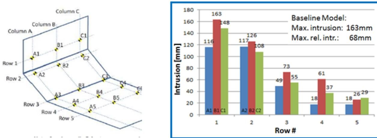
Figure 30 - Right Oblique Toe Pan Intrusion (a) Measurement Points, (b) BM
