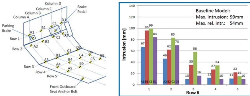
Figure 44 - Left Oblique Toe-Pan Intrusion (a) Measurement Points (b) BM
