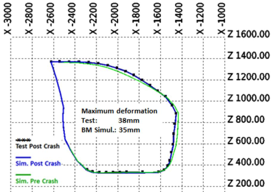
Figure 12(b) - Right Oblique Test Versus Simulation - Door Sill Deformation
