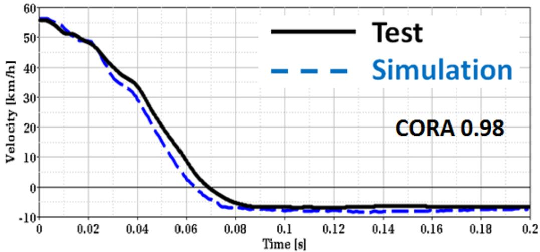
Figure 18(b) - 2015 NCAP Test Versus Simulation - Velocity Pulse
