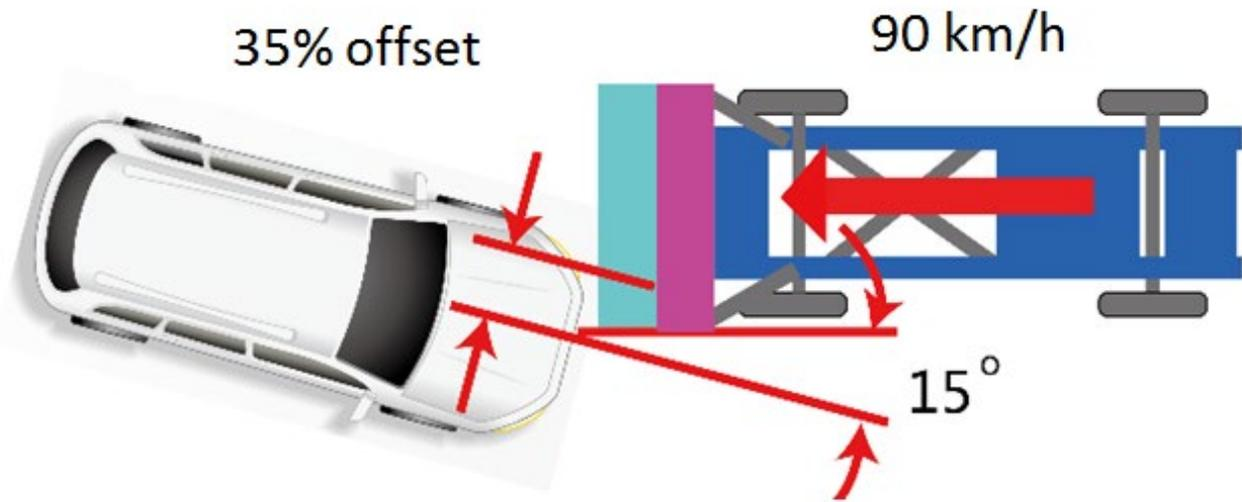
Figure 1 - Frontal Oblique Test Configuration
