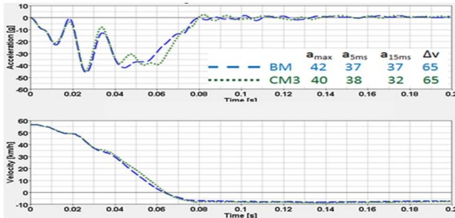
Figure 50(c) - CM3 NCAP Vehicle Pulse
