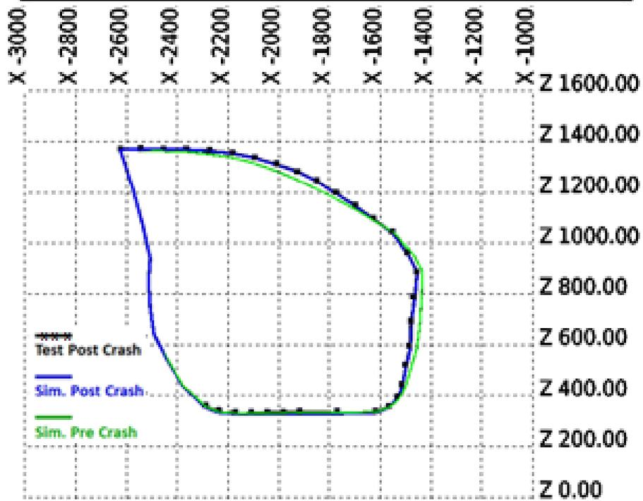
Figure 21(b) - Door Sill Deformation for Passenger Side
