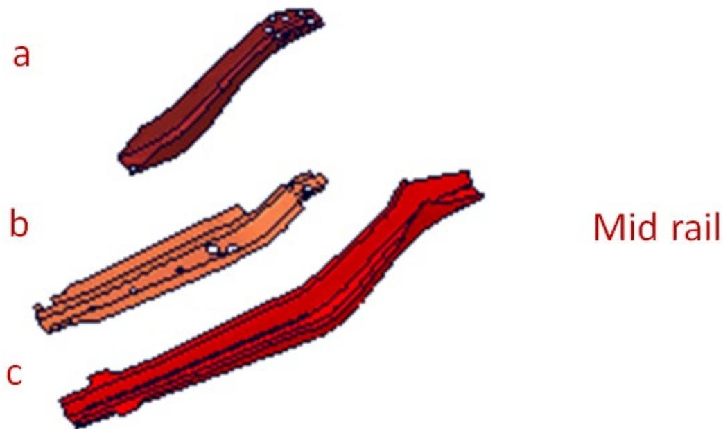
Figure 35(b) - CM2 Exploded View Mid-Rail Components
