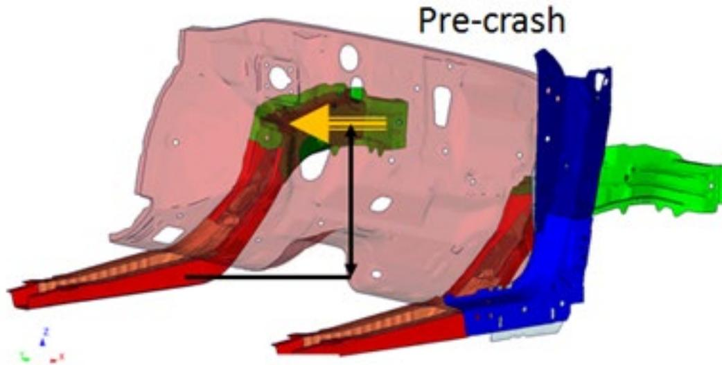
Figure 23(a) - Firewall in Left Oblique Impact Pre-Crash
