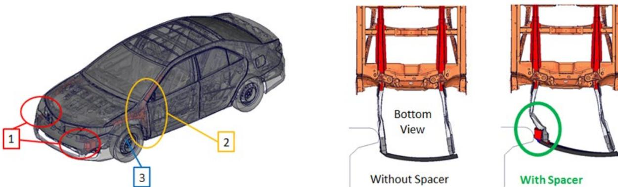
Figure 4 - (a) 2015 Toyota Camry FE model (b) Effect of spacer in IIHS small overlap
