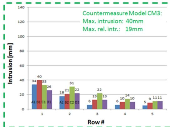
Figure 44(c) - Left Oblique Toe-Pan Intrusion CM3
