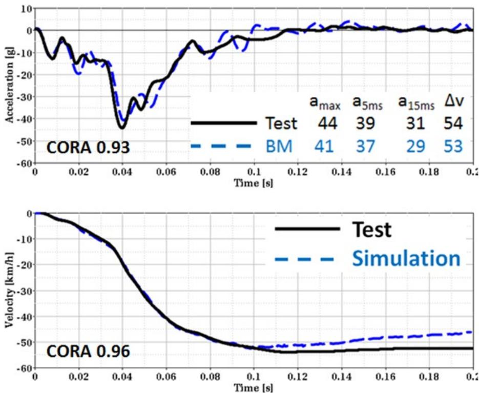
Figure 13(a) - Right Oblique Test Versus Simulation - Vehicle Pulse
