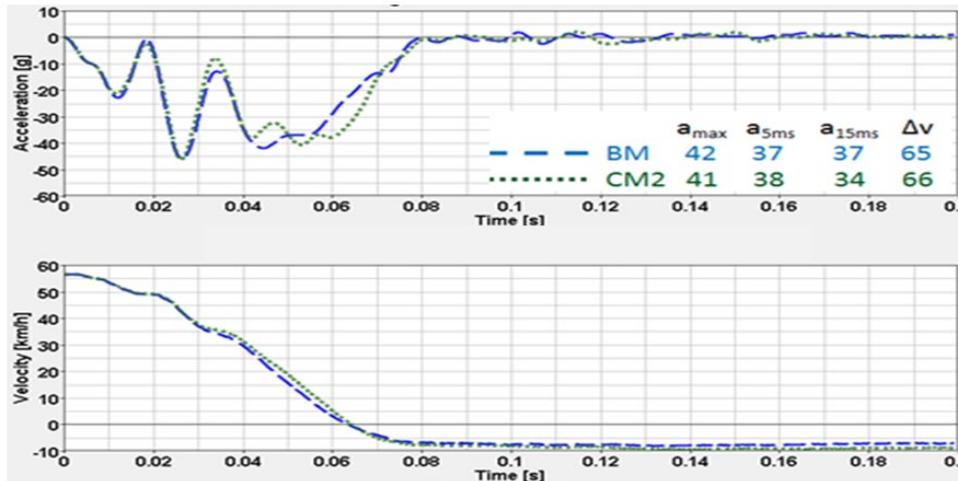
Figure 42(c) - CM2 NCAP Vehicle Pulse
