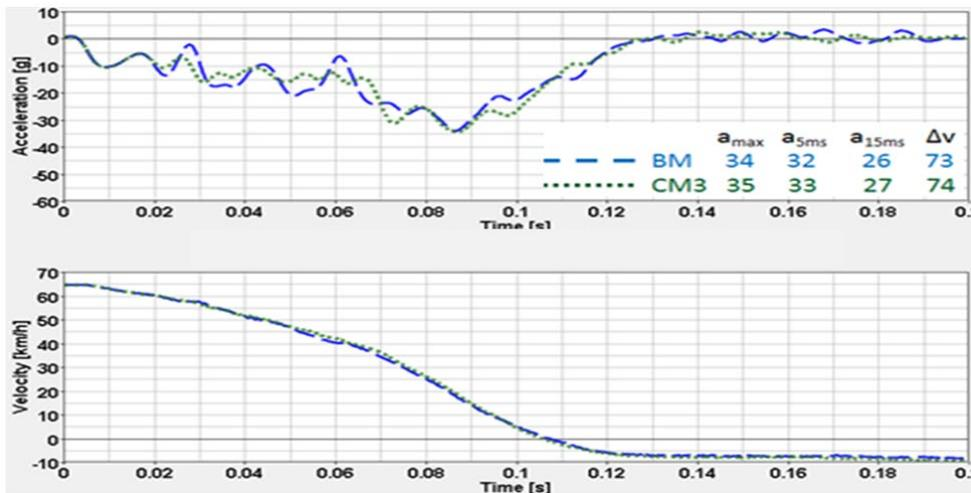
Figure 49(c) - CM3 IIHS MO Vehicle Pulse
