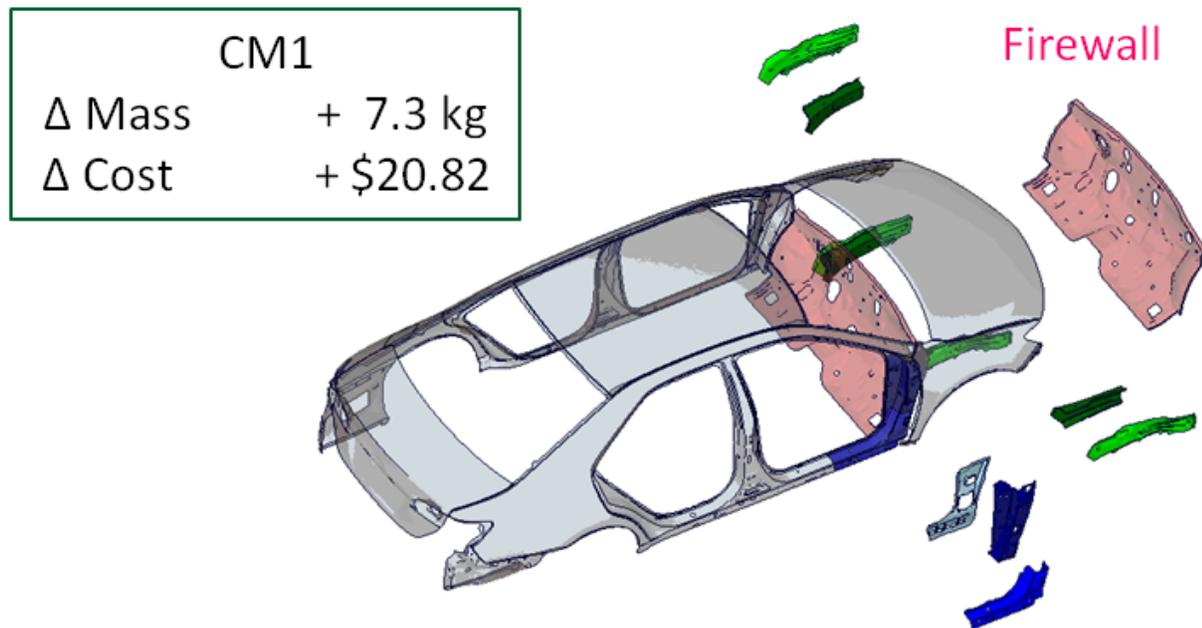
Figure 27(a) - CM1 Exploded View Overall, (b) Right Hinge Pillar, (c) Frontal Rail Parts
