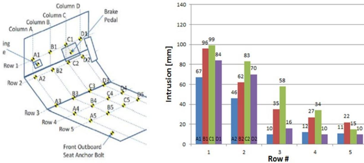
Figure 19(a) - BM Toe-Pan Intrusion Measurements for Left Oblique Impact
