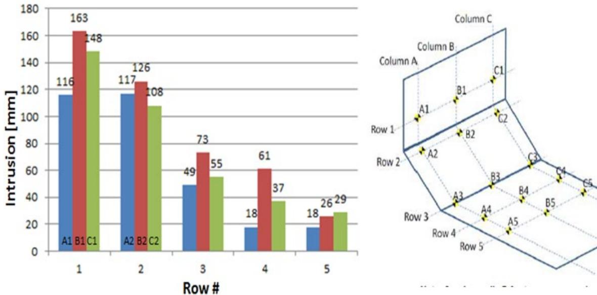
Figure 19(b) - BM Toe-Pan Intrusion Measurements for Right Oblique Impact
