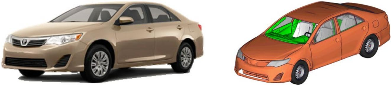
Figure 2 - 2012 Toyota Camry (a) Physical Vehicle and (b) FE Model
