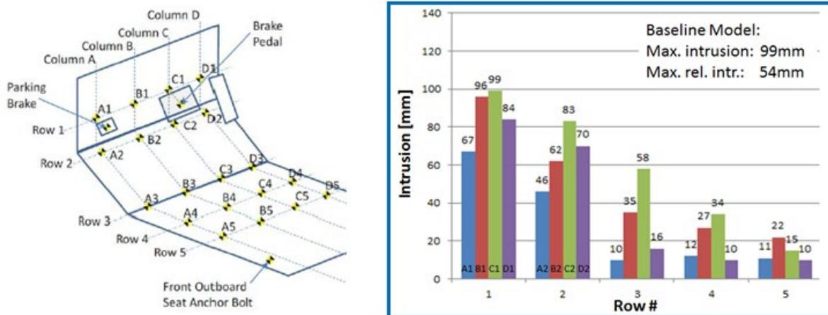
Figure 36 - Left Oblique Toe-Pan Intrusion (a) Measurement Points, (b) BM
