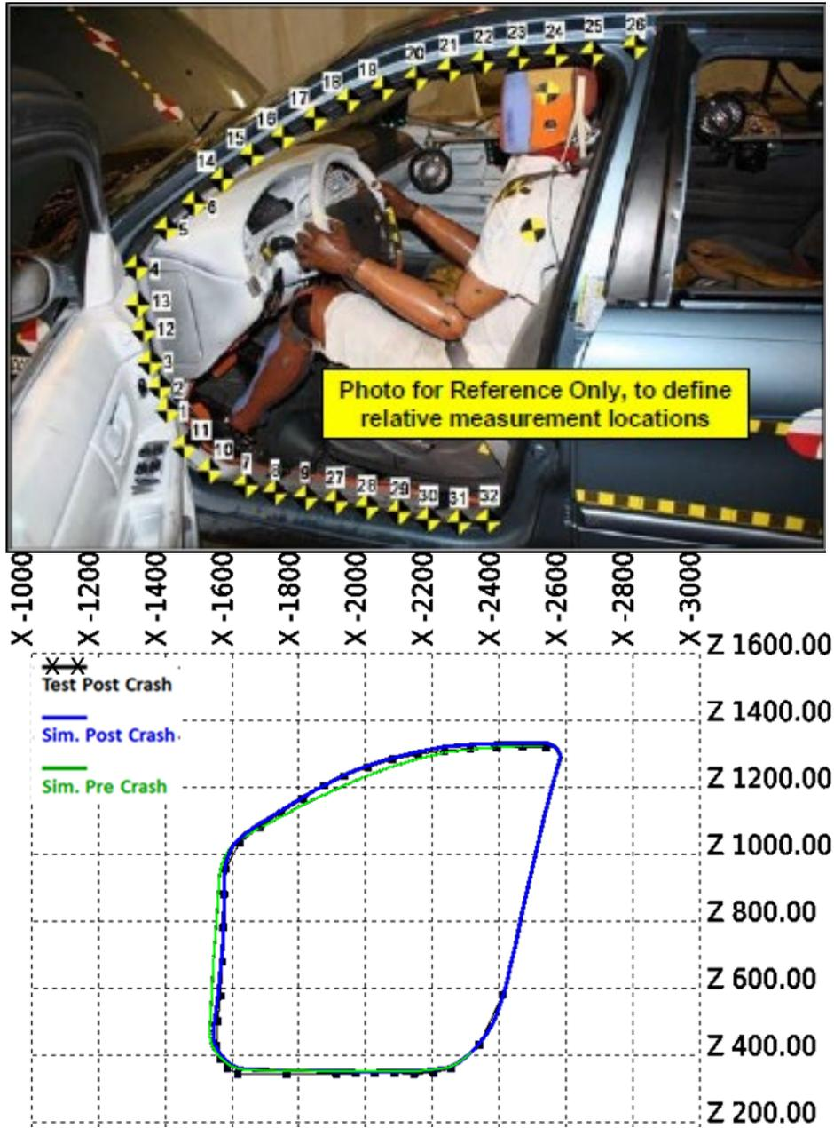
Figure 21(a) - Door Sill Deformation for Driver Side
