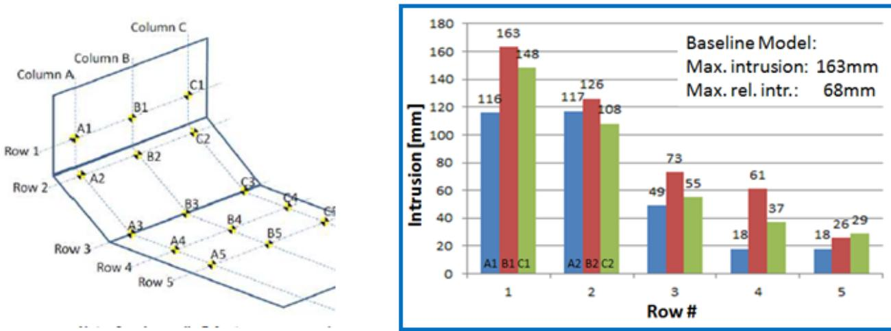
Figure 38 - CM2 Right Oblique Toe Pan Intrusion (a) Measurement Points, (b) BM
