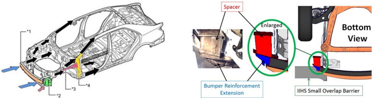
Figure 3 - 2015 Toyota Camry Design Changes (a) Overall Schematic, (b) “Spacer”
