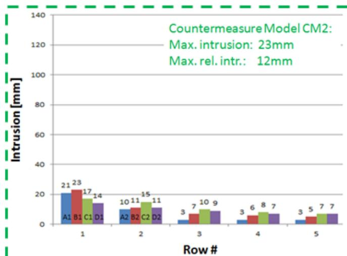
Figure 36(c) - Left Oblique Toe-Pan Intrusion CM2
