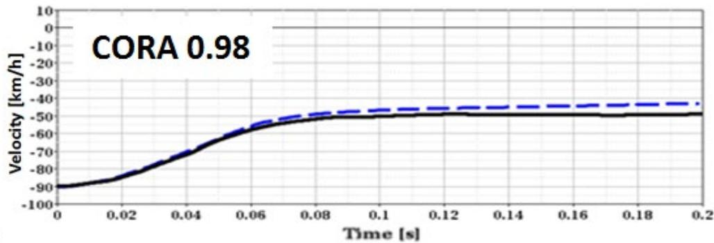
Figure 11(b) - 2015 Left Oblique Test Versus Simulation - Barrier Pulse
