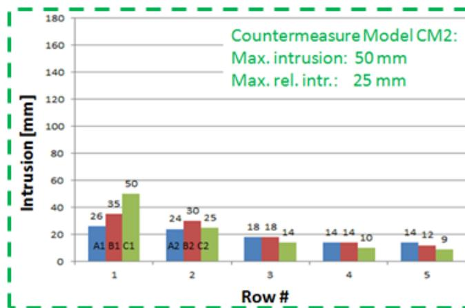
Figure 38(c) - CM2 Right Oblique Toe Pan Intrusion CM2
