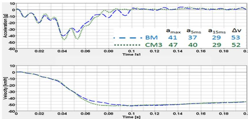
Figure 47(c) - Right Oblique Vehicle Pulse
