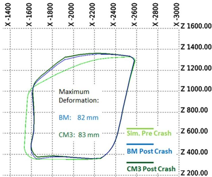
Figure 48 - CM3 IIHS SO (a) Intrusion (b) Door Sill (c) Vehicle Pulse
