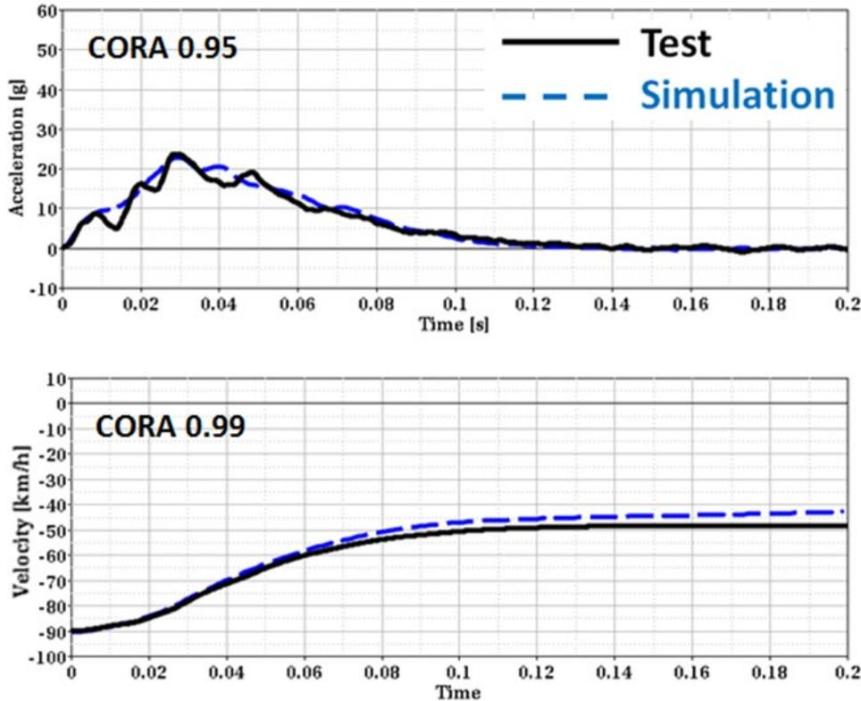
Figure 13(b) - Right Oblique Test Versus Simulation - Barrier Pulse
