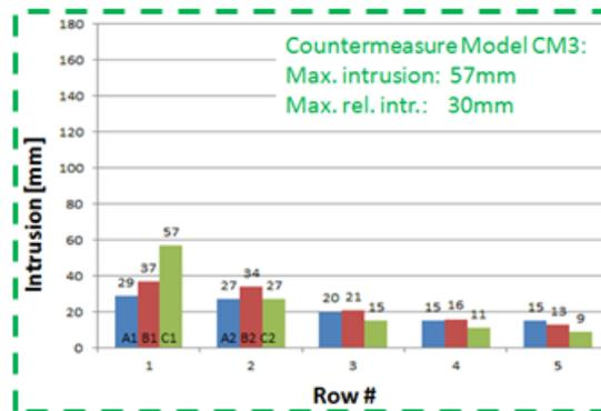
Figure 46(c) - Right Oblique Toe Pan Intrusion CM3
