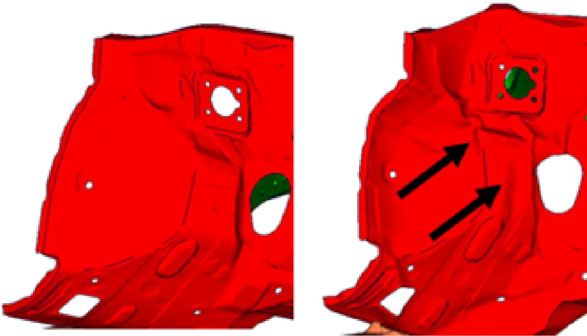
Figure 22(a) - Firewall in Driver-Side Oblique Impact
