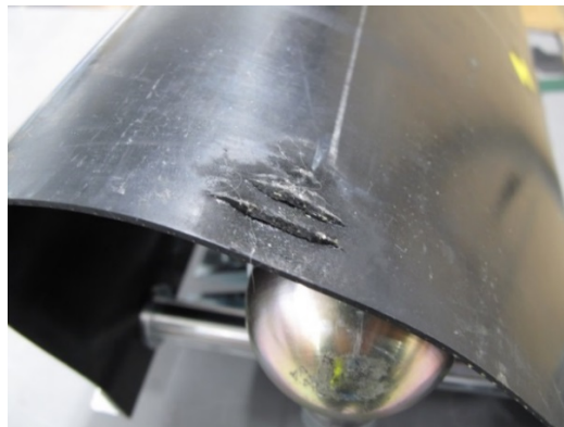
Figure 42. Minor damage to upper legform impactor
