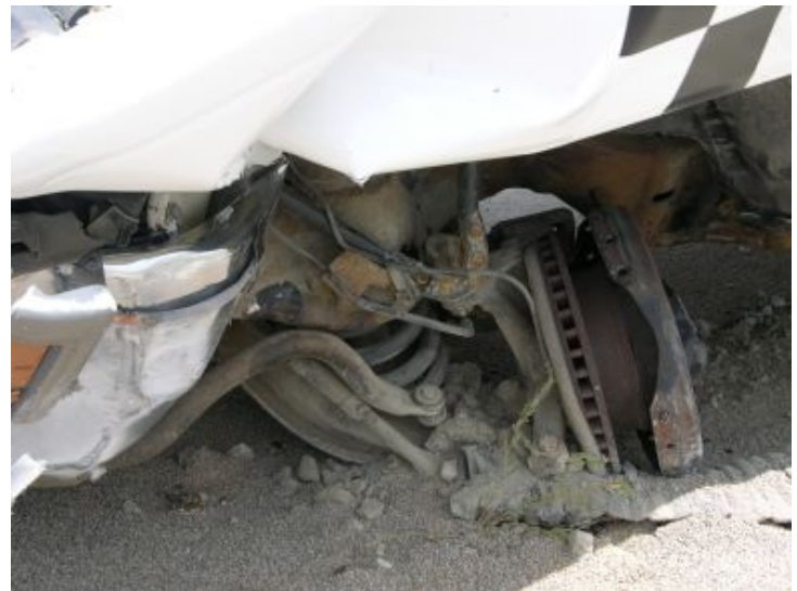
Figure 24. Vehicle Damage, Left-Front Wheel, Test CBPP-1
