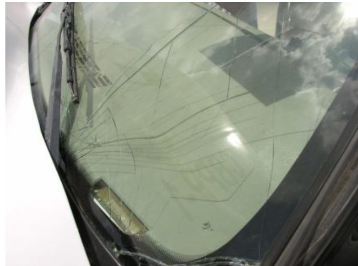
Figure 27. Vehicle Damage, Hood and Windshield, Test CBPP-1
