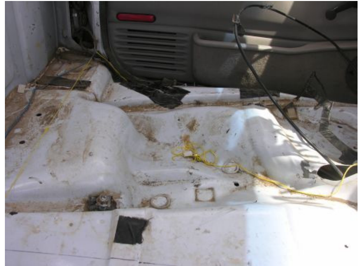
Figure 28. Vehicle Damage, Occupant Compartment, Test CBPP-1
