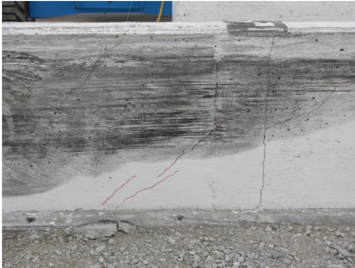
Figure 20. System Damage, Front Side Concrete Cracks, Test CBPP-1
