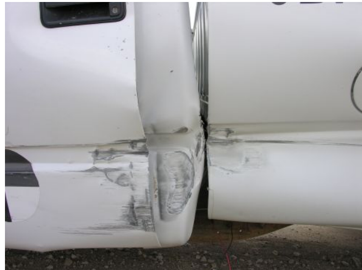
Figure 25. Vehicle Damage, Left Side, Test CBPP-1
