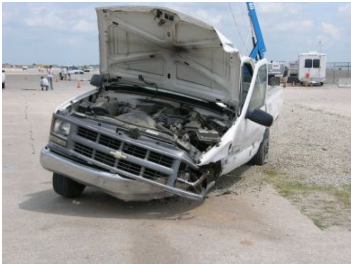
Figure 23. Vehicle Damage, Test CBPP-1
