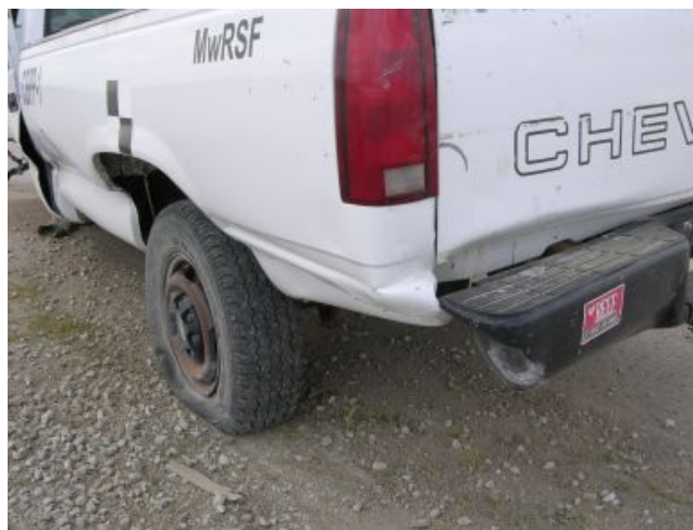
Figure 29. Vehicle Damage, Rear of Vehicle, Test CBPP-1
