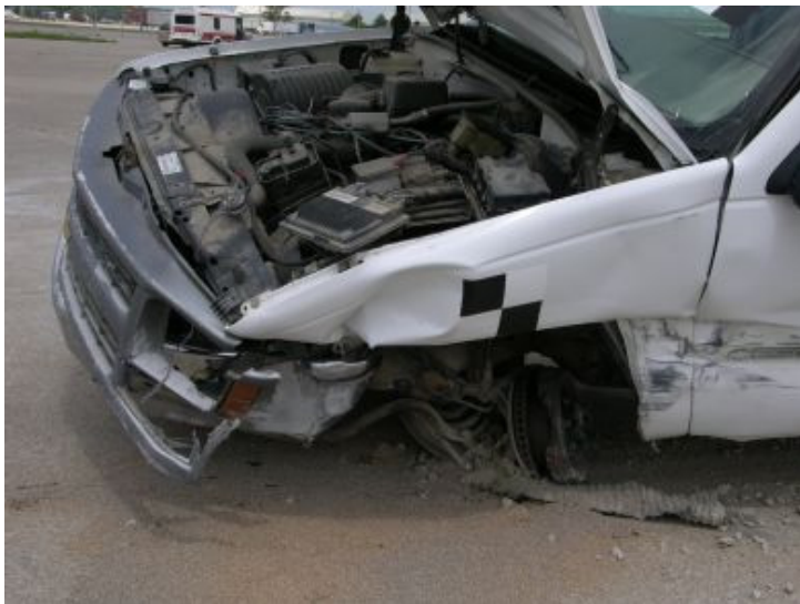
Figure 24. Vehicle Damage, Left-Front Wheel, Test CBPP-1
