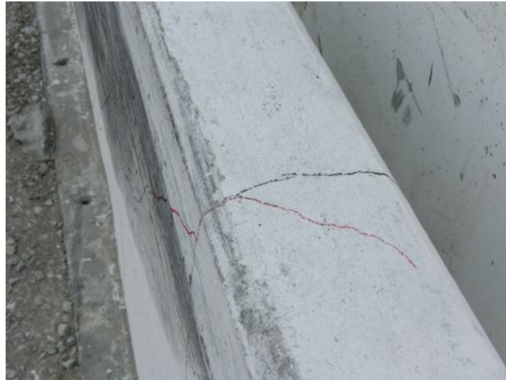
Figure 20. System Damage, Front Side Concrete Cracks, Test CBPP-1
