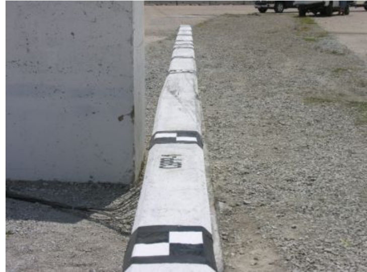
Figure 19. System Damage, Contact Marks and Gouging, Test CBPP-1
