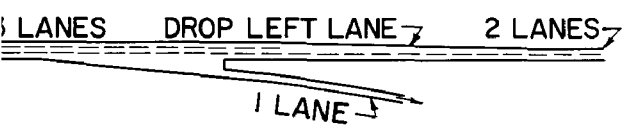
Figure K-5. Lane Drops: Three Lanes to Two, with a One-Lane Exit
