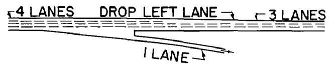
Figure K-6. Lane Drops: Four Lanes to Three, with a One-Lane Exit
