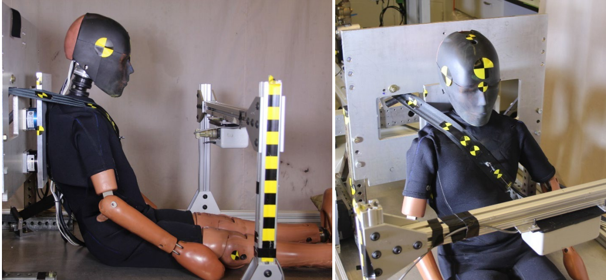
Figure 52. Diagonal belt pull test setup of the LODC Rev5 thorax adapted from Kent et al. (2011)
