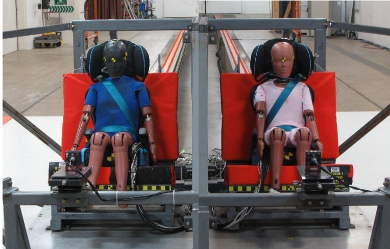
Figure 18. FMVSS No. 213 setup with LODC Rev4 (BioDB #11760) and HIII-10C (BioDB #11757) seated in the highback belt positioning booster (Evenflo Big Kid)
