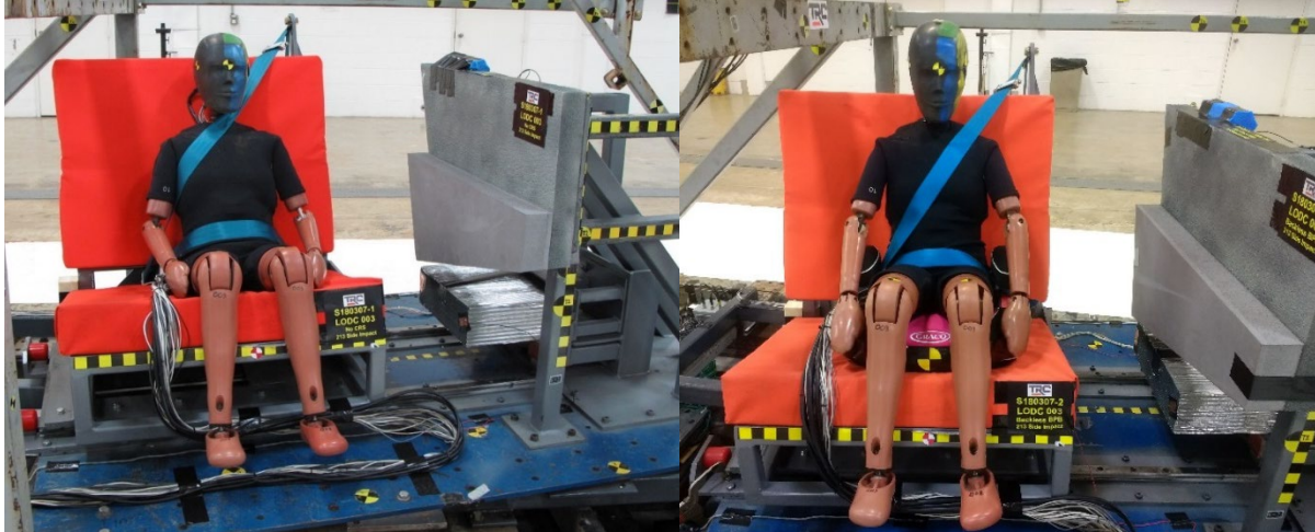
Figure 57. FMVSS No. 213 side impact test setup with no CRS (left) and backless booster (right)
