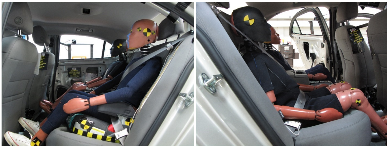
Figure 34. HIII-10C and LODC Rev4 setup in a backless belt positioning booster (left) and with no-CRS (right) in the rear seat of the Chevrolet Malibu vehicle buck
