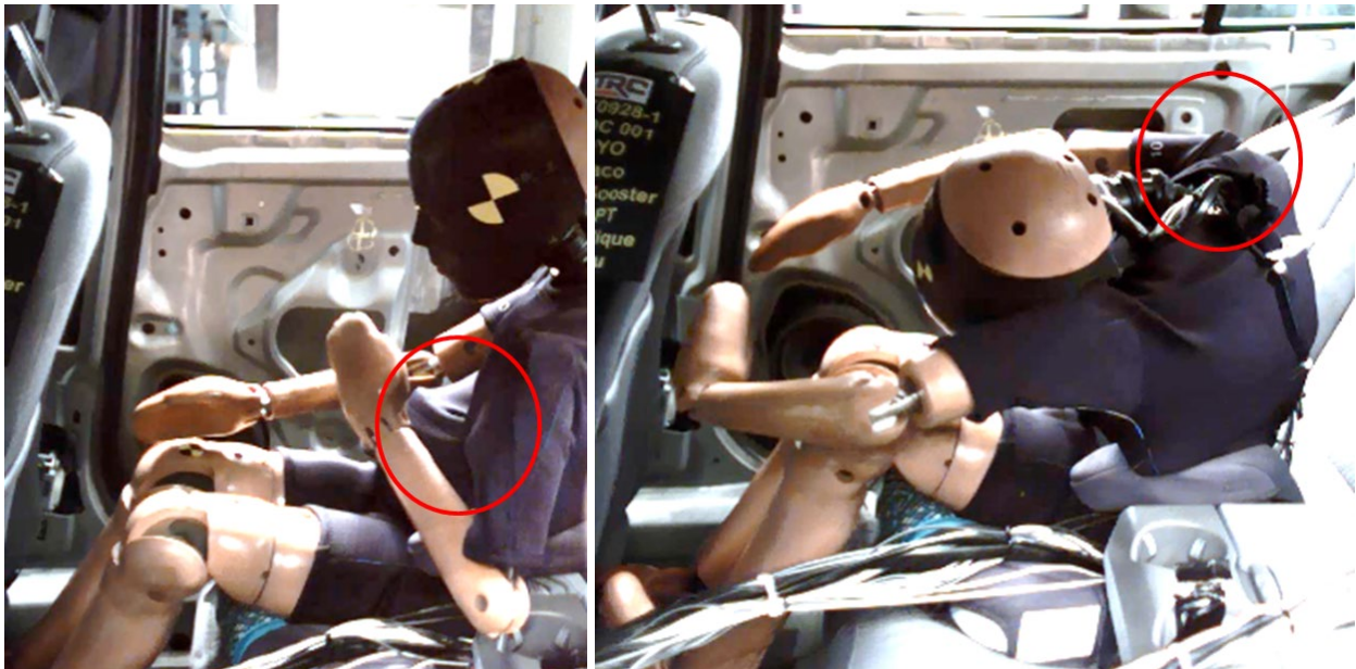
Figure 40. Forward translation of the abdomen (left) and shoulder belt entrapment (right) of the LODC Rev4 in the Malibu vehicle buck sled tests
