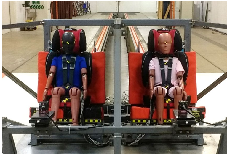
Figure 17. FMVSS No. 213 setup with LODC Rev4 (BioDB #11756) and HIII-10C (BioDB #11755) seated in the five-point harness (Britax Frontier Clicktight)
