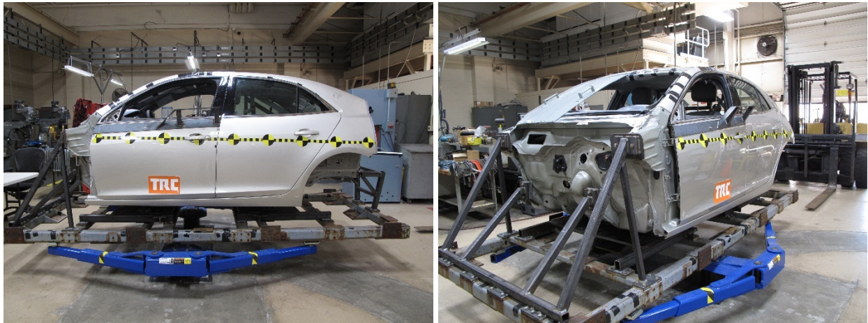
Figure 32. 2016 Chevrolet Malibu sled buck in a frontal configuration
