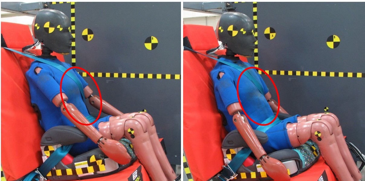
Figure 31. Initial position of LODC 001 (left) that exhibited an unusually high chest acceleration versus an LODC that exhibited a more normal chest acceleration (right)
