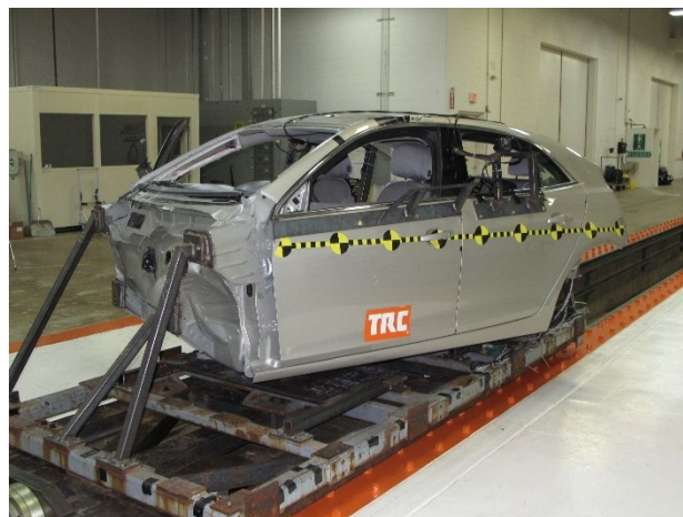
Figure 33. 2016 Chevrolet Malibu sled buck in an oblique configuration
