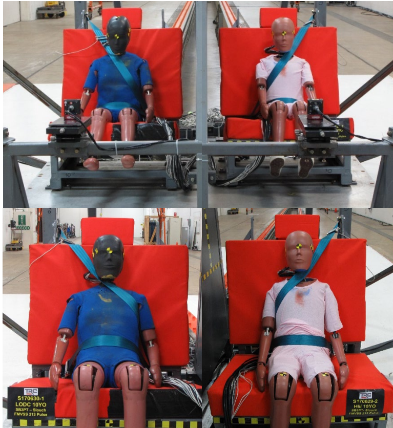
Figure 20. FMVSS No. 213 setup with LODC Rev4 (BioDB #11764/11766) and HIII-10C (BioDB #11761/11763) seated in the no-CRS upright (top) and slouched (bottom) posture configurations, respectively
