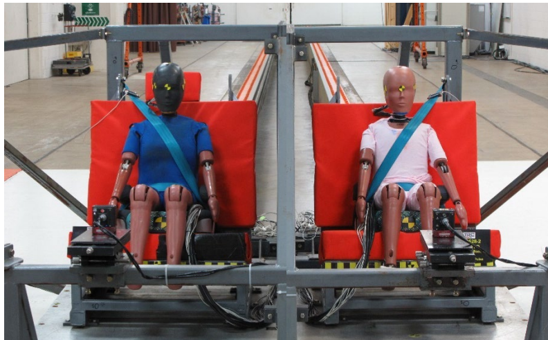
Figure 19. FMVSS No. 213 setup with LODC Rev4 (BioDB #11762) and HIII-10C (BioDB #11759) seated in the backless belt positioning booster (Graco TurboBooster)
