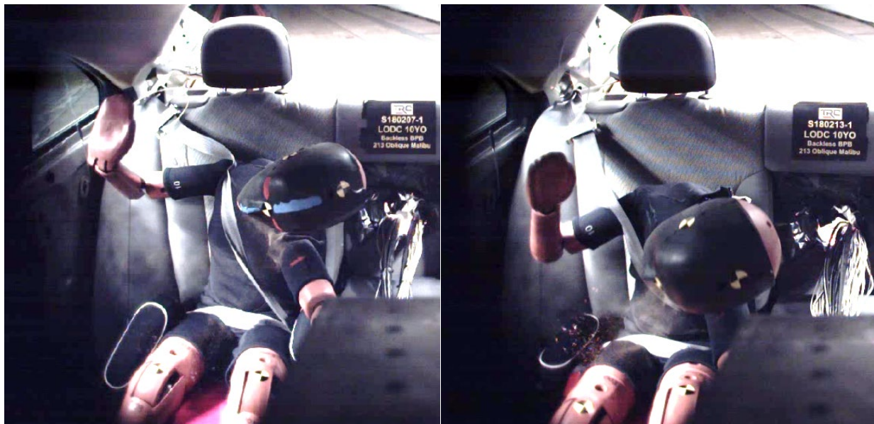
Figure 48. Vehicle buck sled tests showing the previous LODC with shoulder belt entrapment (left) and the modified LODC without shoulder belt entrapment (right)
