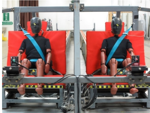
Figure 30. FMVSS No. 213 setup with two LODC Rev4 builds to evaluate reproducibility
